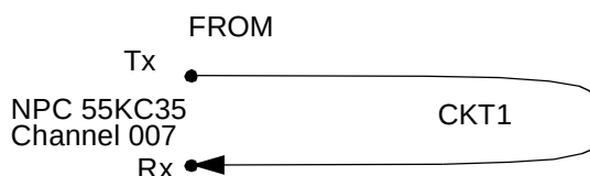
Figure 9-6. Sample Half-Duplex Loopback Circuit
