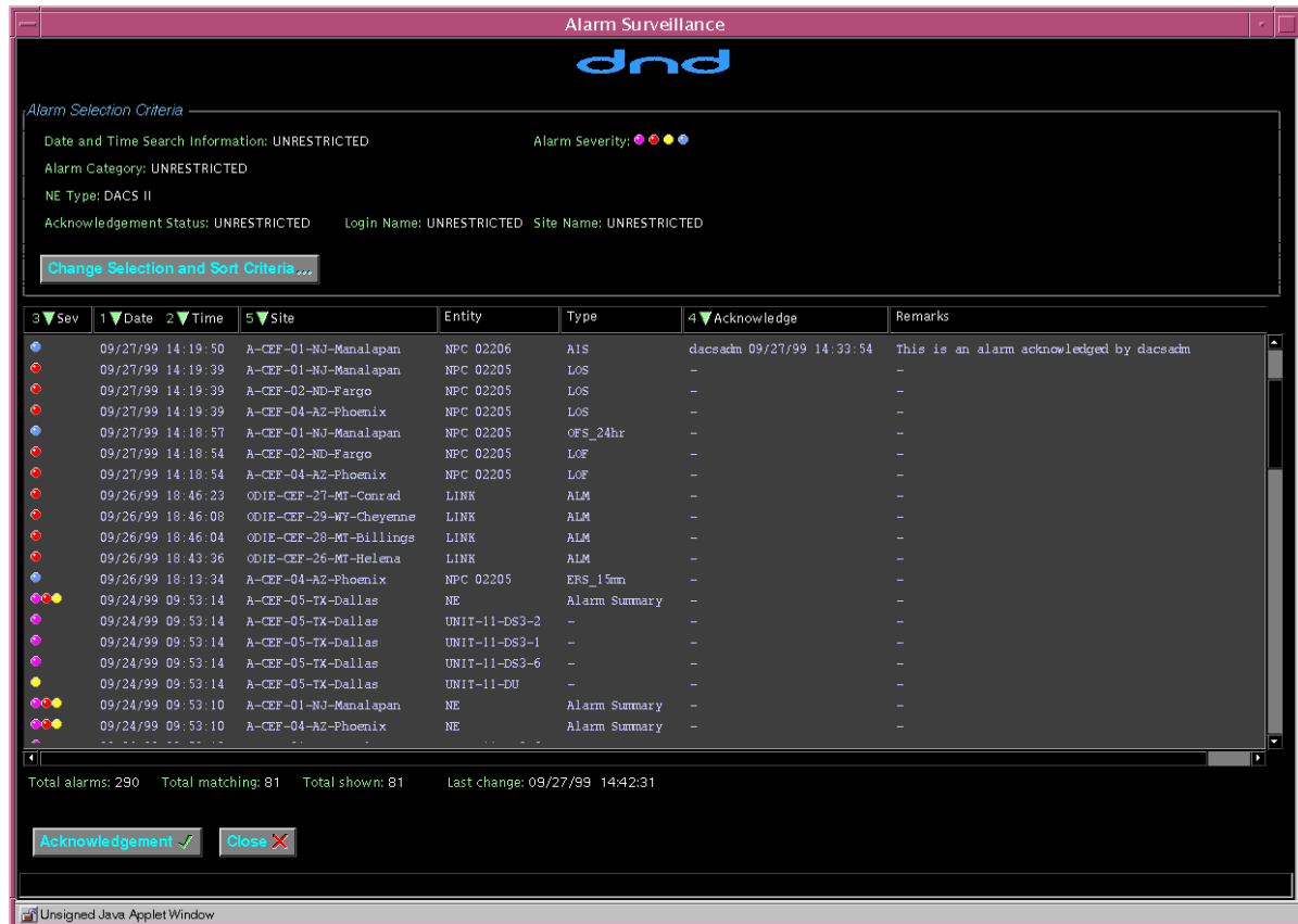
Figure 25-1. ALARM SURVEILLANCE Display - DACS II Related Alarms
