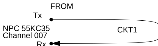
Figure 10-6. Sample Half-Duplex Loopback Circuit
