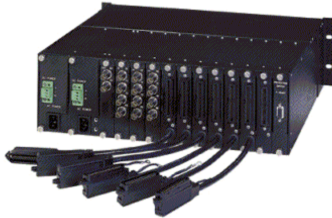
Figure 2-15. N+1 Protection Switch (rear view)
