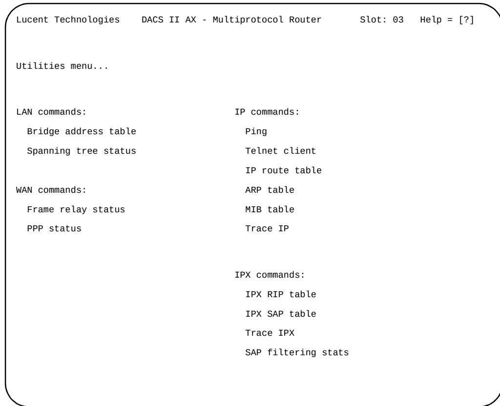
Figure 20-59. Router Utilities Menu
