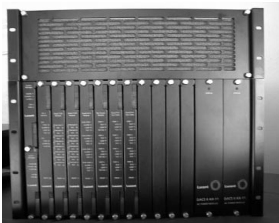
Figure 10-1. N+1 Protection Switch and DACS II AX-11
