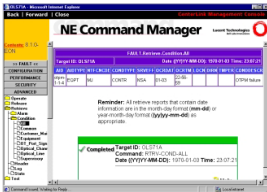
Figure 3-1 Active Alarms and Status Report
