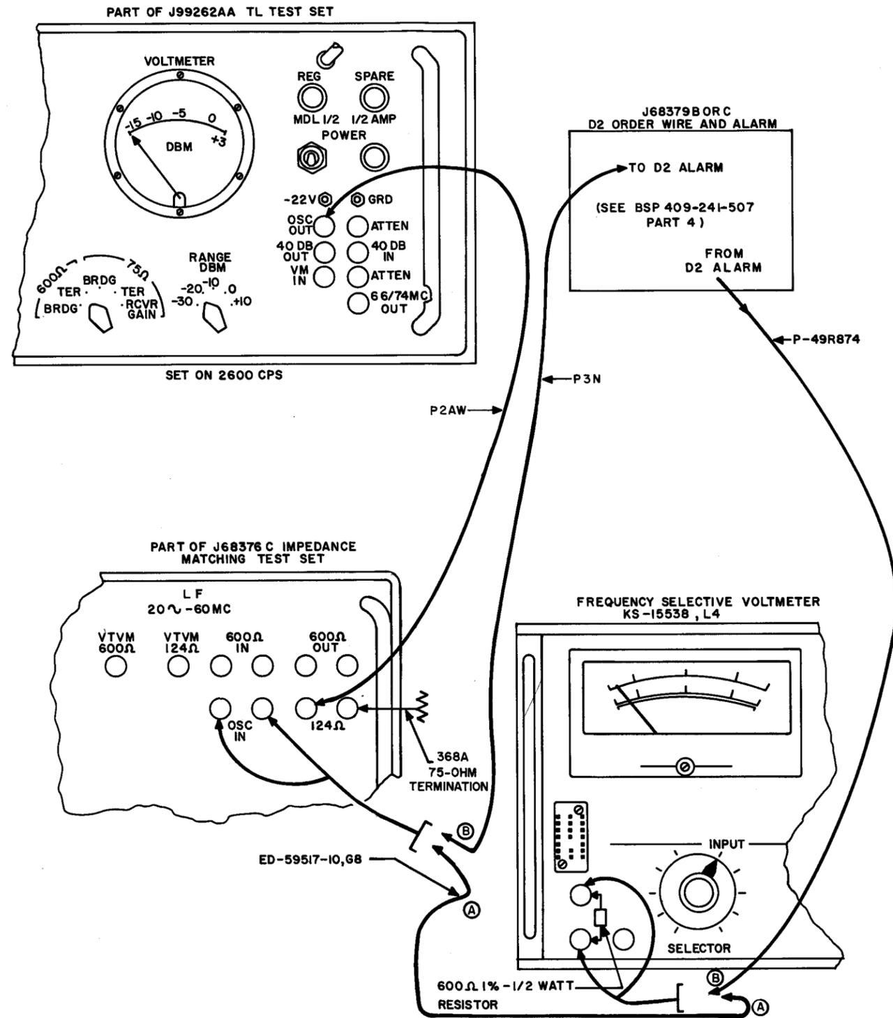
Fig. 6 - Test Connections for Setting 2600 CPS Signaling Tone Levels
