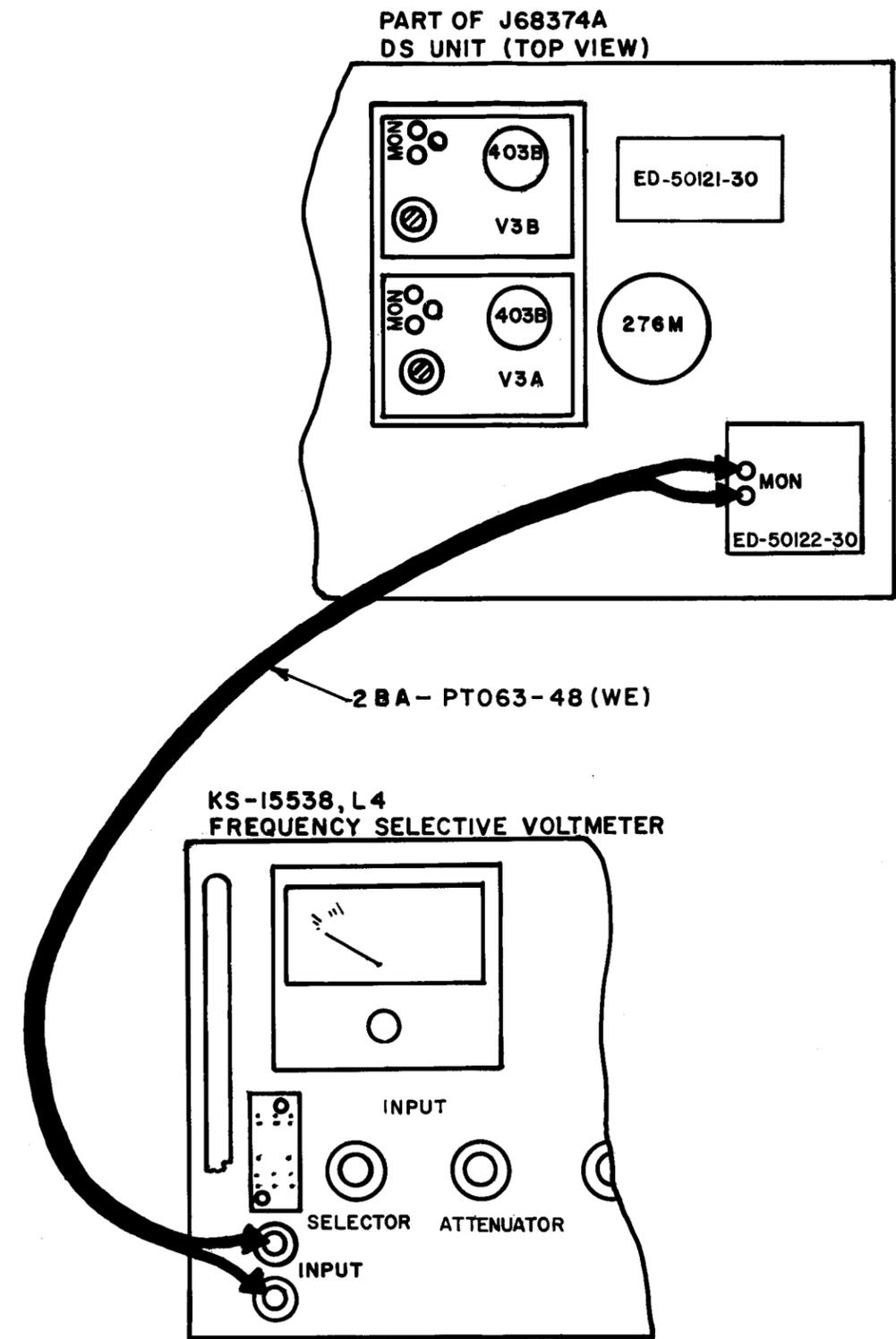
Fig. 3 - Test Connections for 3700-Cycle Pilot Tone Measurements
