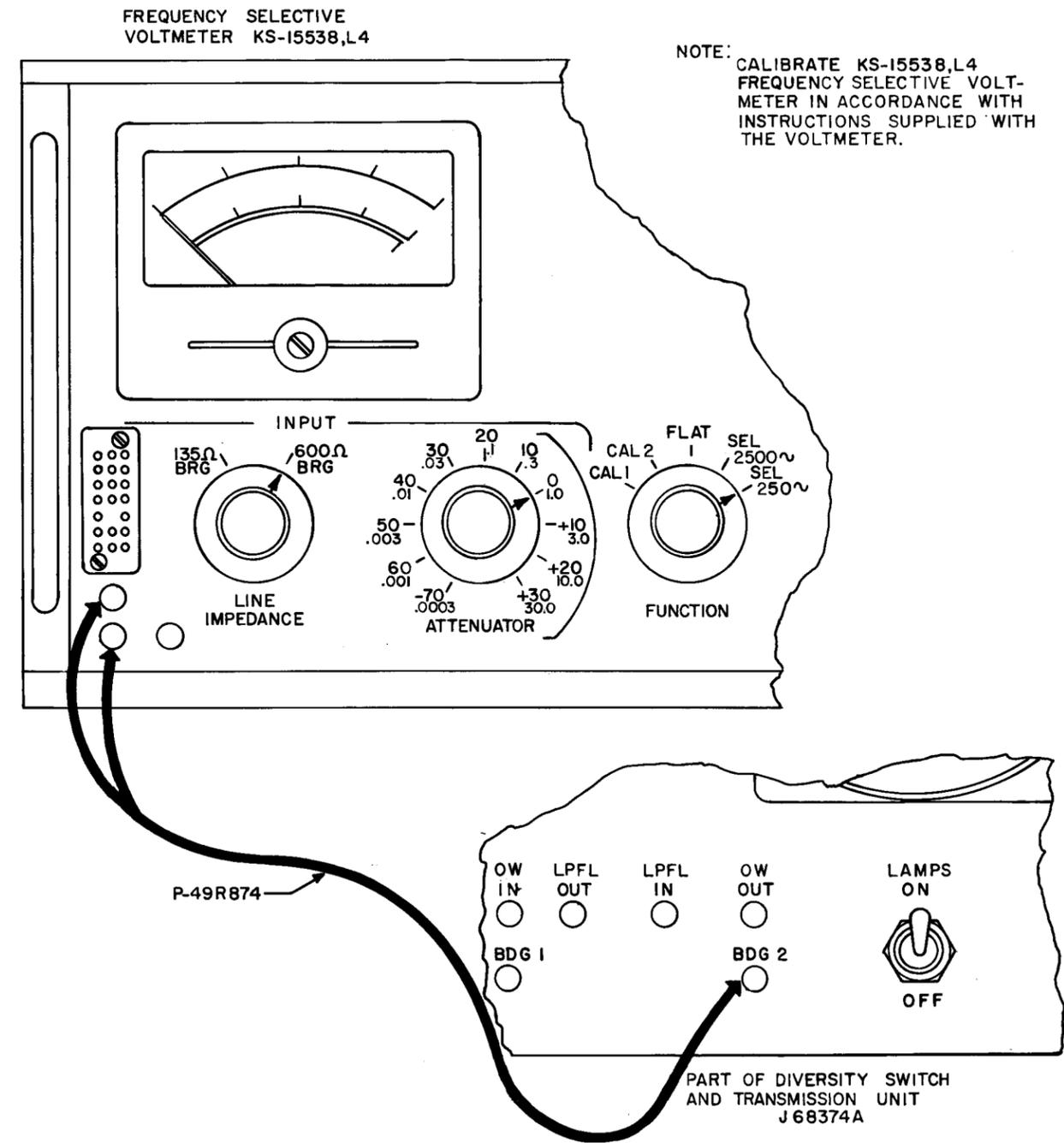
Fig. 1 - Test Connection for Signaling Tone Measurements
