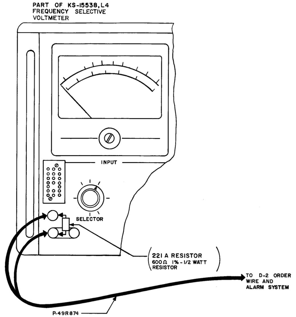
Fig. 5 - Test Connections for Measurement of
