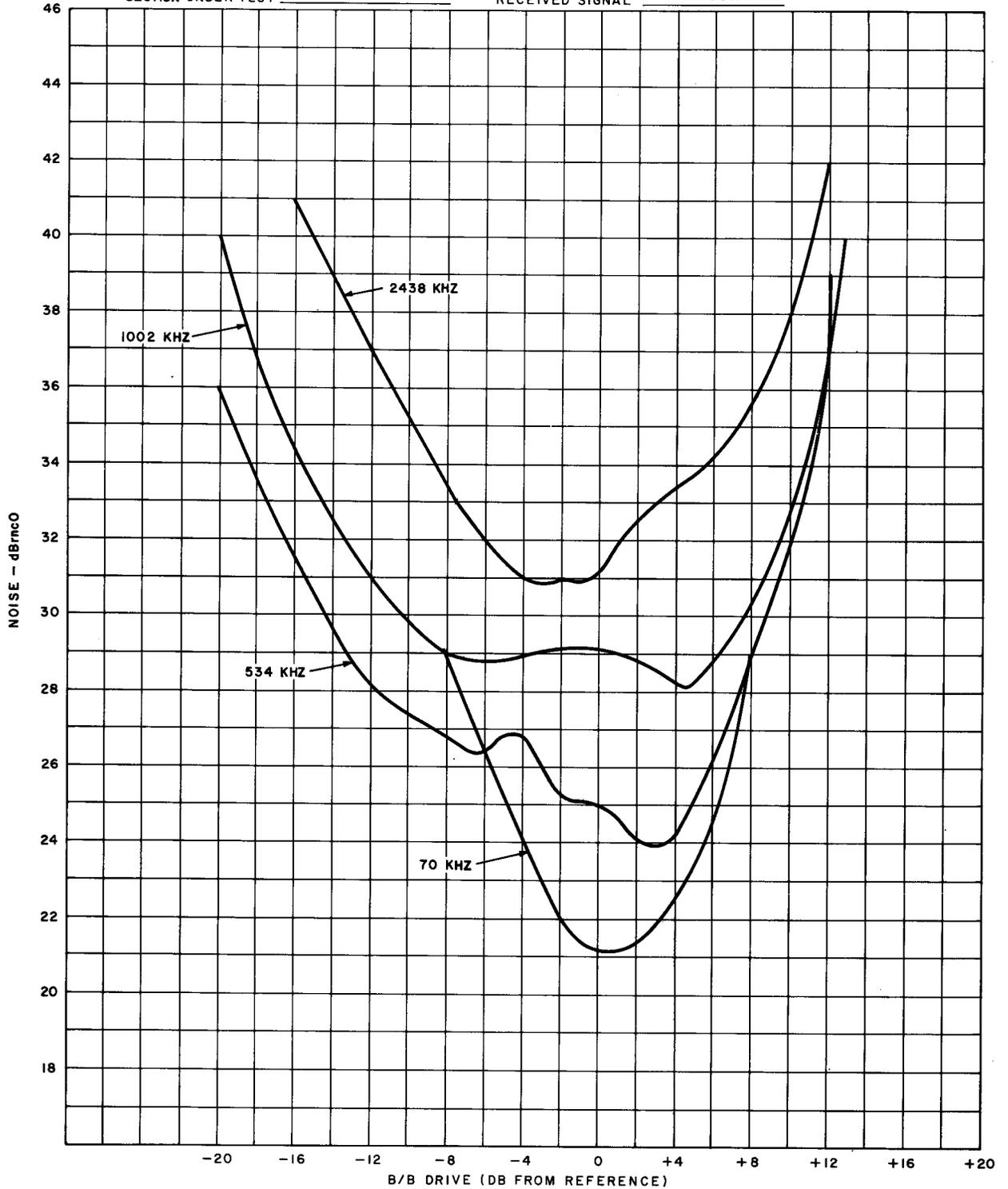
Fig. 6—TM-1 Noise Loading Plot—Unsatisfactory
