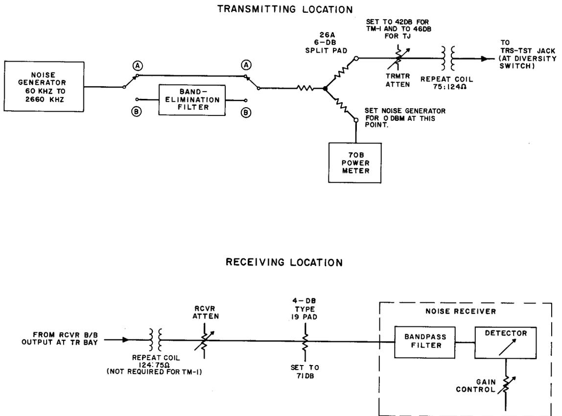
**Fig. 1—TJ/TM-1 Noise Loading—Test Connections**
