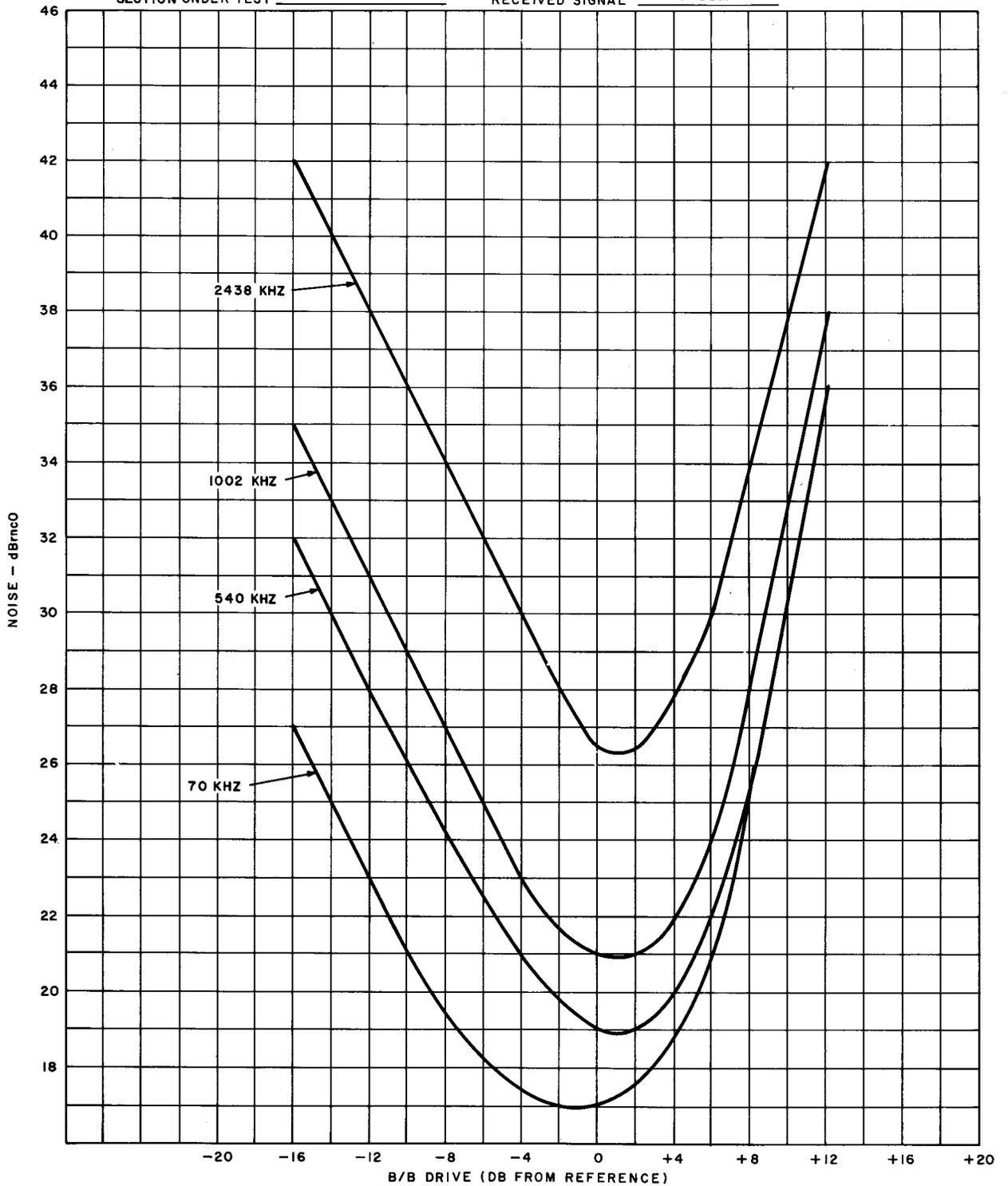
Fig. 4—Typical Satisfactory Noise Loading Plot
