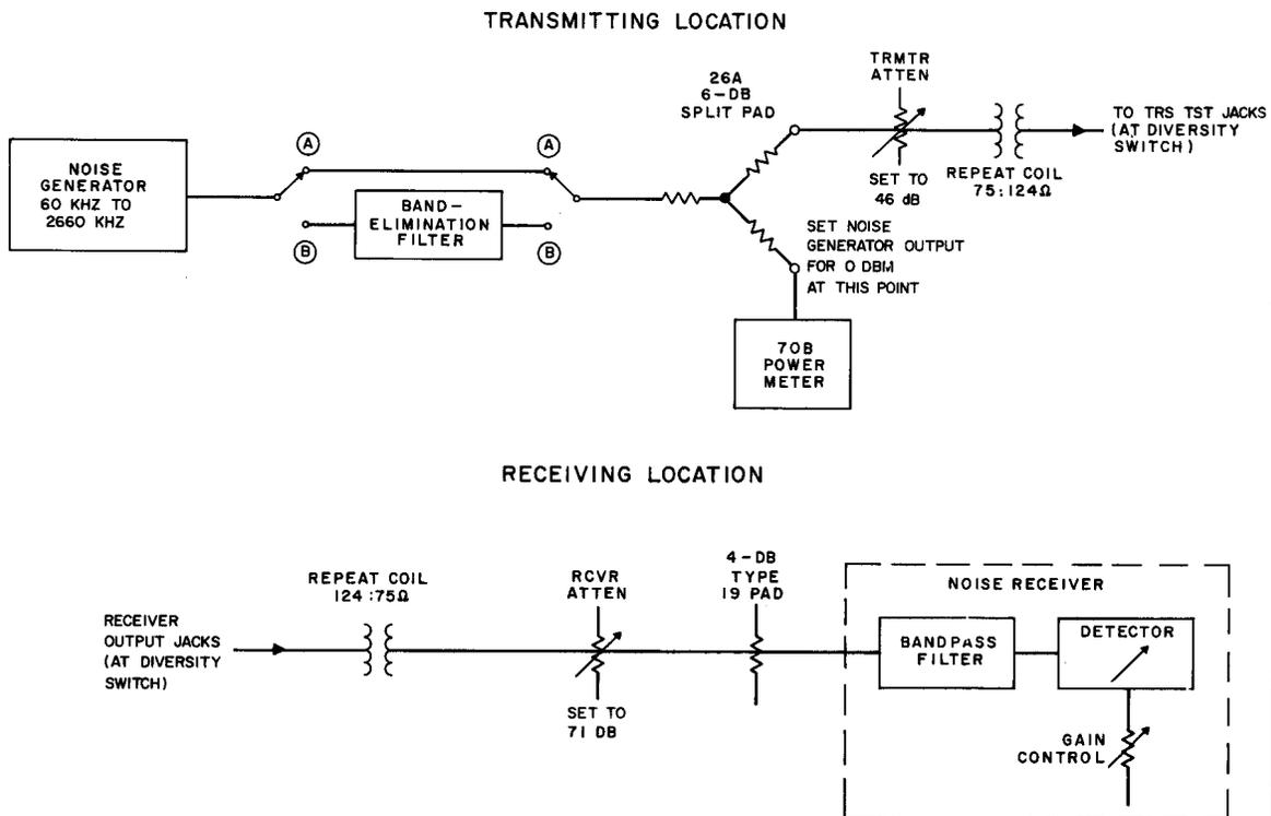
Fig. 1—◆TJ Noise Loading—Test Connections◆
