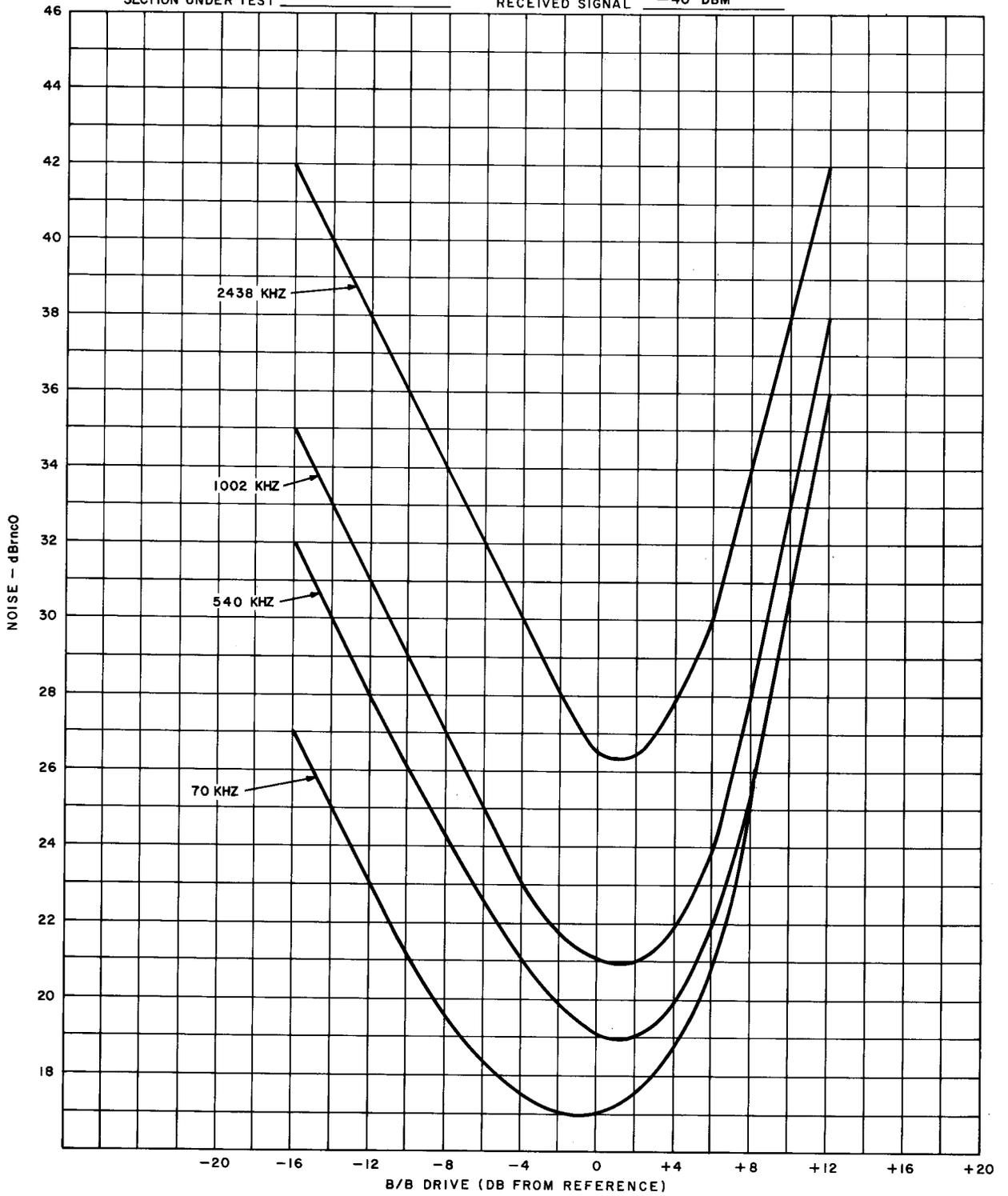
Fig. 4—Typical Satisfactory Noise Loading Plot
