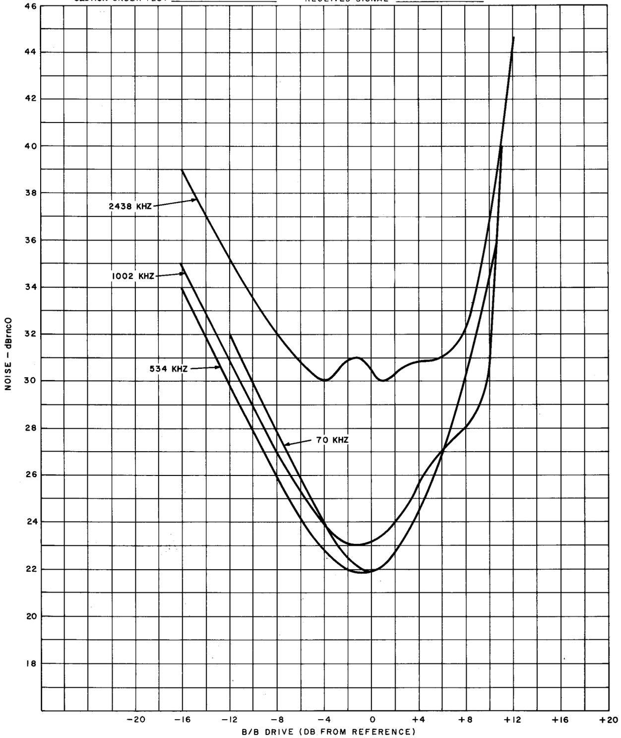
Fig. 5—Noise Loading Plot—Unsatisfactory
