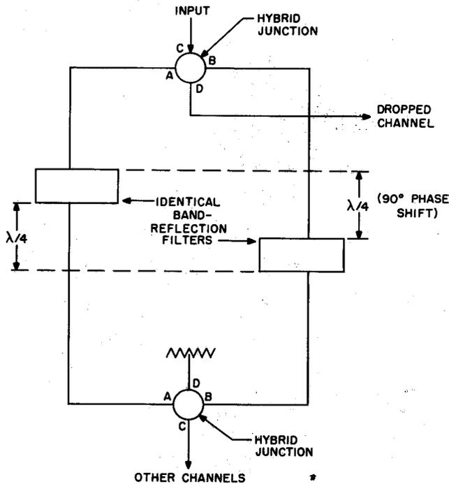
**Fig. 22—Channel Dropping Network—Block Diagram**
