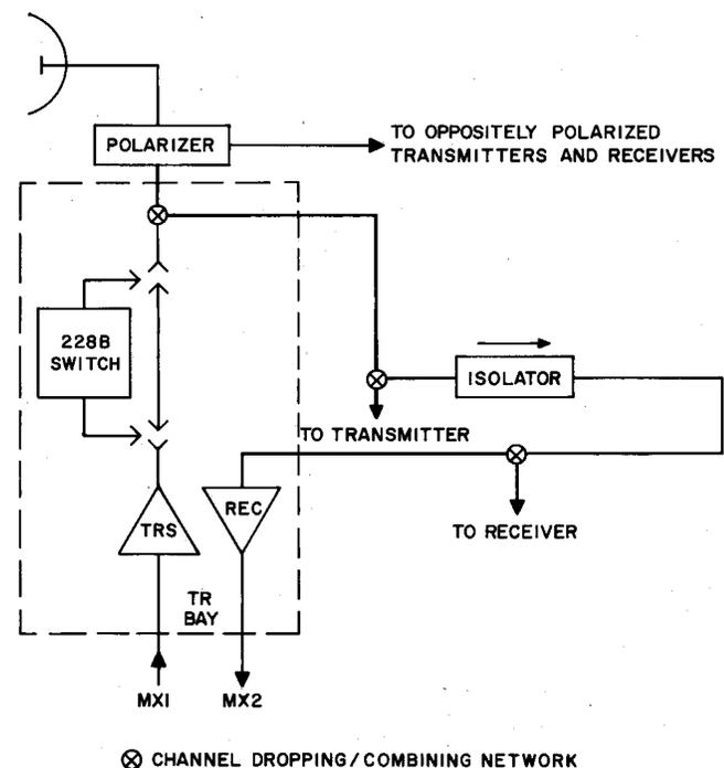
Fig. 20—Typical Terminal-Type Transmitter-Receiver Bay Arrangement—Block Diagram
