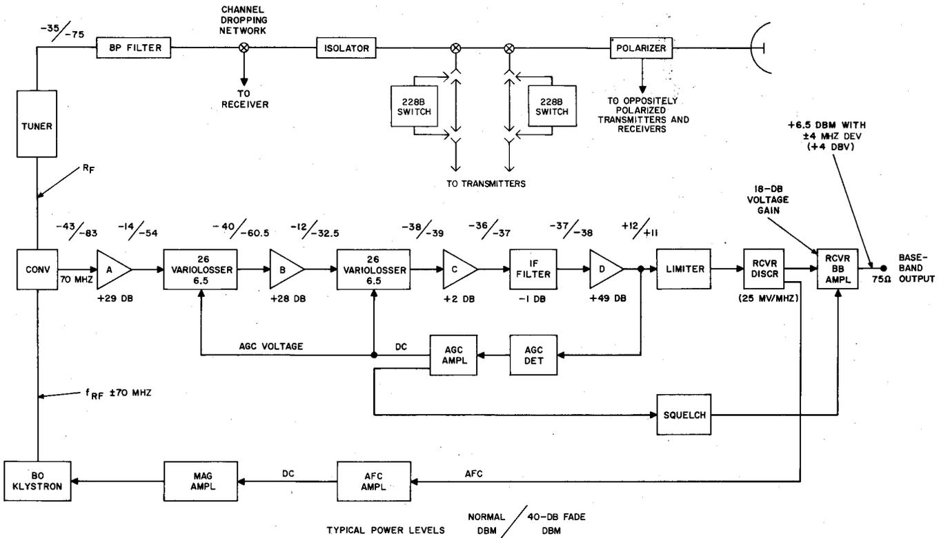
Fig. 3—J99262G Receiver—Block Diagram
