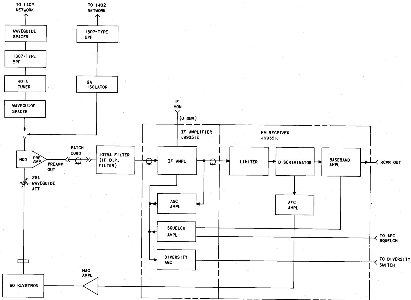
Fig. 9—Receiver Equipped With J99351E IF Amplifier Unit, J99351J FM Receiver, and 1075A Filter—Block Diagram
