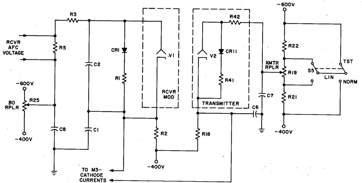
Fig. 18—Klystron Repeller Voltage Circuit—Schematic Diagram
