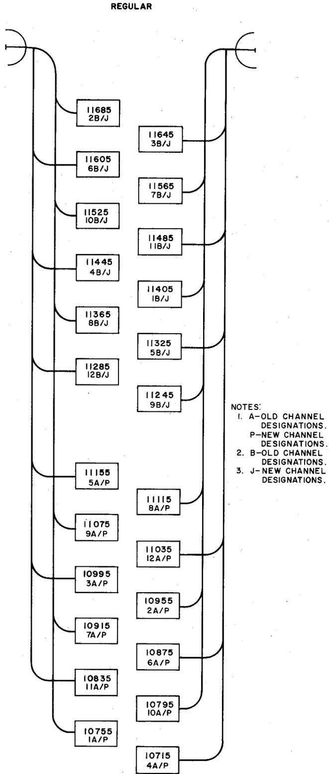
**Fig. 12—The 11-GHz Frequency Plan—Block Diagram**
