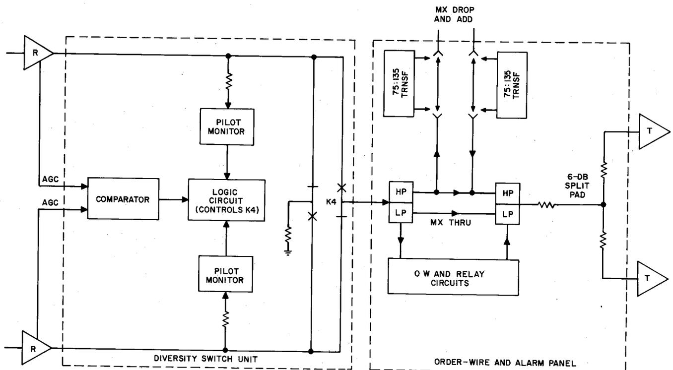
Fig. 11—Transmitter-Receiver Auxiliary Circuits—Block Diagram
