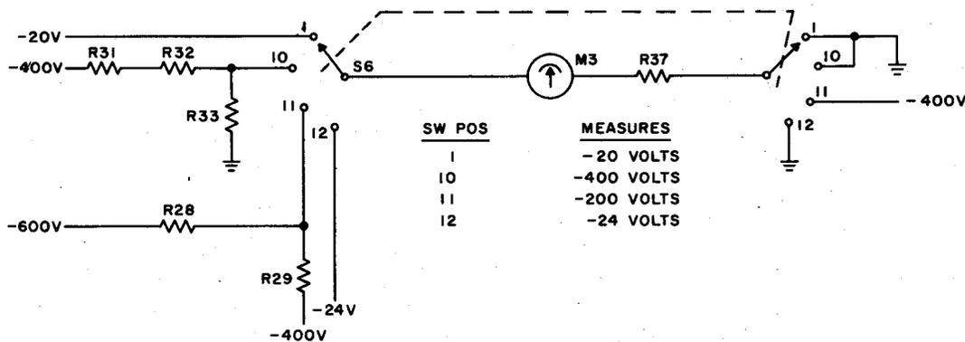
Fig. 16—M3 Metering Circuit—Simplified Schematic Diagram
