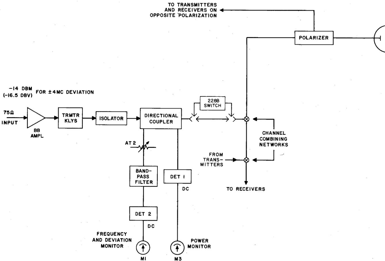
Fig. 10—Transmitter—Block Diagram
