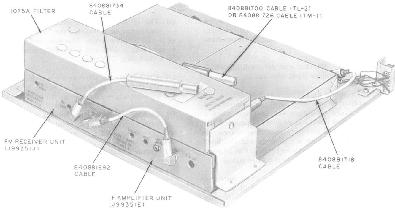
**Fig. 8—IF Amplifier and FM Receiver Arrangement Consisting of 1075A Filter, J99351E IF Amplifier Unit, J99351J FM Receiver, and Associated Cables**
