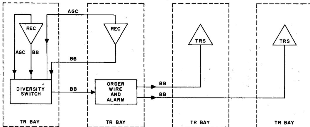
Fig. 21—Automatic Gain Control and Baseband Signal Paths—Block Diagram
