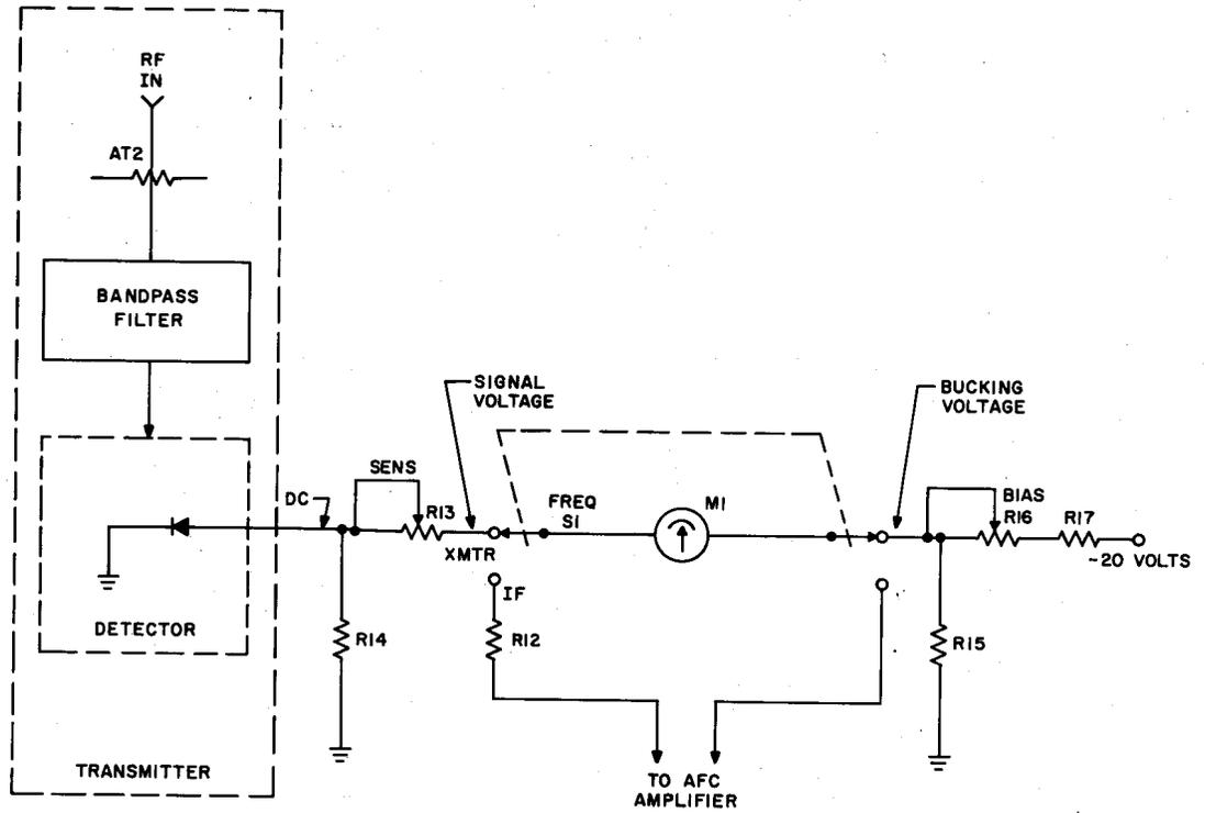
Fig. 17—M1 Metering Circuit—Simplified Schematic Diagram
