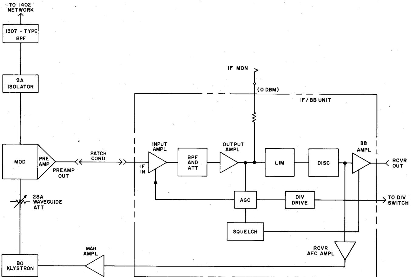
Fig. 7—Receiver Equipped With J99296G IF and Baseband Unit—Block Diagram
