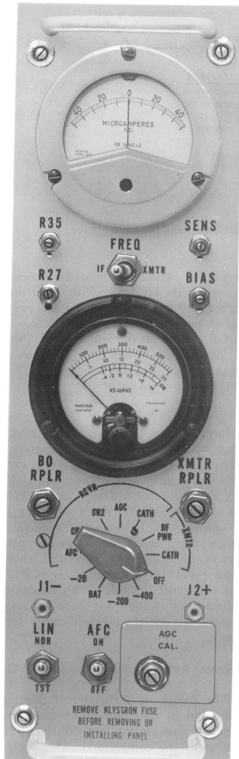
Fig. 15—J99262K Meter and Control Panel Equipped With Printed Wiring Board Assembly (ED-3C535-30)
