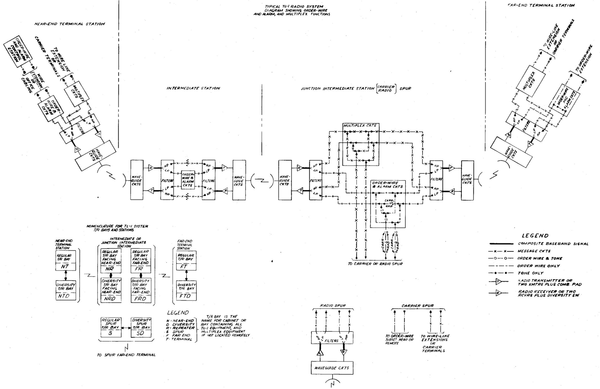
Fig. 25—Typical TL-1 Radio System—Functional Block Diagram
