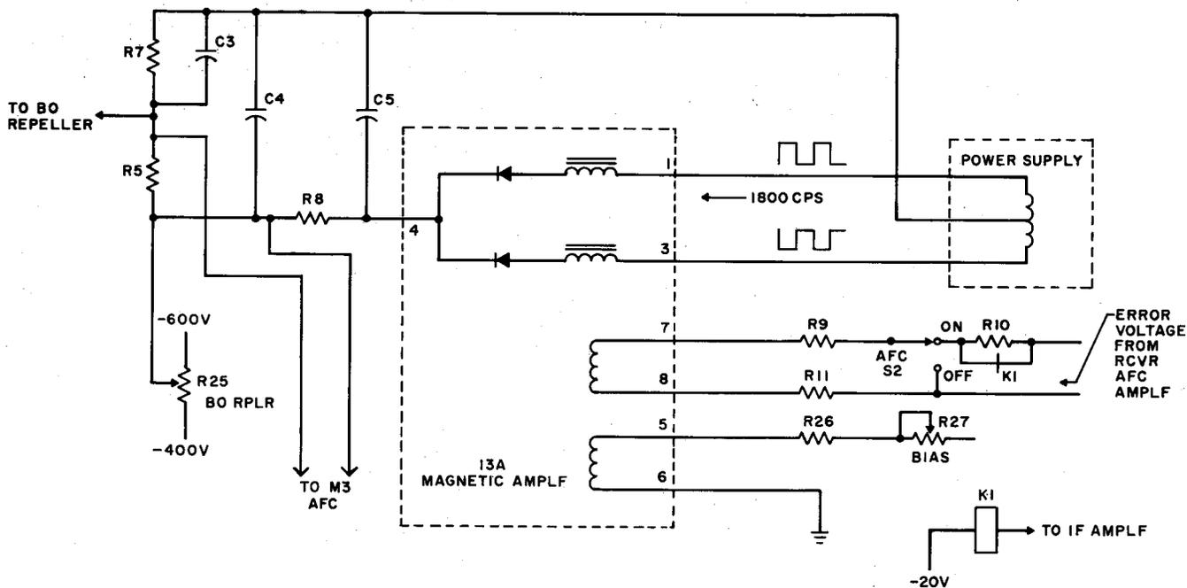
Fig. 19—Receiver Automatic Frequency Control Circuit—Schematic Diagram
