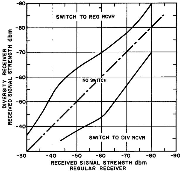
Fig. 2 – Typical Comparator Switching Characteristic
