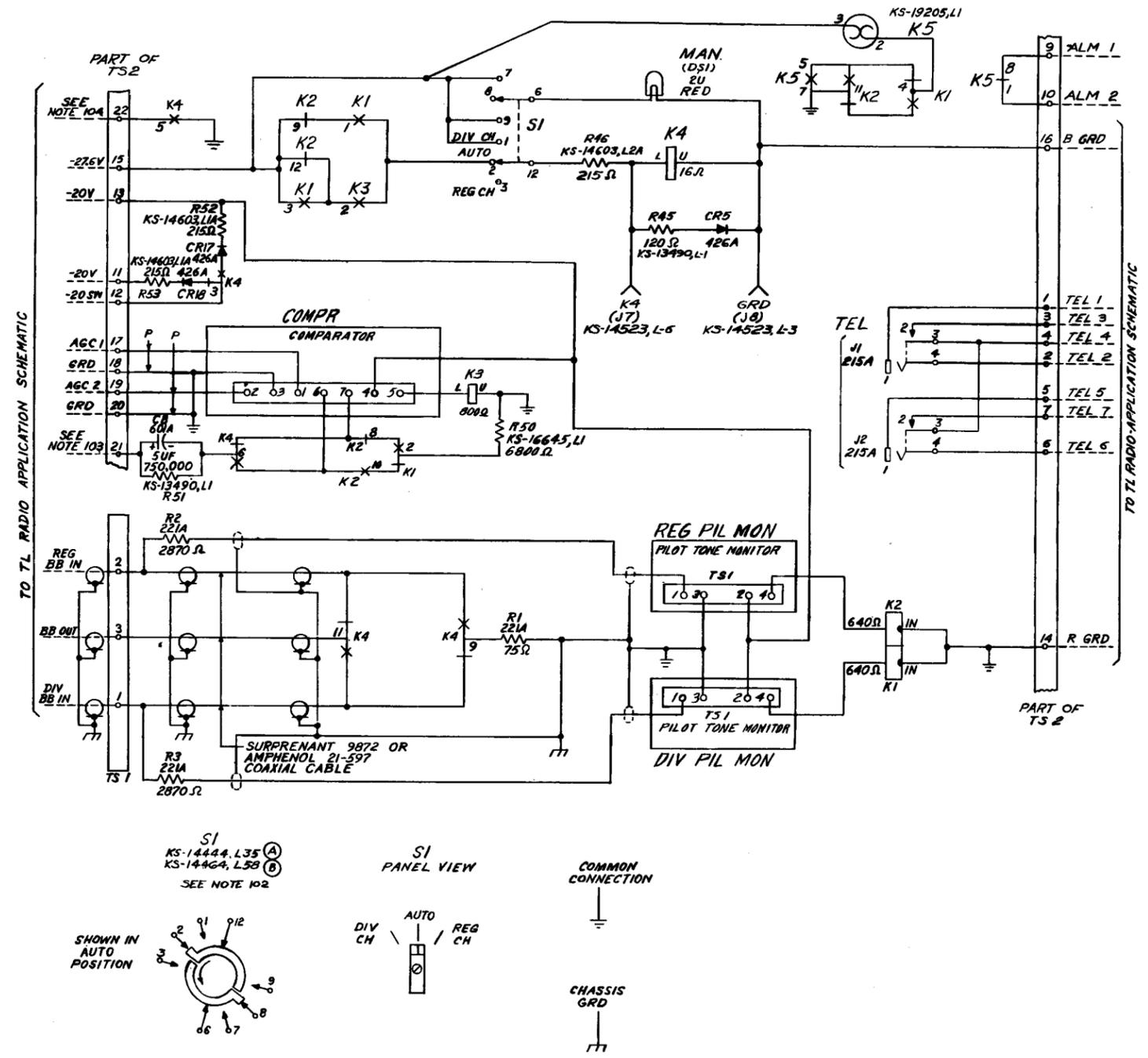
Fig. 4 - Typical Diversity Switch Circuit
