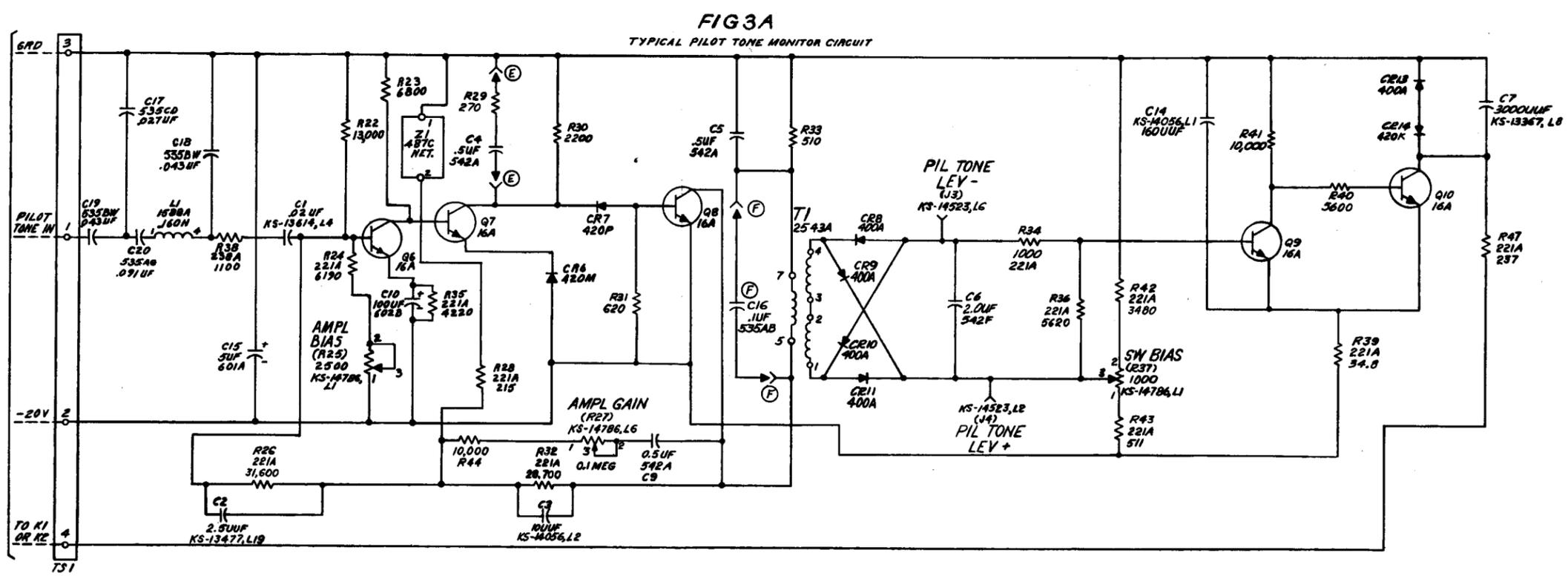
Fig. 3 - Typical Comparator and Pilot Tone Monitor Circuits
