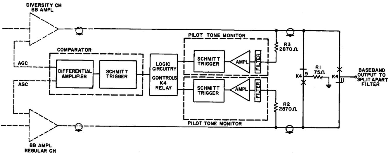
Fig. 1 - TL Radio Diversity Switch Block Diagram
