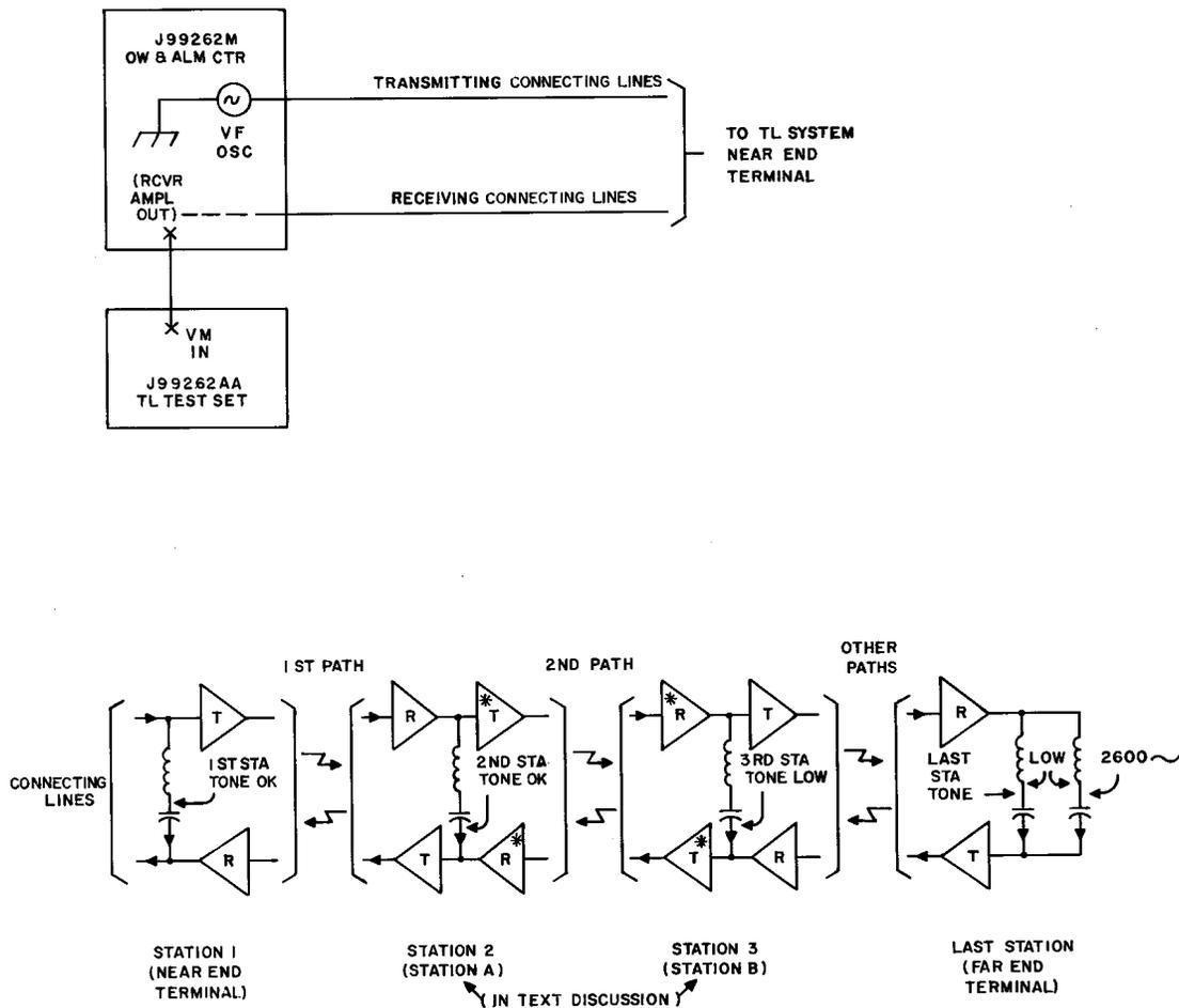
Fig. 1 - Block Schematic of TL Order Wire Route
