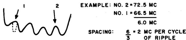
Fig. 4—Delay Pattern with Ripples
