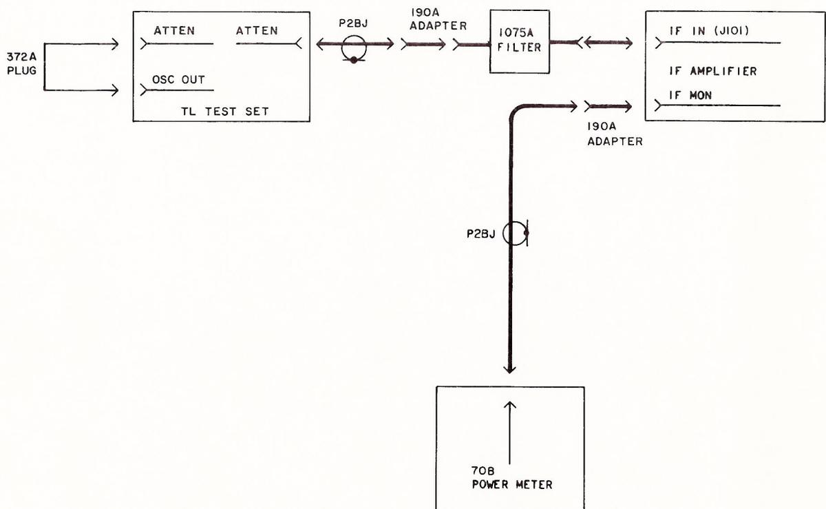
Fig. 2—J99351E IF Amplifier Unit—AGC Performance Test—Test Setup Diagram
