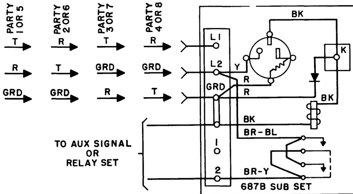
Fig. 6 - Auxiliary Signals on Party Lines
