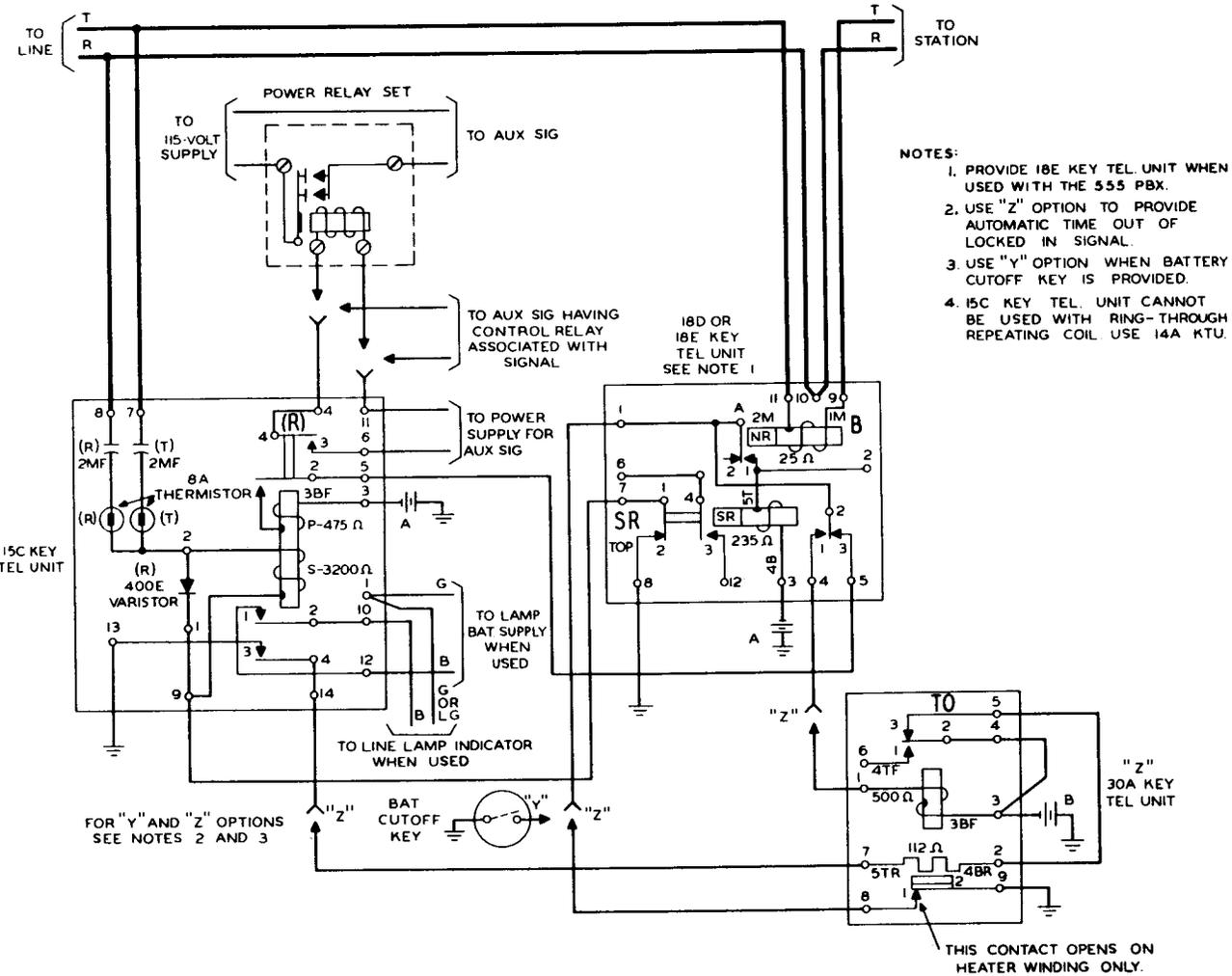
Fig. 8 - Connections and Circuit Operation for Continuous Auxiliary Signals
