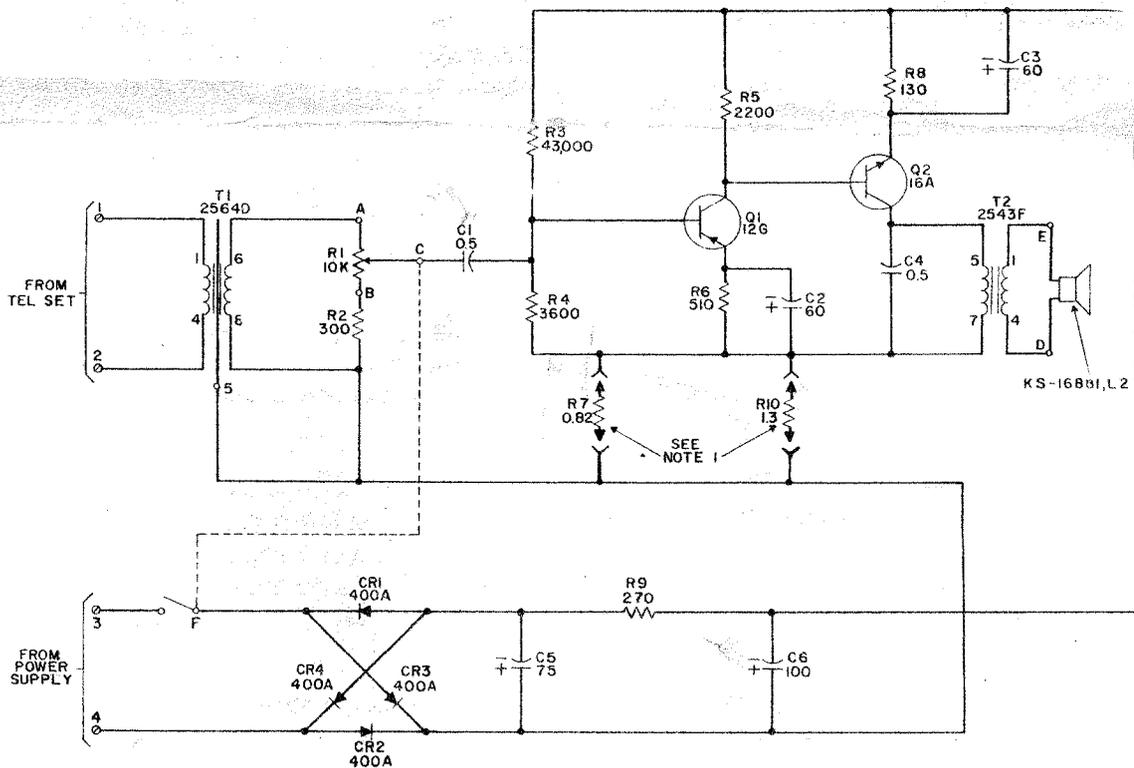
Note 1: Resistor R7 or R10 may have been removed at the factory to adjust gain. (This is a factory option).
