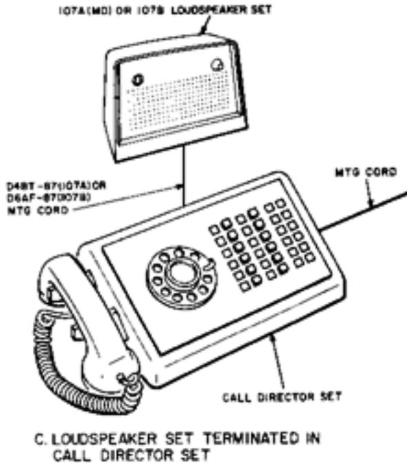
Fig. 4—107-Type Loudspeaker Set, Typical Installation Layouts
