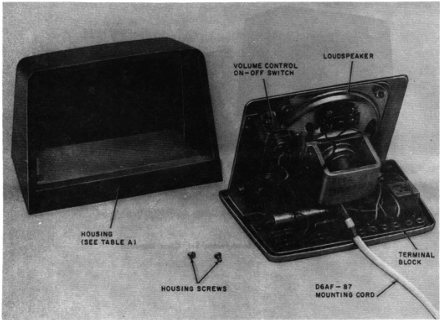
Fig. 3— $\Phi$ 107B Loudspeaker Set, Cover Removed $\Phi$
