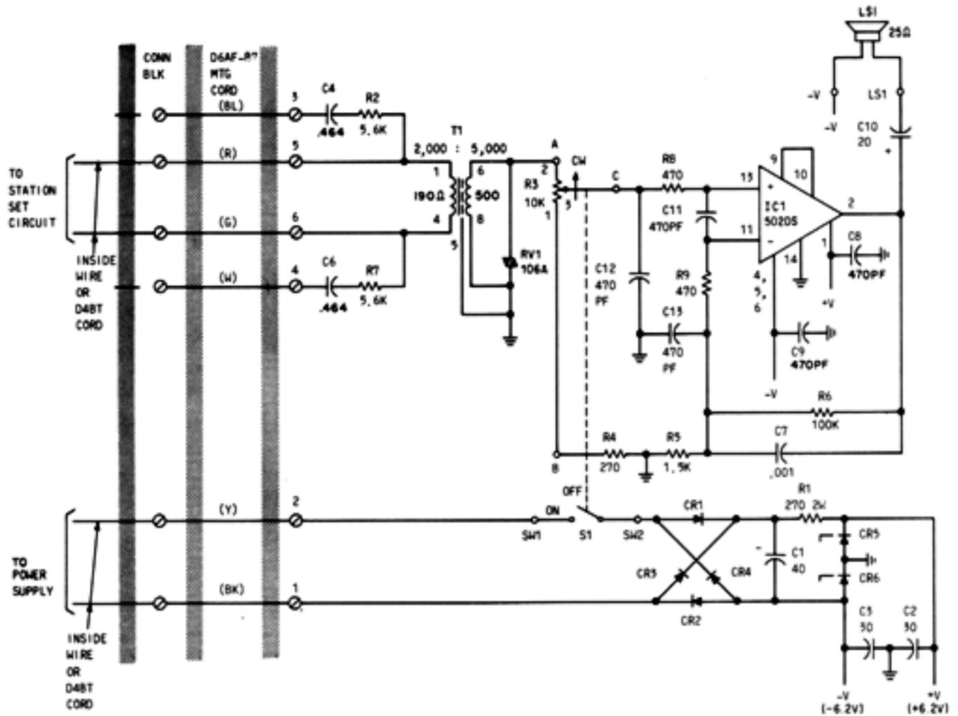
Fig. 10—107B Loudspeaker Set, Schematic and Typical Connections
