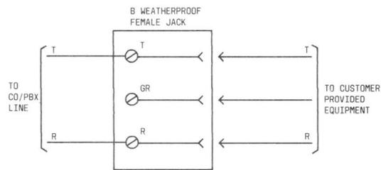
Fig. 4—Connections for USOC RJ15C—Bridged Tip and Ring
