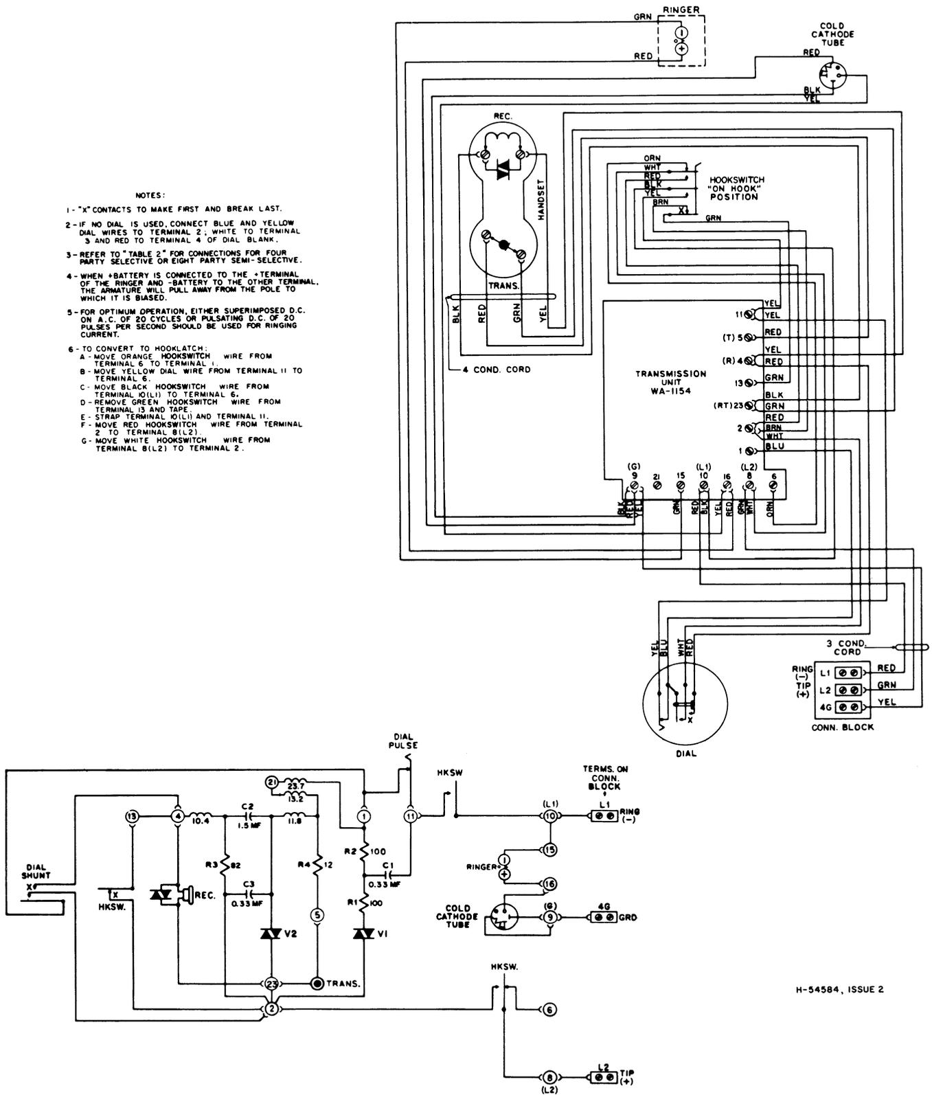
Figure 2. Schematic and Wiring Diagram, Type 80 Self-Compensating Telephone Set NC-802 with Superimposed Ringing.
