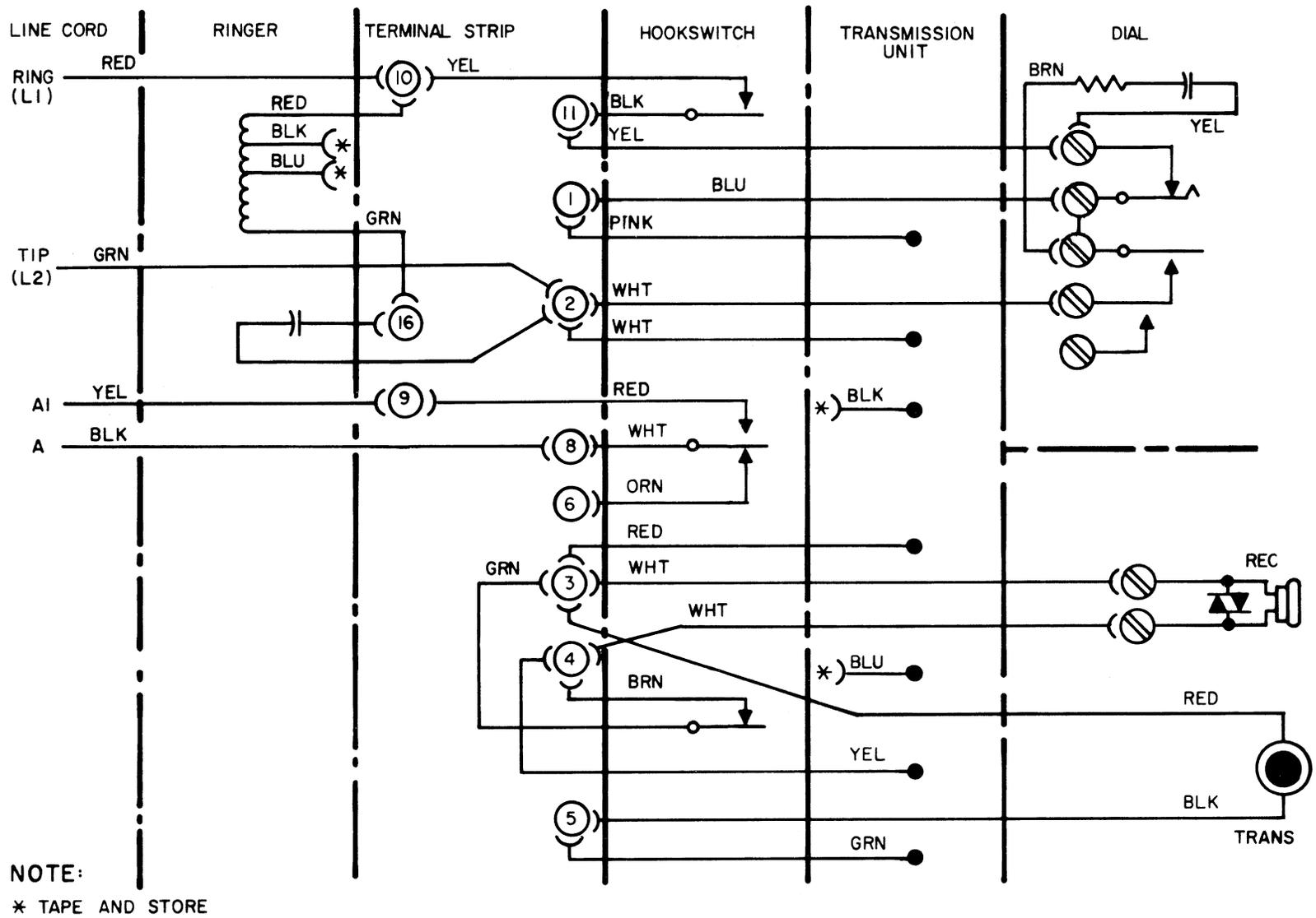
Figure 5. Wiring Diagram of Decorator Conversion Kit Wired for Use in Key Telephone System.
