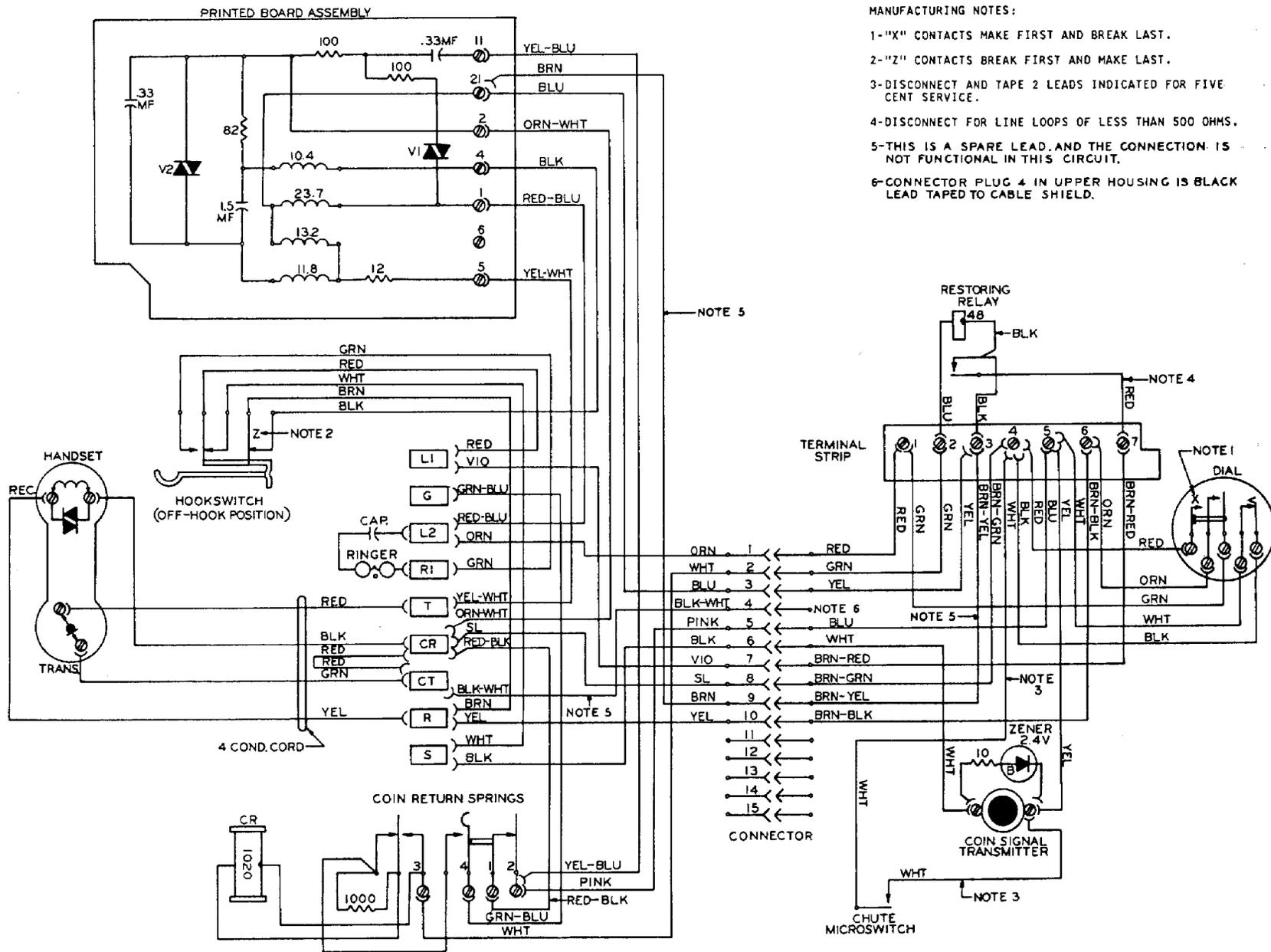
Figure 2. Wiring Diagram, LPC82-55 Coin Telephone Set.
