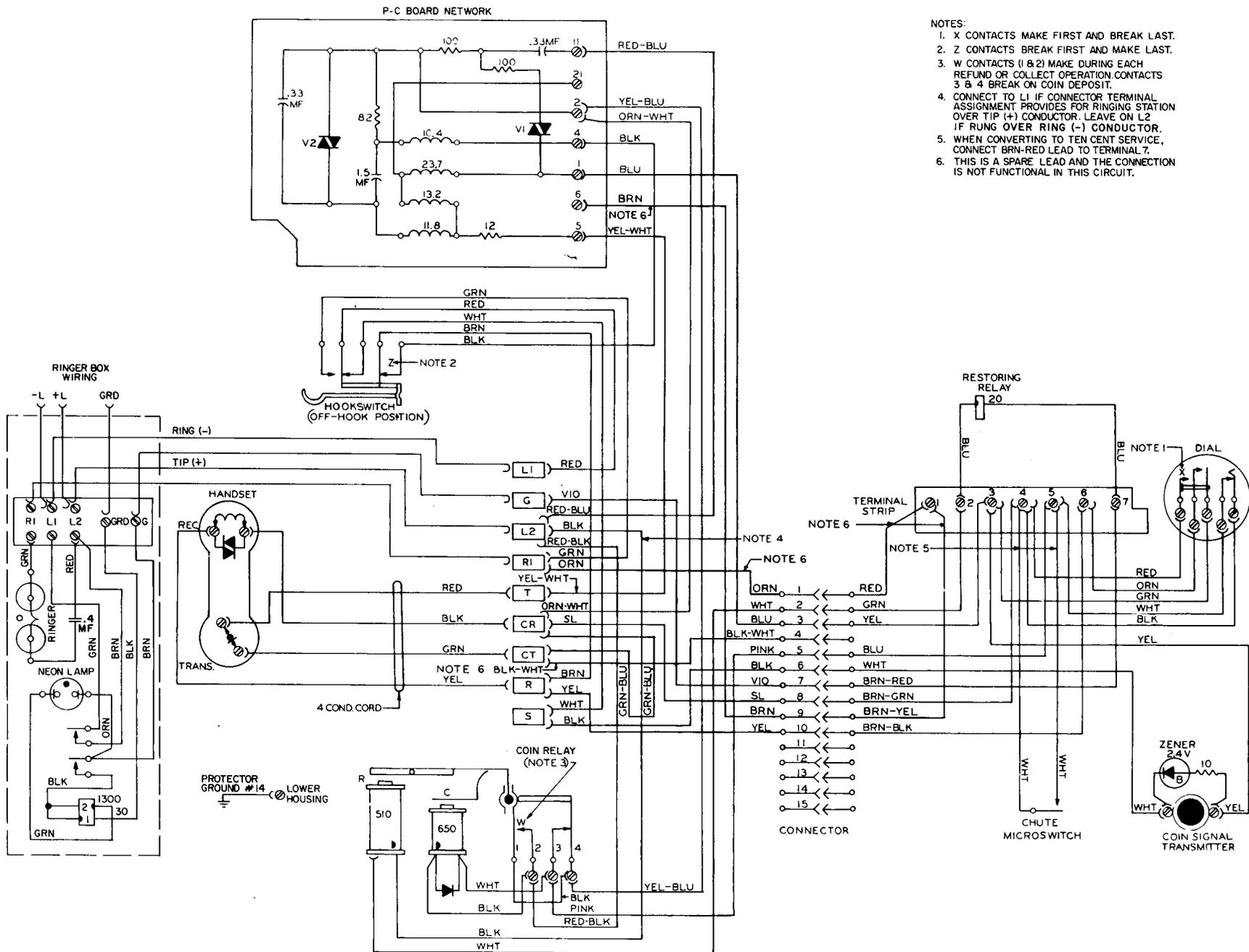
Figure 2. Wiring Diagram, LPC89-55 Coin Telephone Set.
