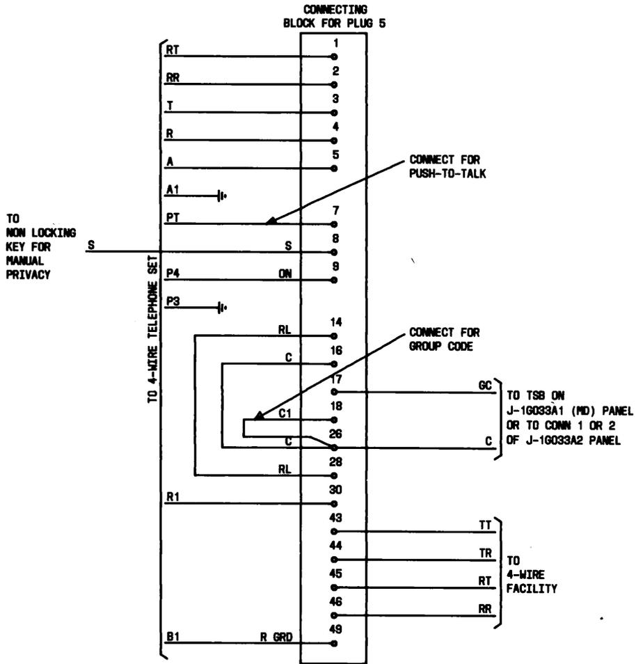
Fig. 11—Connections for One 4-Wire Telephone Set (Sheet 1 of 2)
