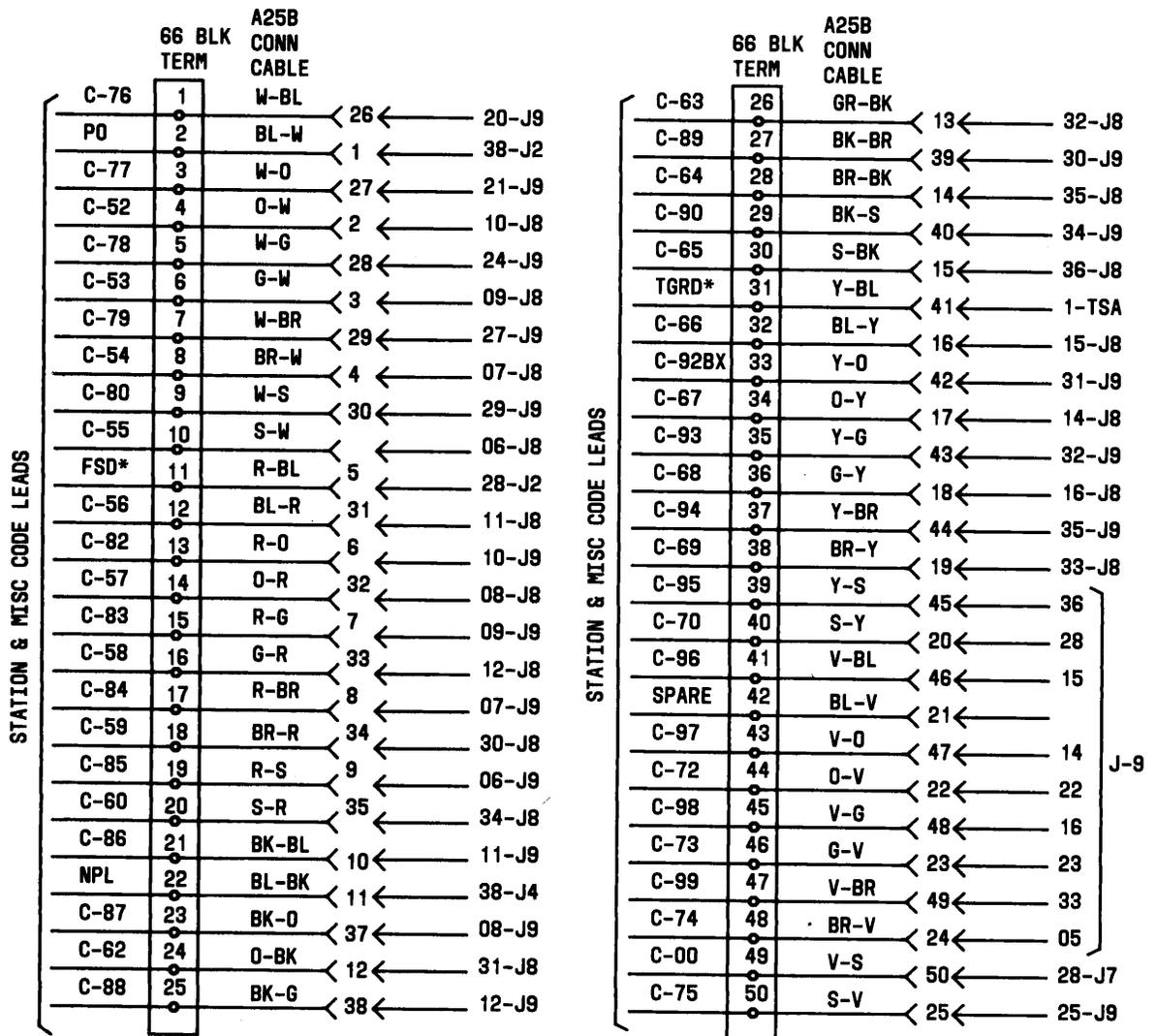
\* DENOTES THE TERMINALS TO BE STRAPPED TO SEND CONTINUOUS 2600-HZ TONE TO THE STC FOR CIRCUIT LINEUP PROCEDURES.
