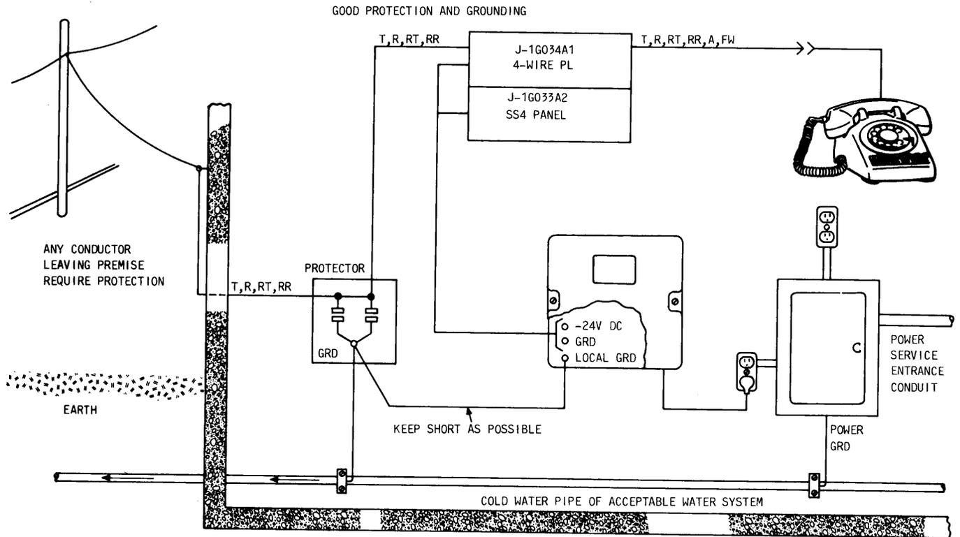
Fig. 33—System Grounding
