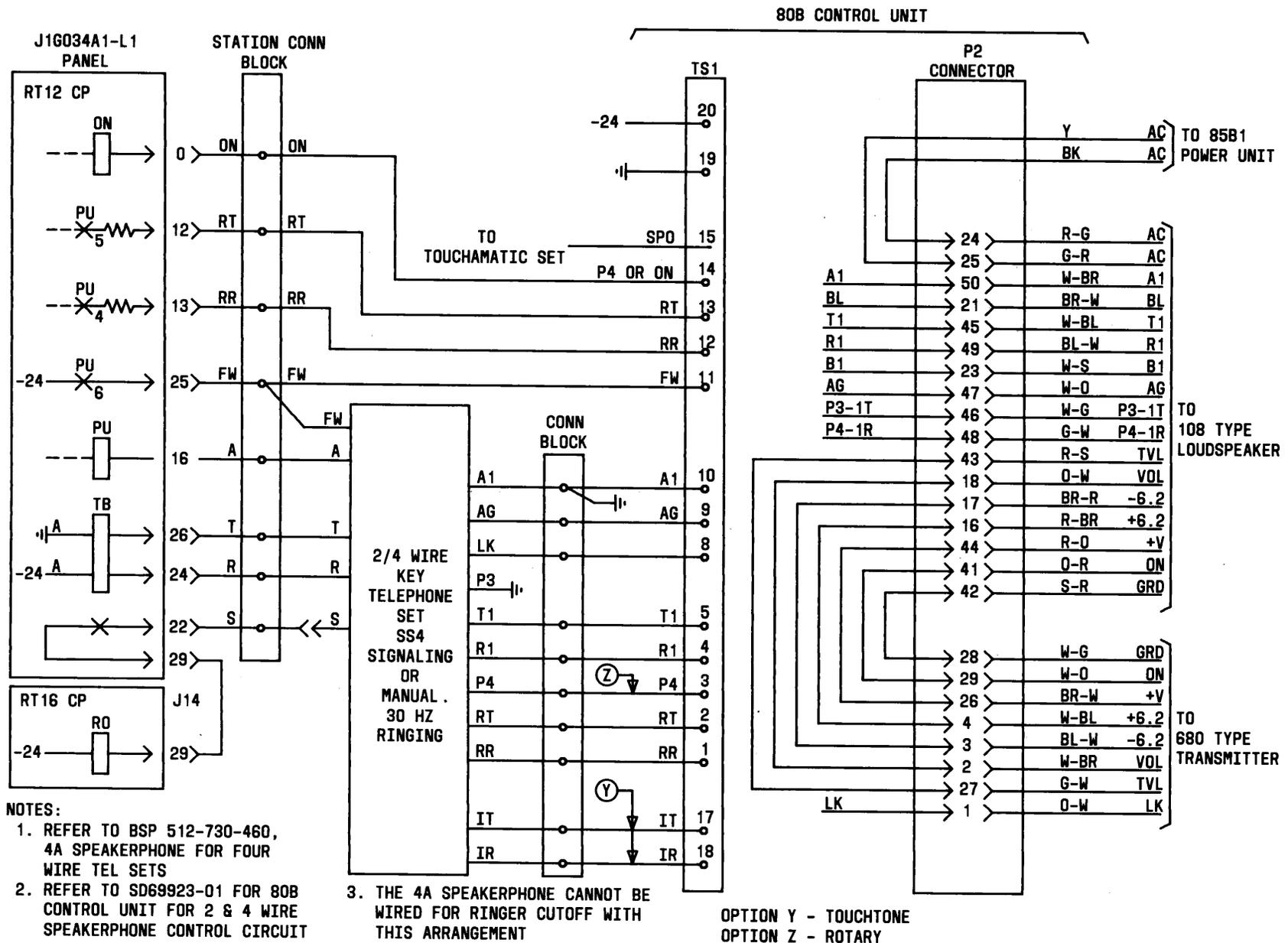
Fig. 24—4A Speakerphone Connections
