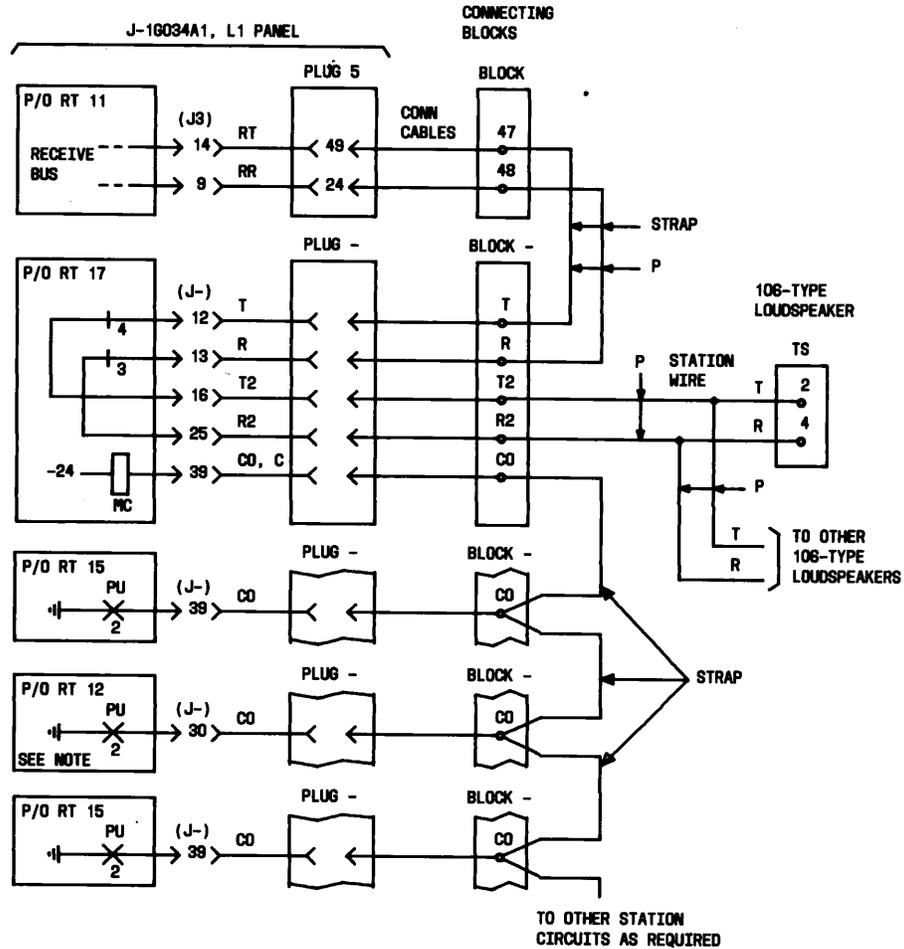
NOTE: WHERE THE RT 12 CP IS USED AS A STATION CIRCUIT IN A VOICE SIGNALING CIRCUIT, STRAP TERMINALS 12 AND 13 ON TERMINAL STRIP A OF THE J-16034A1, L1 PANEL
