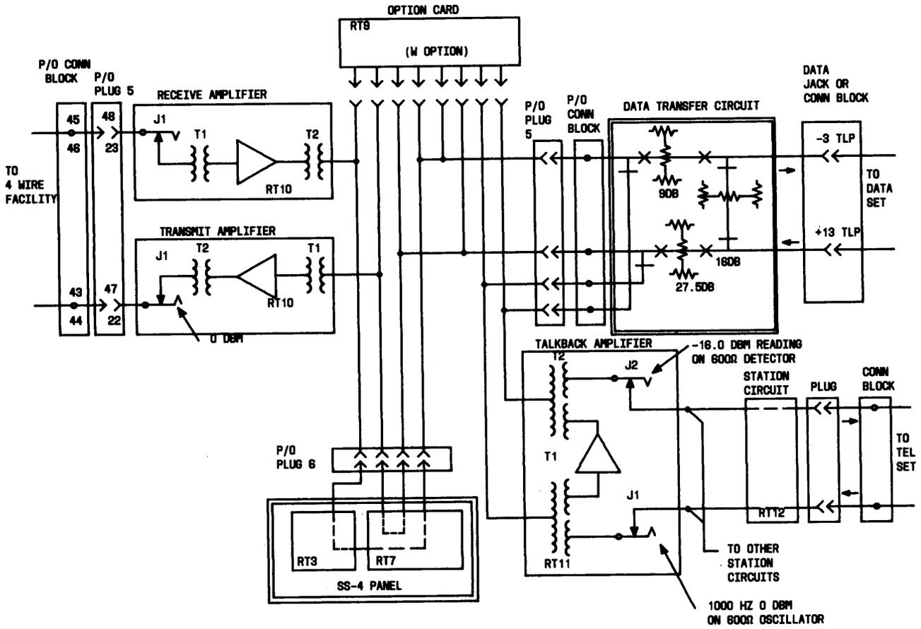
Fig. 32—Typical Transmission Diagram, SS-4 With Data Access
