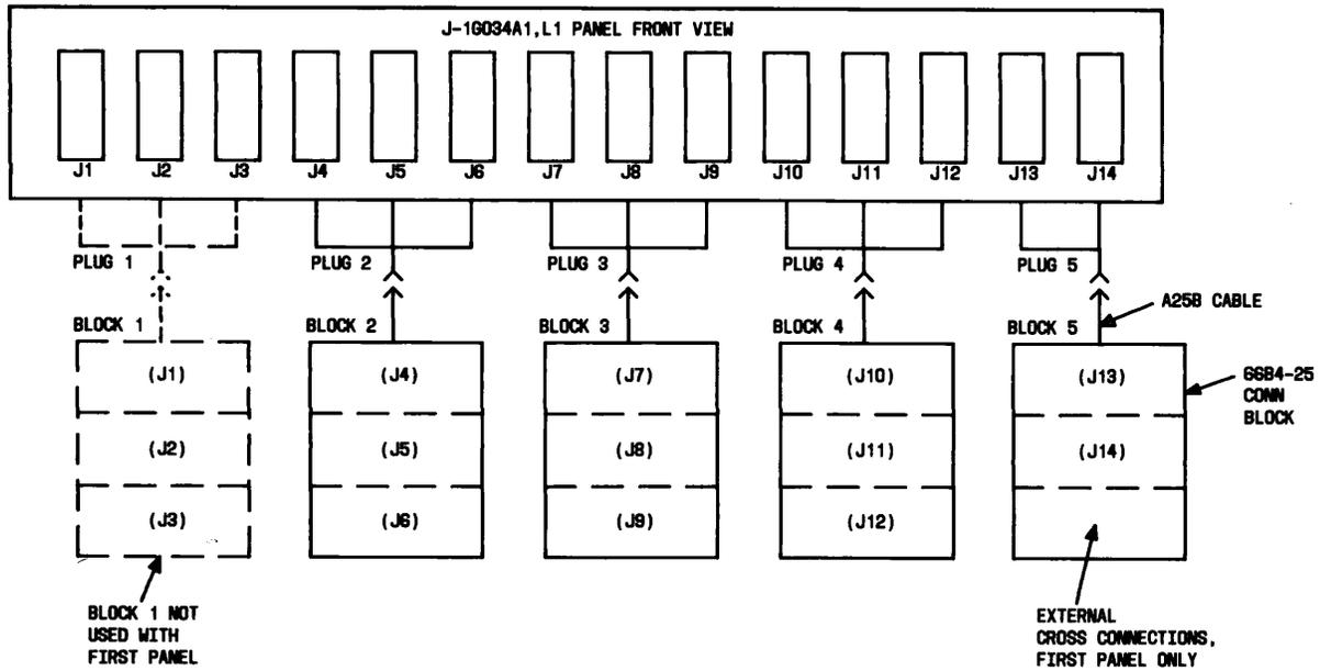
Fig. 8—▶Connecting Blocks Associated With Connectors in J1G034A-1,L1 Panel (Nonpackaged System)◆
