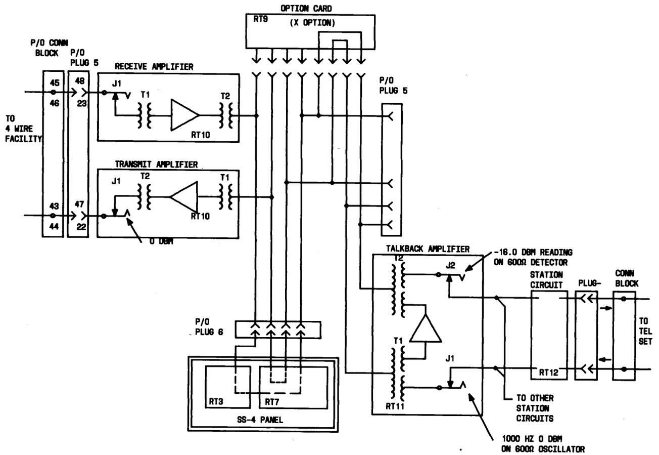
Fig. 31—Typical Transmission Diagram, SS-4 Without Data Access
