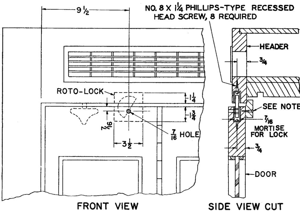
**Note:** Replace P-381074 (1-1/2 inch) door-stop screws with 1-inch wood screws (three required).
