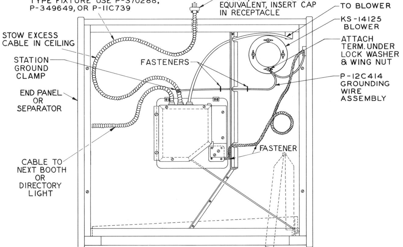
Fig. 4 - Typical Installation for 3-way Receptacle
