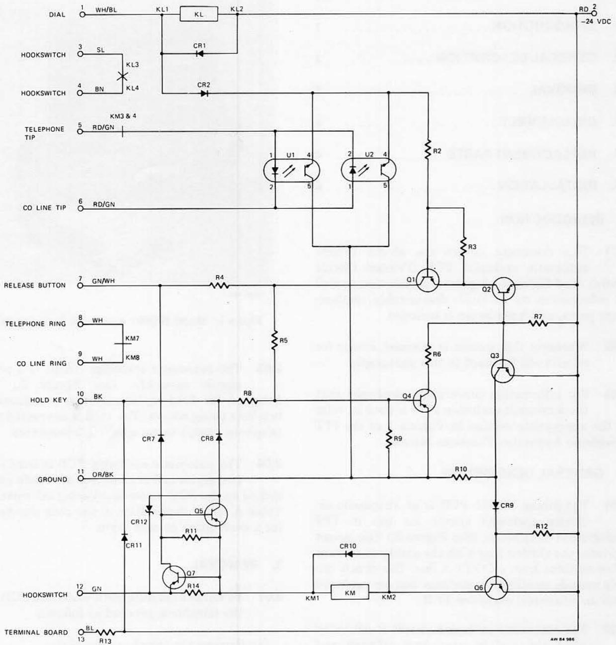
Figure 2: Model 182691 Automatic Exclusion PCB, Schematic
