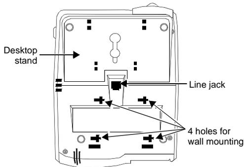
**Figure 2. The Bottom of the 6200 Series Telephones**
