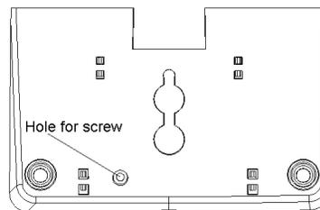
**Figure 5. Tightening the Stand to Back of the Telephone**
