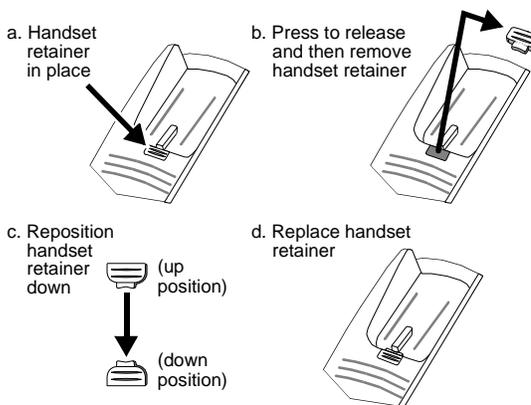
**Figure 6. Reversing the Handset Hook**
