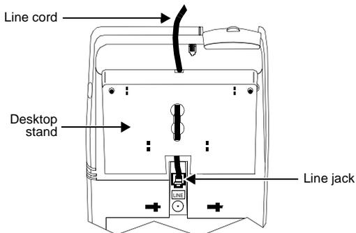
**Figure 4. Attaching the Line Cord and Threading It Through the Slot at the Top of the Desktop Stand**
