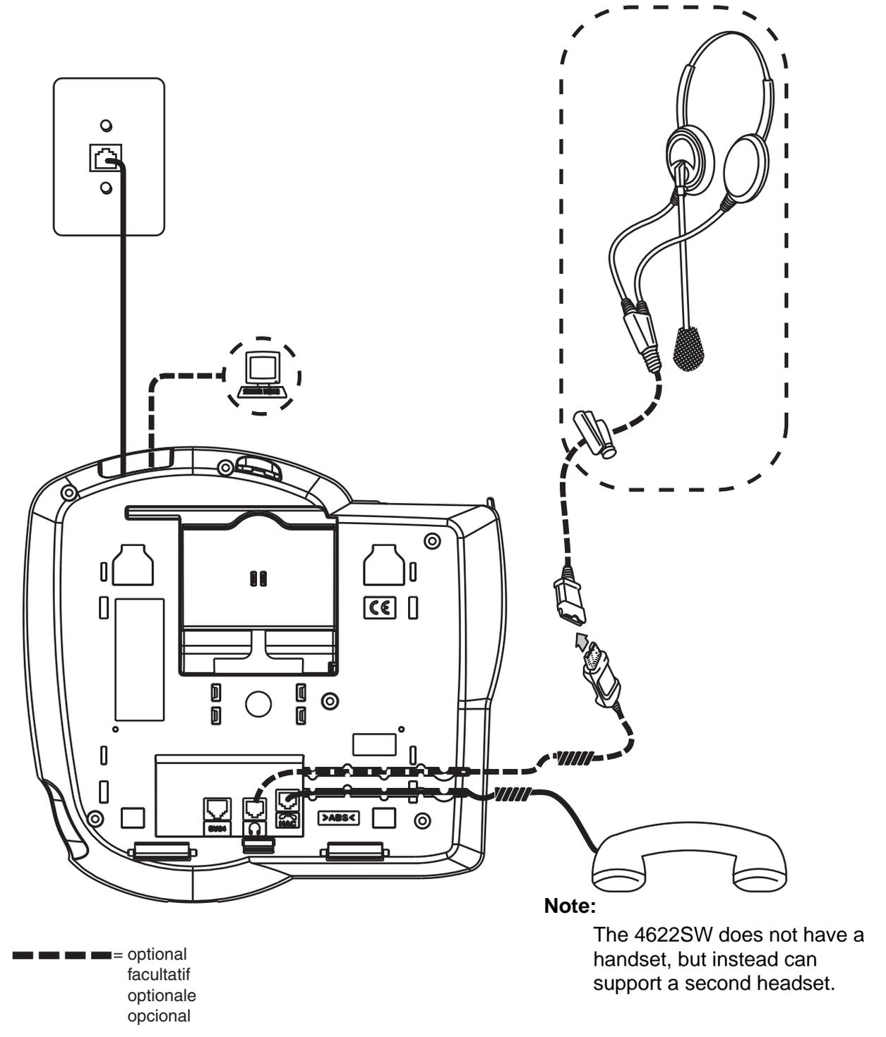
Figure 6: Connection Jacks on a 4630 IP Telephone
