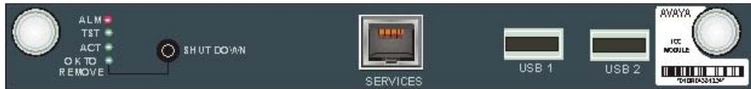
The S8300 Media Server has a total of 4 LEDs on the faceplate ([Figure 19: S8300 Media Server](#) on page 301), the three standard LEDs and one additional LED:
