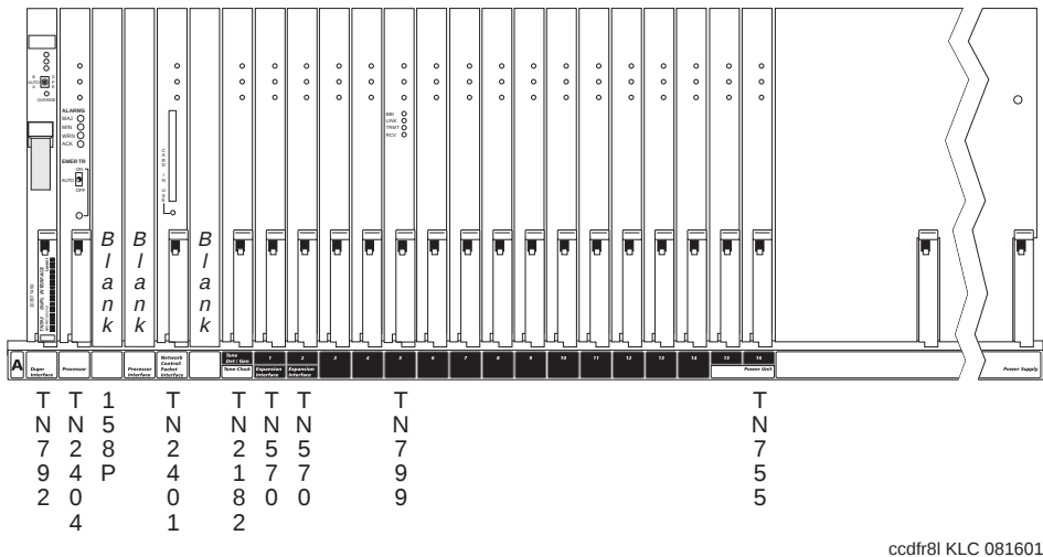
Figure 54: SCC1 basic control cabinet (front)
