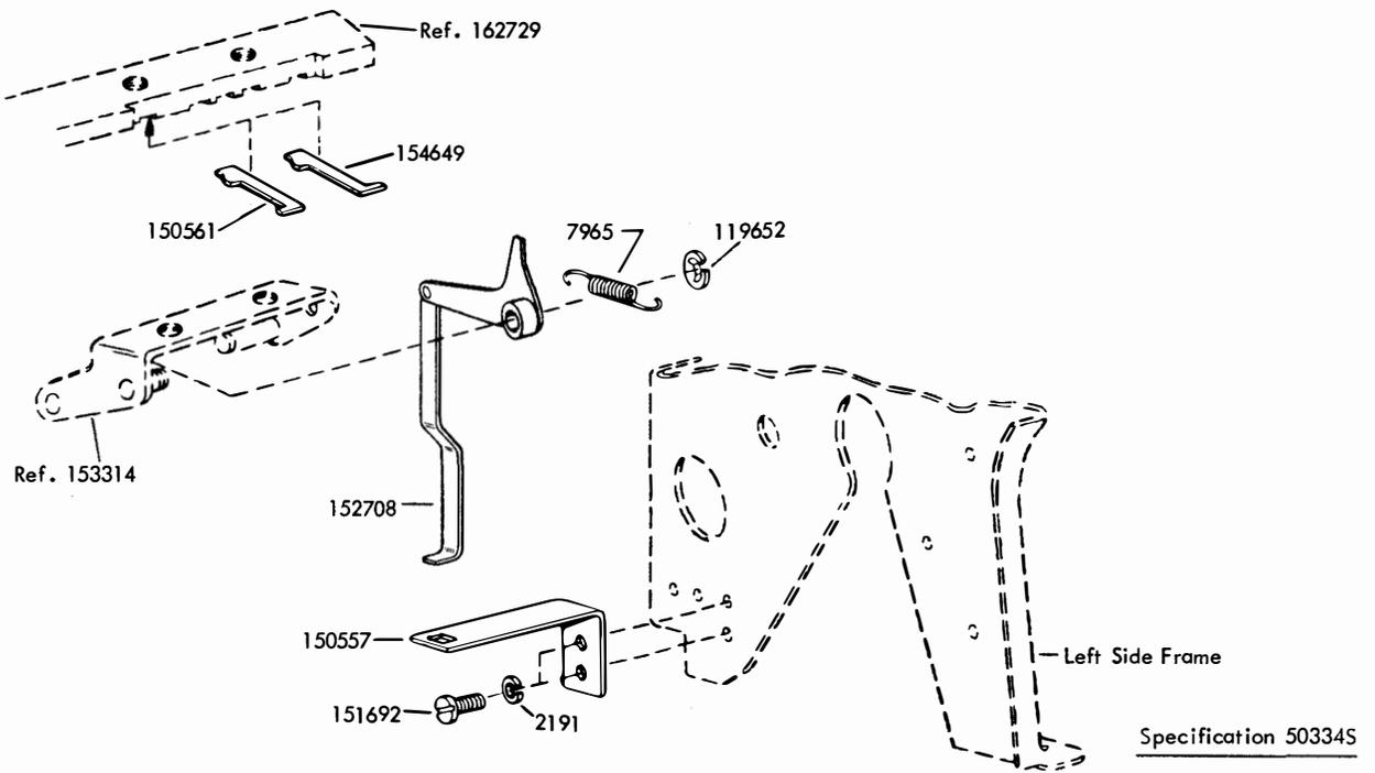
FIGURE 83. 152350 MODIFICATION KIT TO PROVIDE KEYBOARD LOCK
