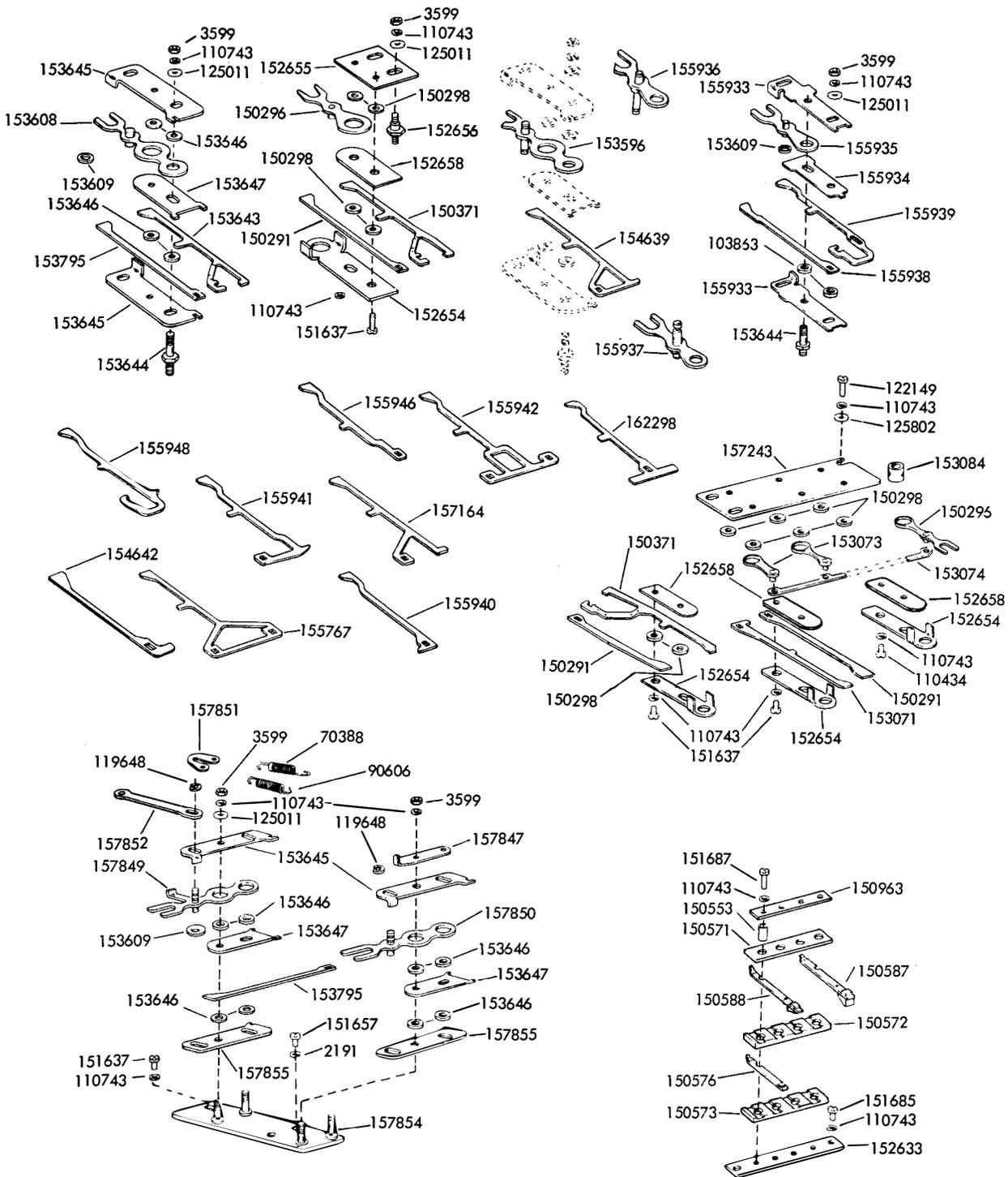
FIGURE 57. SHIFT MECHANISM COMPONENTS
