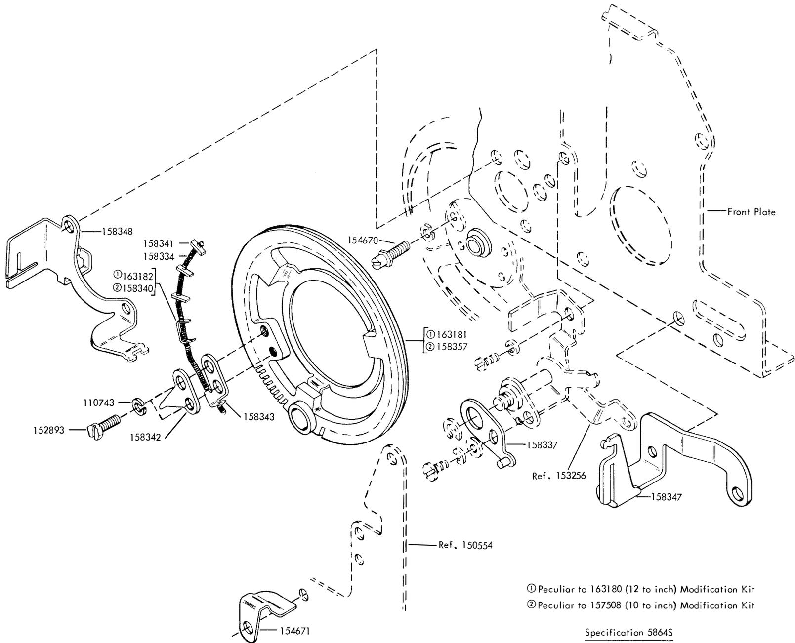
FIGURE 104. 157508 AND 163180 MODIFICATION KITS TO PROVIDE HORIZONTAL TABULATION
