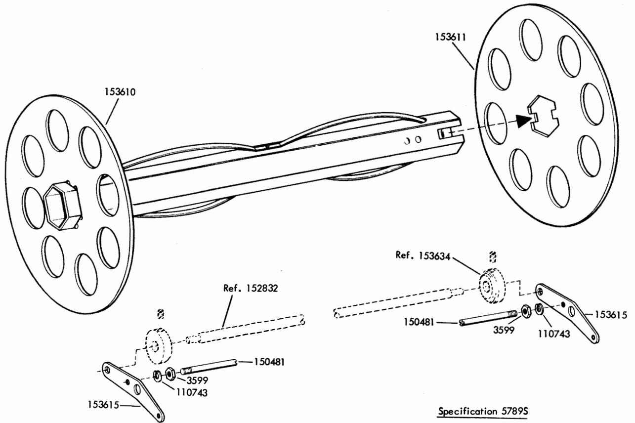
FIGURE 80. 152340 MODIFICATION KIT TO PROVIDE MULTI-COPY PAPER HANDLING
