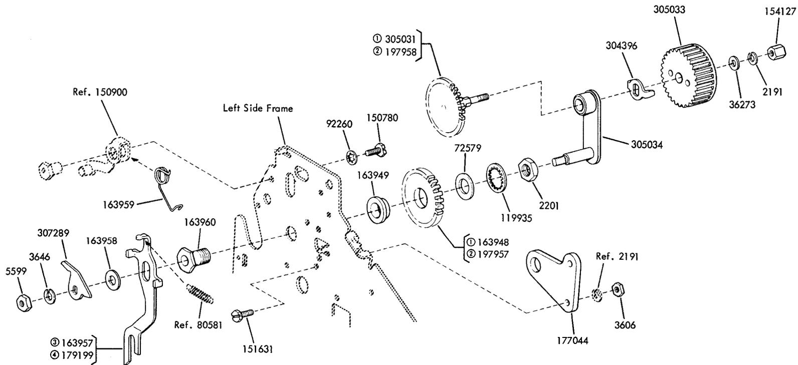
FIGURE 126. 305035, 305036 AND 307065 MODIFICATION KITS TO PROVIDE IMPROVED MANUAL PLATEN LINE FEED
