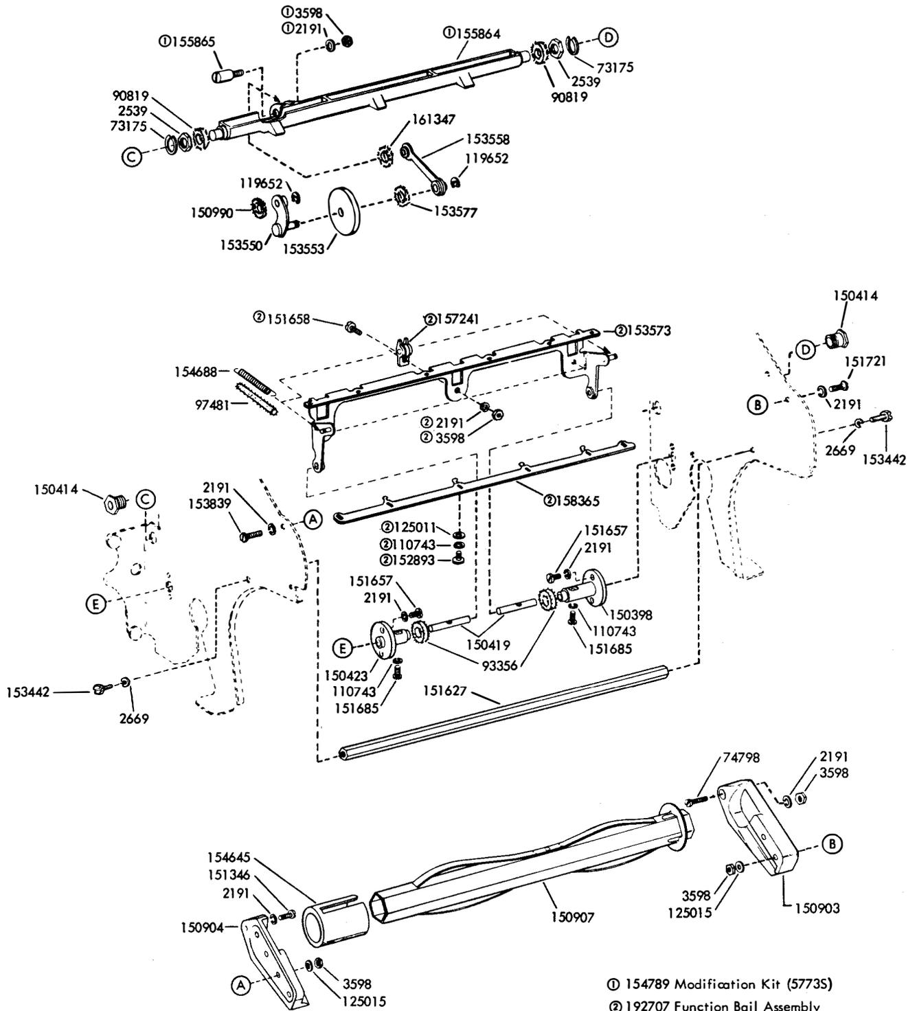
FIGURE 14. PAPER SPINDLE AND RESET BAIL MECHANISM
