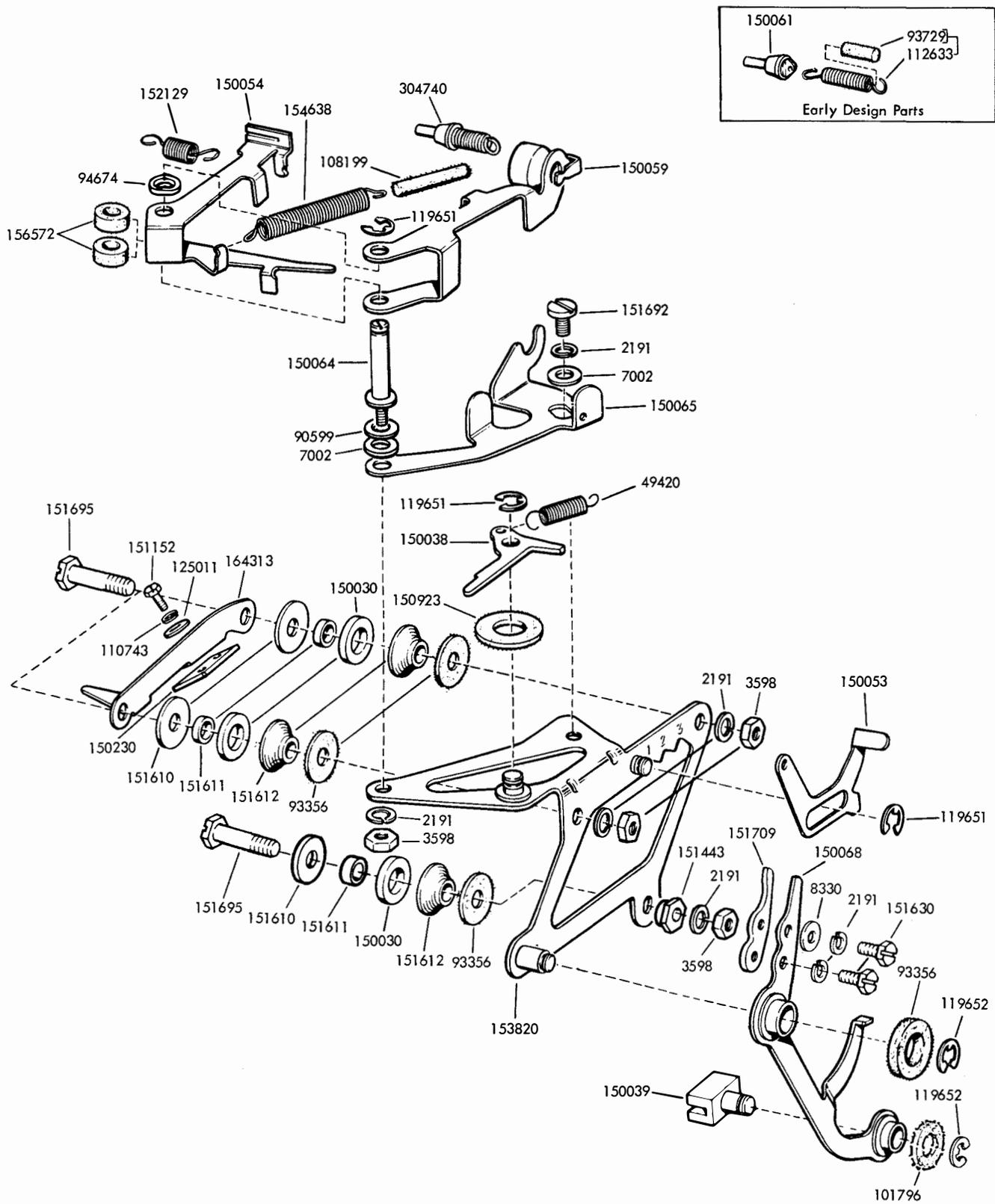
FIGURE 49. 150036 PRINTING CARRIAGE ASSEMBLY
