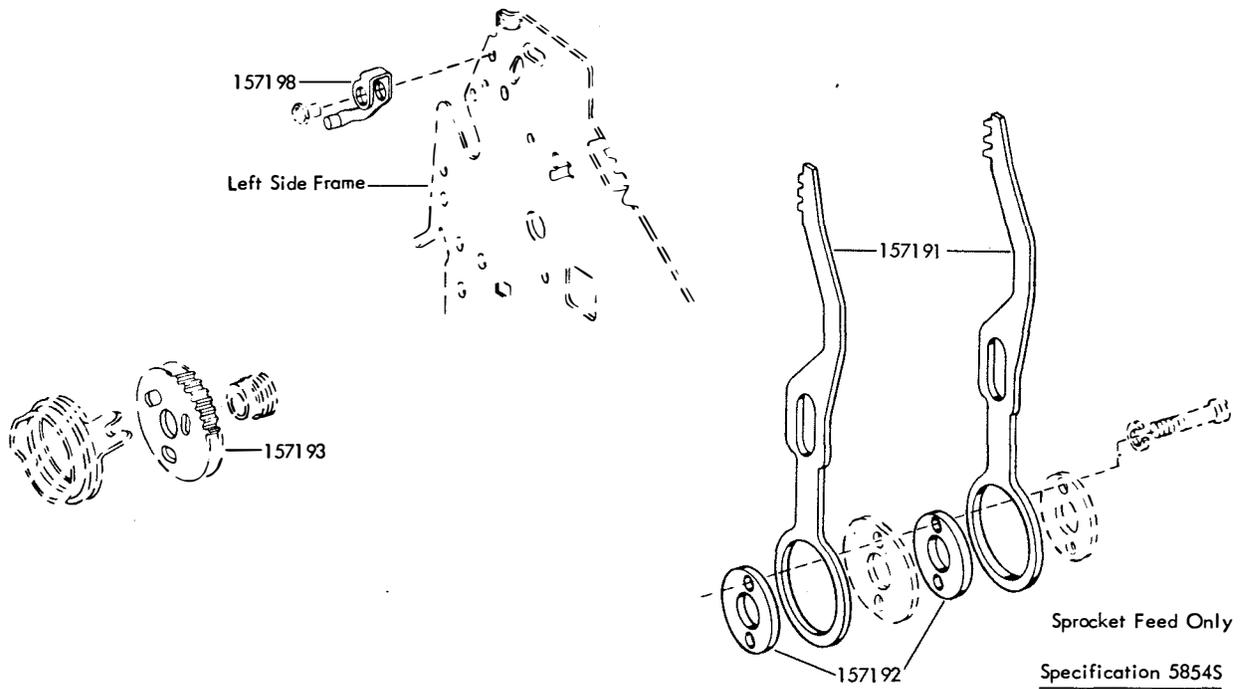
FIGURE 91. 154742 MODIFICATION KIT TO PROVIDE FOUR LINES PER INCH
