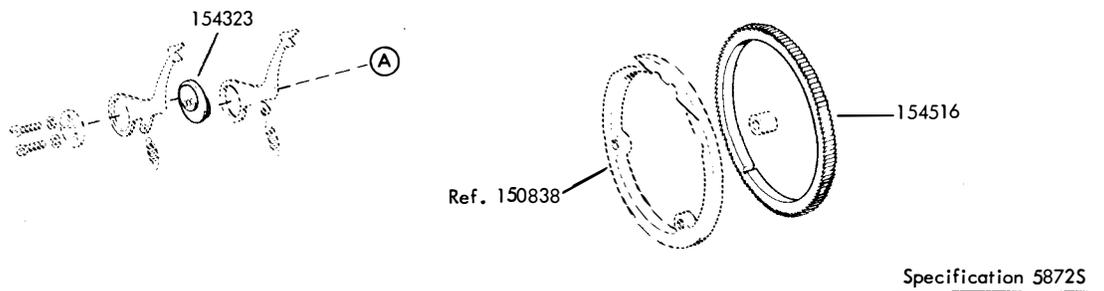
FIGURE 97. 154792 MODIFICATION KIT TO PROVIDE 12 SPACES PER INCH HORIZONTALLY
