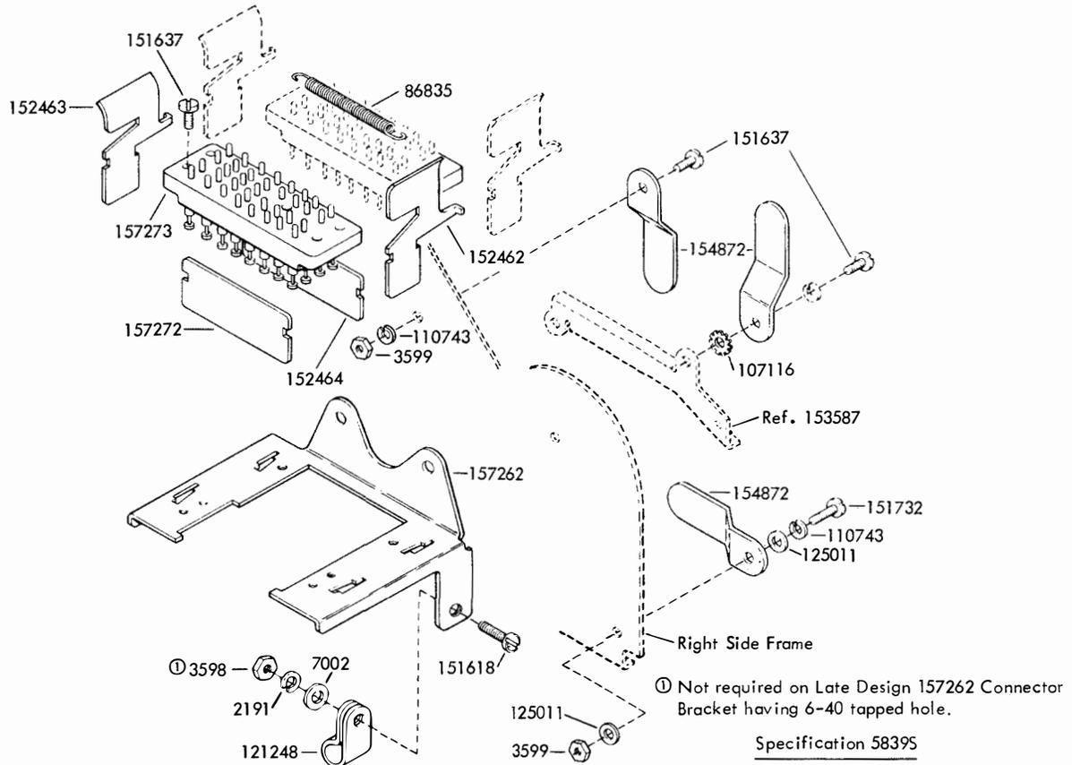
FIGURE 74. 154727 MODIFICATION KIT TO PROVIDE AUXILIARY CONNECTOR
