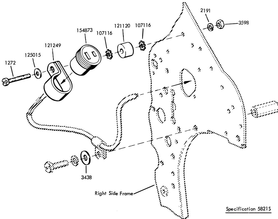
FIGURE 93. 154753 MODIFICATION KIT TO PROVIDE AUXILIARY CONNECTOR
