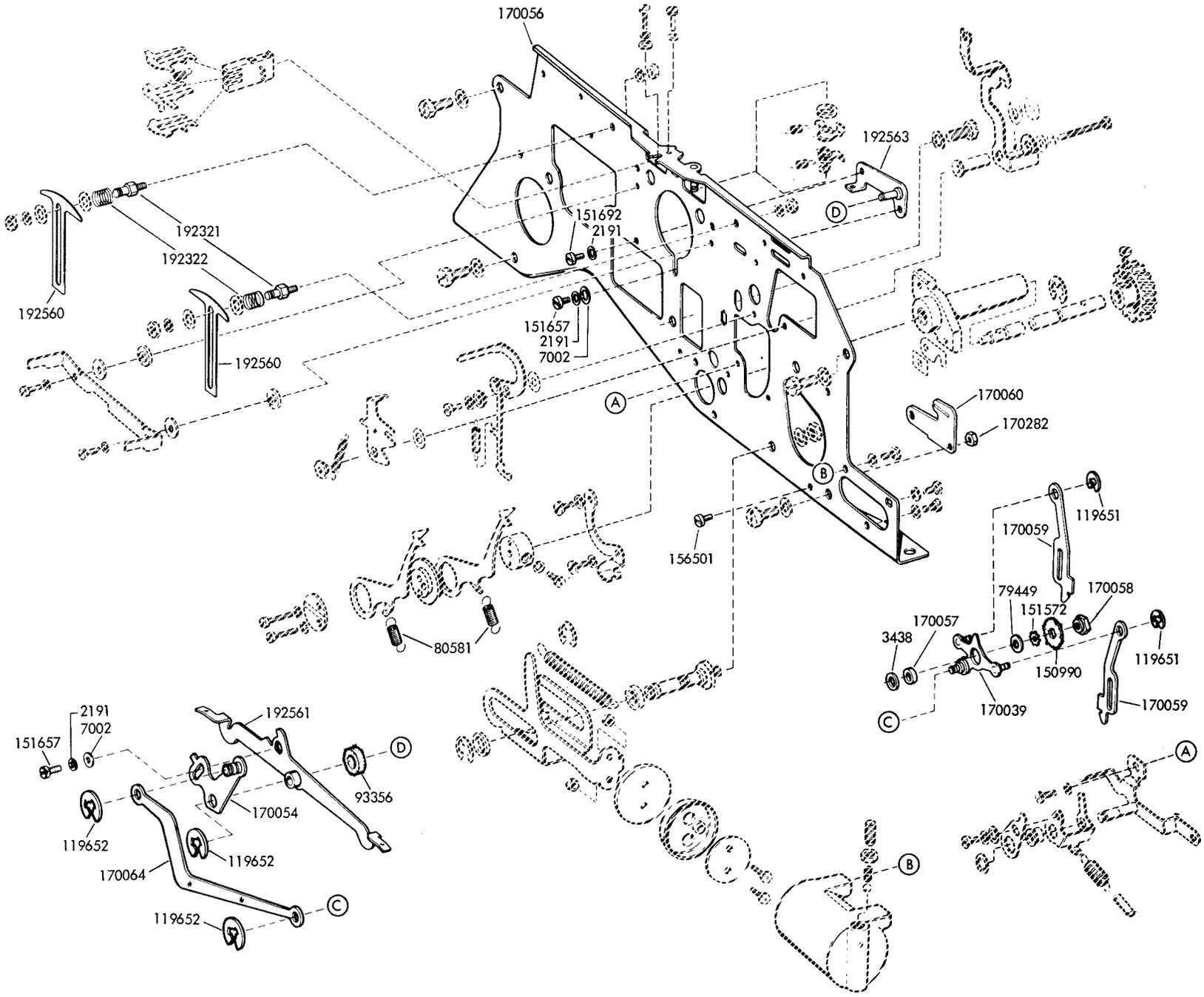
FIGURE 33. FRONT PLATE MECHANISM (8 LEVEL)
