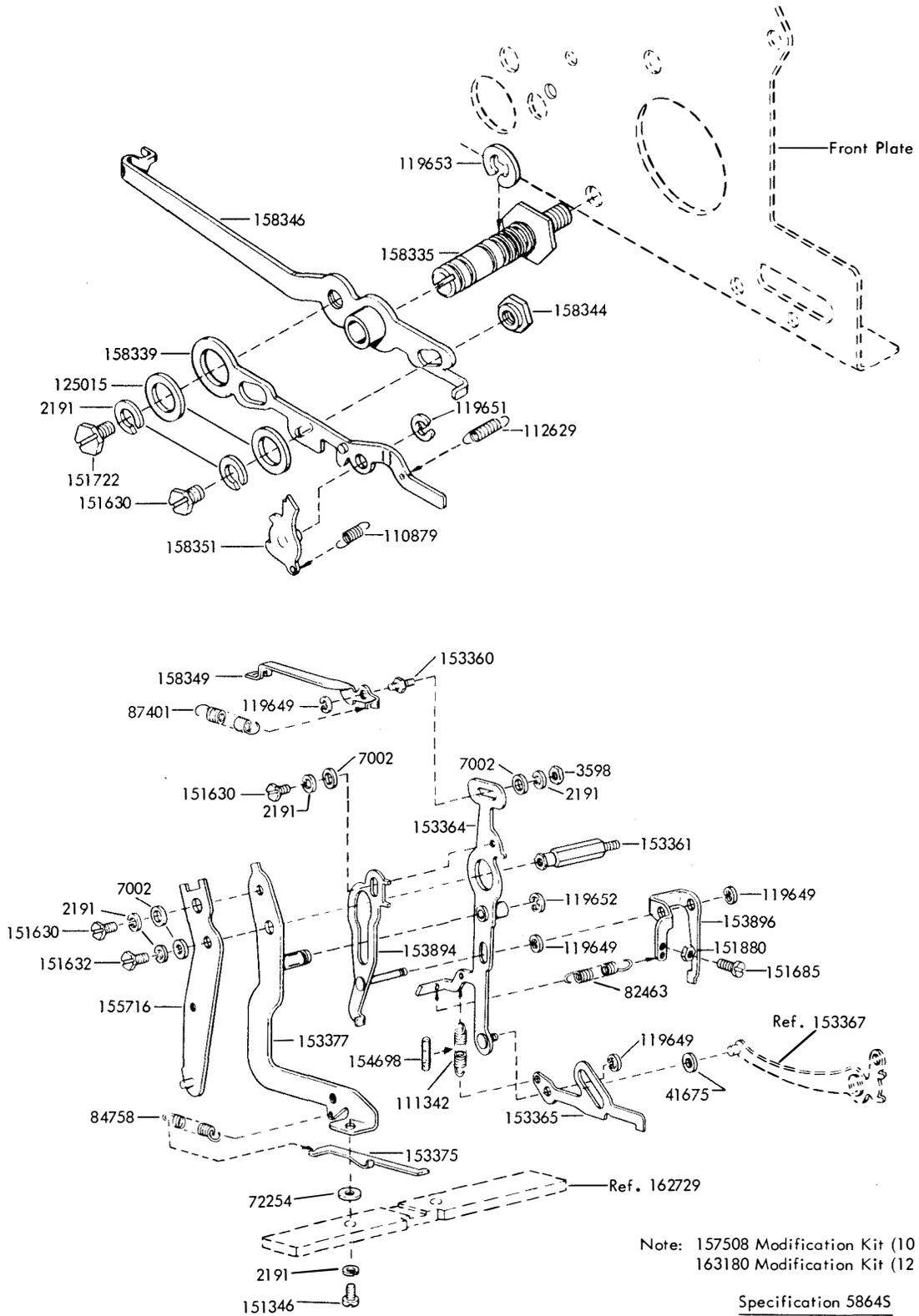
FIGURE 103. 157508 AND 163180 MODIFICATION KITS TO PROVIDE HORIZONTAL TABULATION
