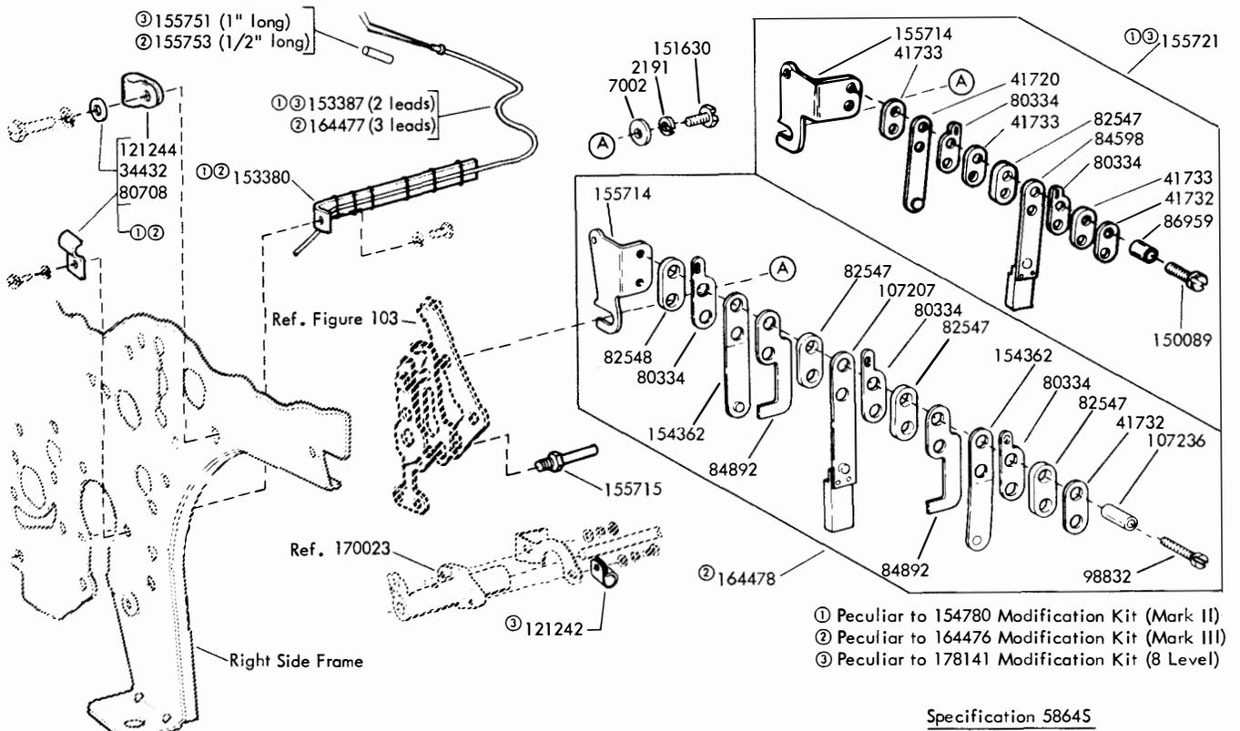
FIGURE 67. 154780, 164476 AND 178141 MODIFICATION KITS TO PROVIDE HORIZONTAL TABULATOR XD CONTROL
