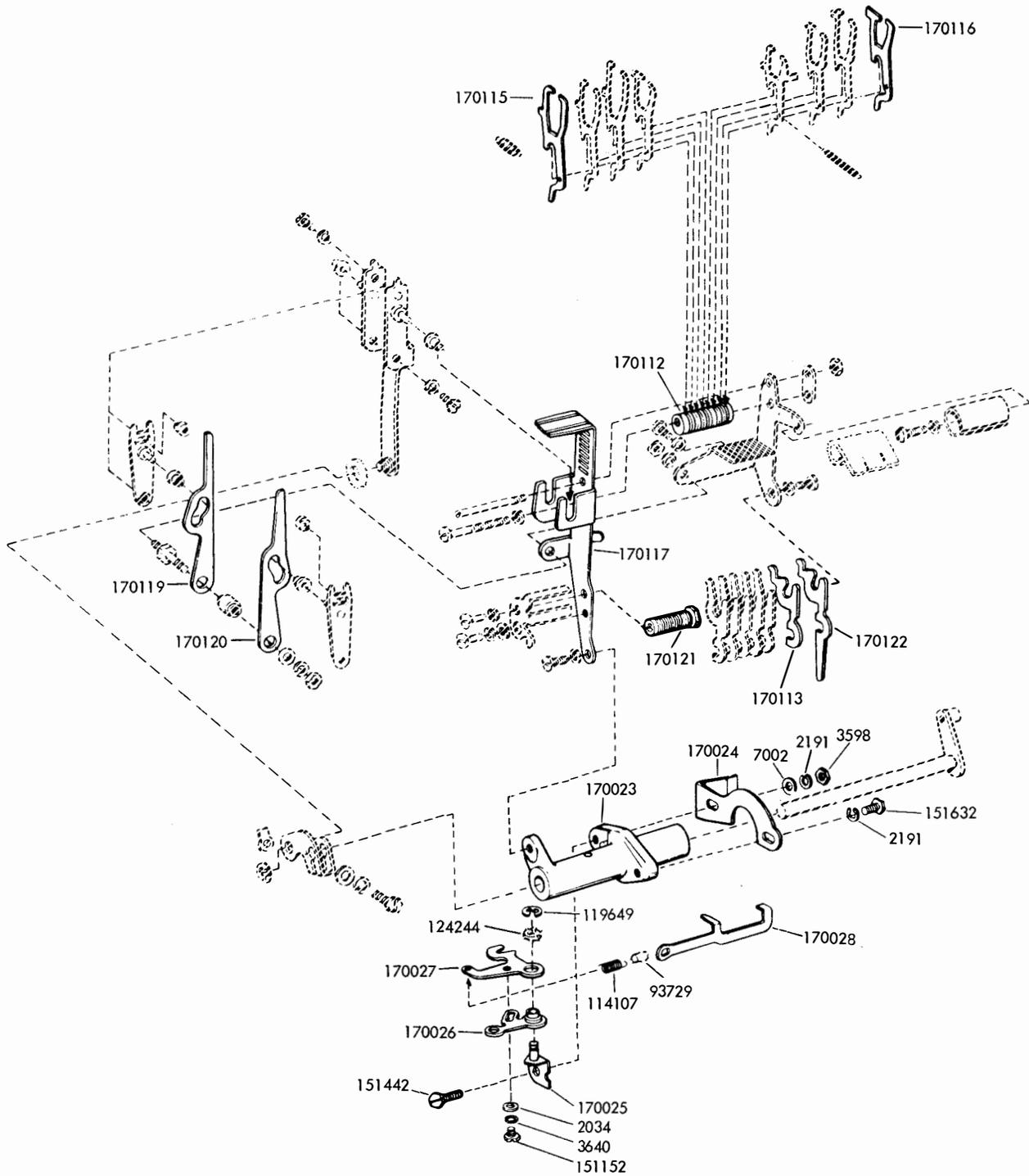
FIGURE 37. CODE BAR POSITIONING MECHANISM (8 LEVEL)
