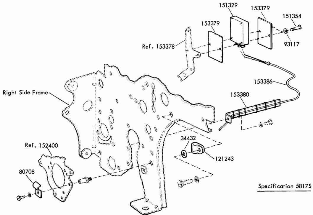
FIGURE 75. 152317 MODIFICATION KIT TO PROVIDE HORIZONTAL TABULATOR XD CONTROL
