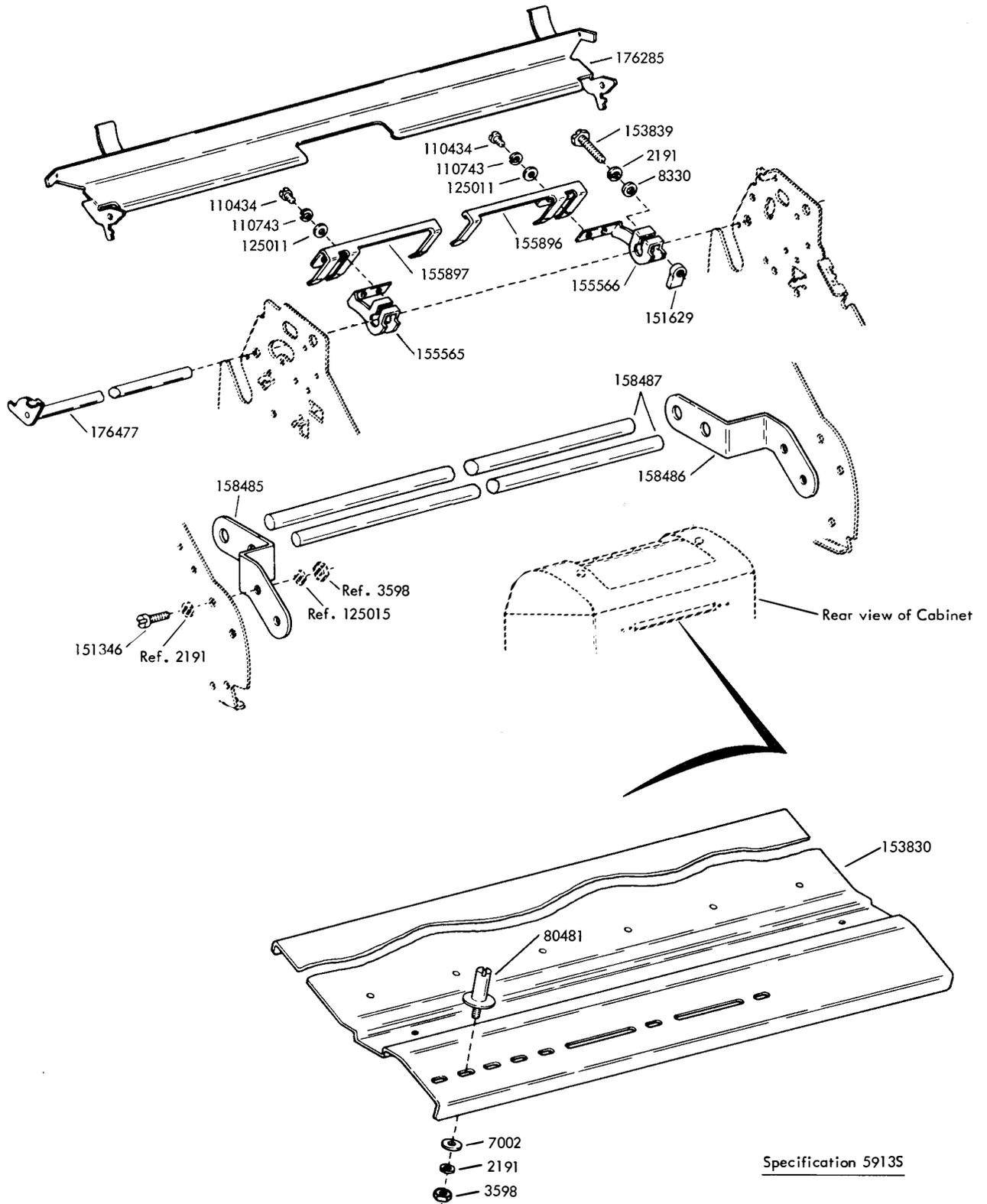
FIGURE 123. 154798 MODIFICATION KIT TO PROVIDE SUPERFOLD FRICTION FEED PAPER HANDLING
