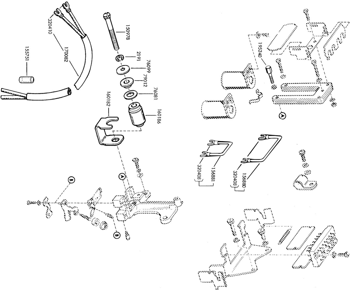
FIGURE 43. SELECTOR MAGNET MECHANISM (8 LEVEL)
