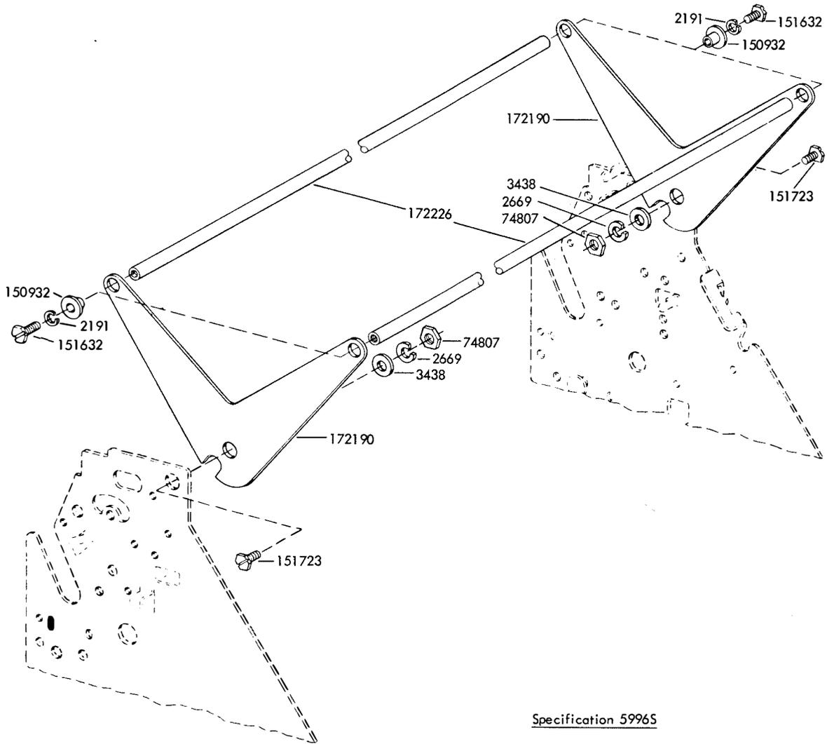
FIGURE 112. 172181 MODIFICATION KIT TO PROVIDE COPY DISPLAY
