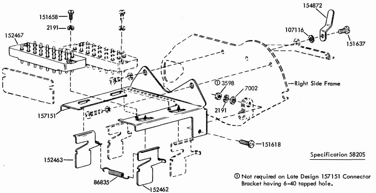
FIGURE 84. 153919 MODIFICATION KIT TO PROVIDE AUXILIARY CONNECTOR
