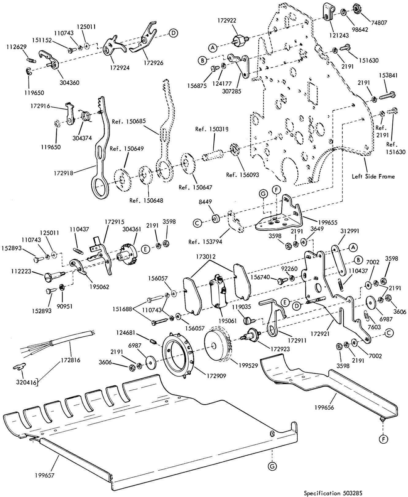
FIGURE 124. 194092 MODIFICATION KIT TO PROVIDE PAPER MOTION ALARM
