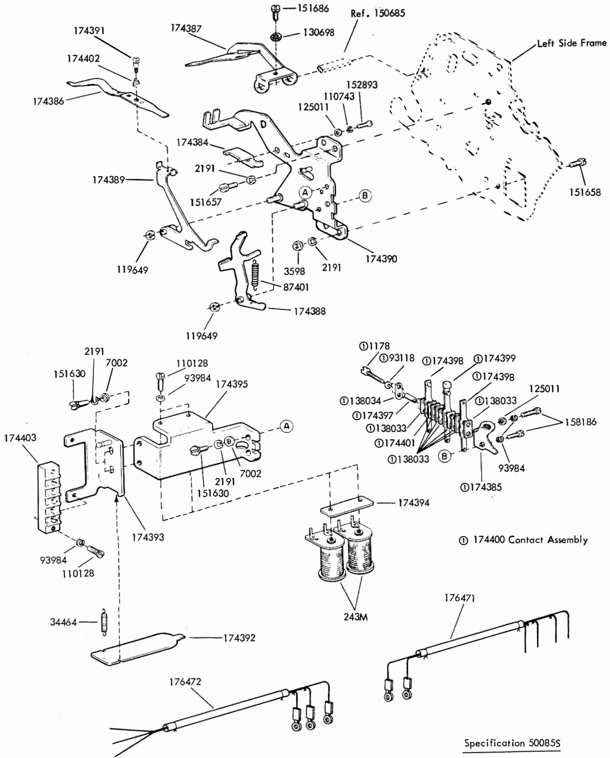
FIGURE 120. 174043 MODIFICATION KIT TO PROVIDE PAPER FEED FAILURE INDICATOR
