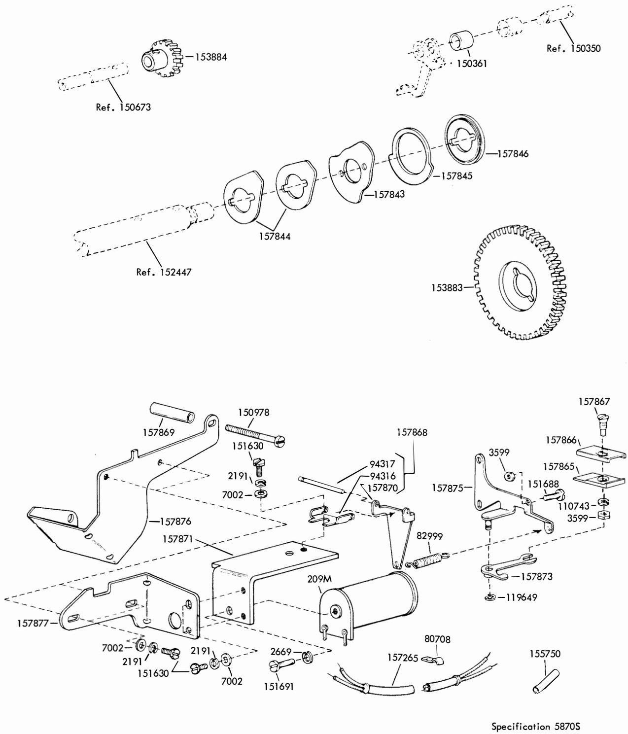
FIGURE 100. 154778 MODIFICATION KIT TO PROVIDE EXTERNAL PULSE SHIFT FEATURE
