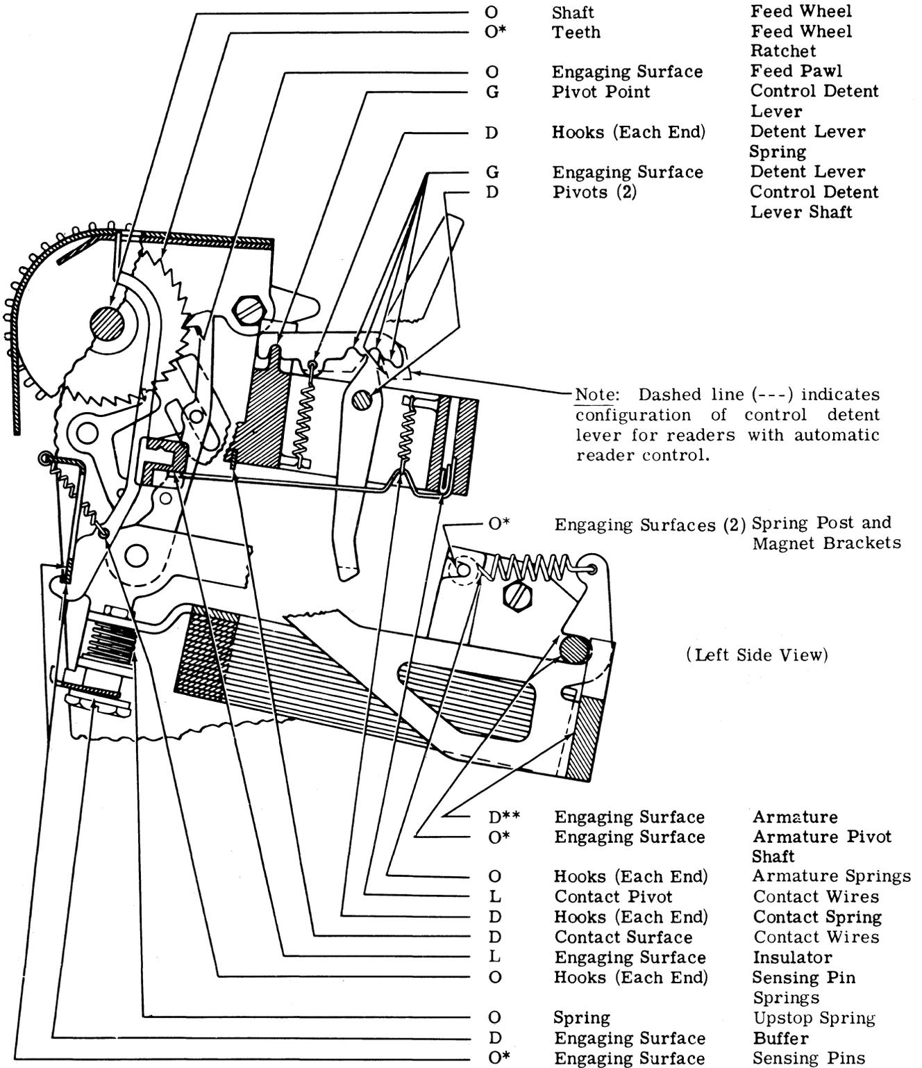
\*At 1500 hour lubrication intervals, apply with a coat of thoroughly mixed 50 percent KS7470 oil and 50 percent KS7471 grease.
