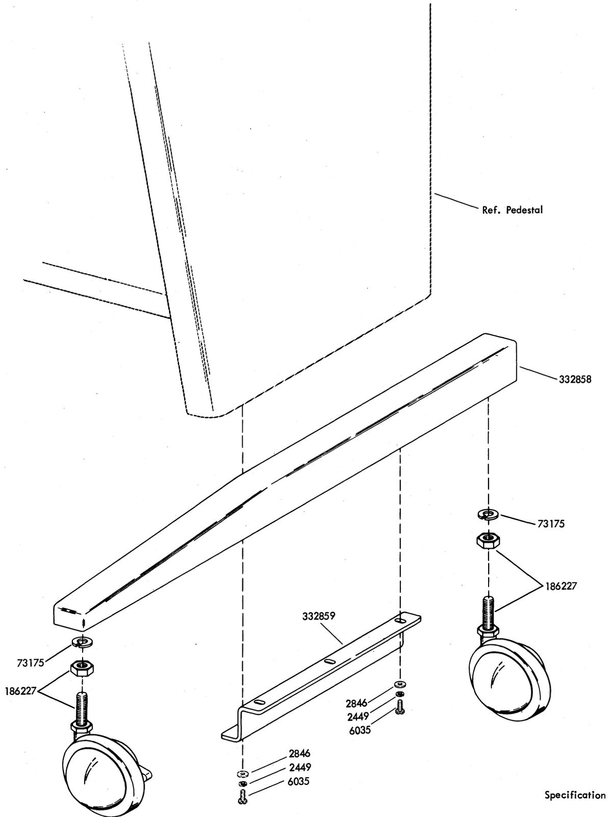
Fig. 17 — 333456 Modification Kit to Provide Mobility for Cabinet
