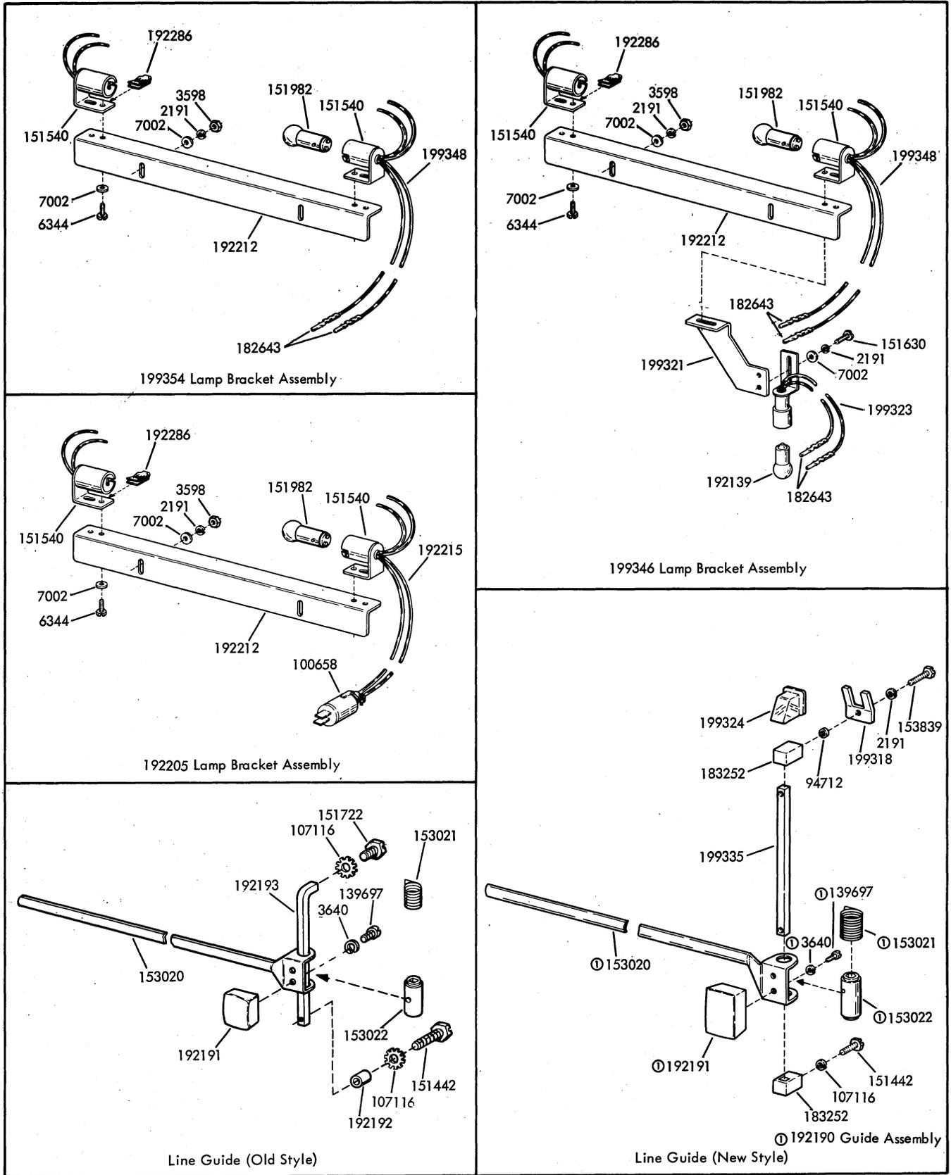
Fig. 13 — Lamp Brackets and Line Guides
