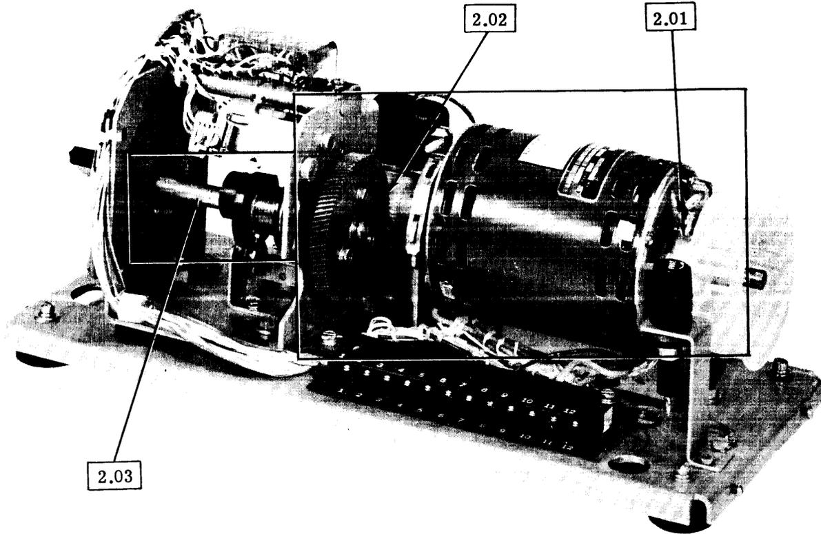
2.01 Motor (Lubricate every 1500 hours of continuous operating time or every six months, whichever occurs first).
