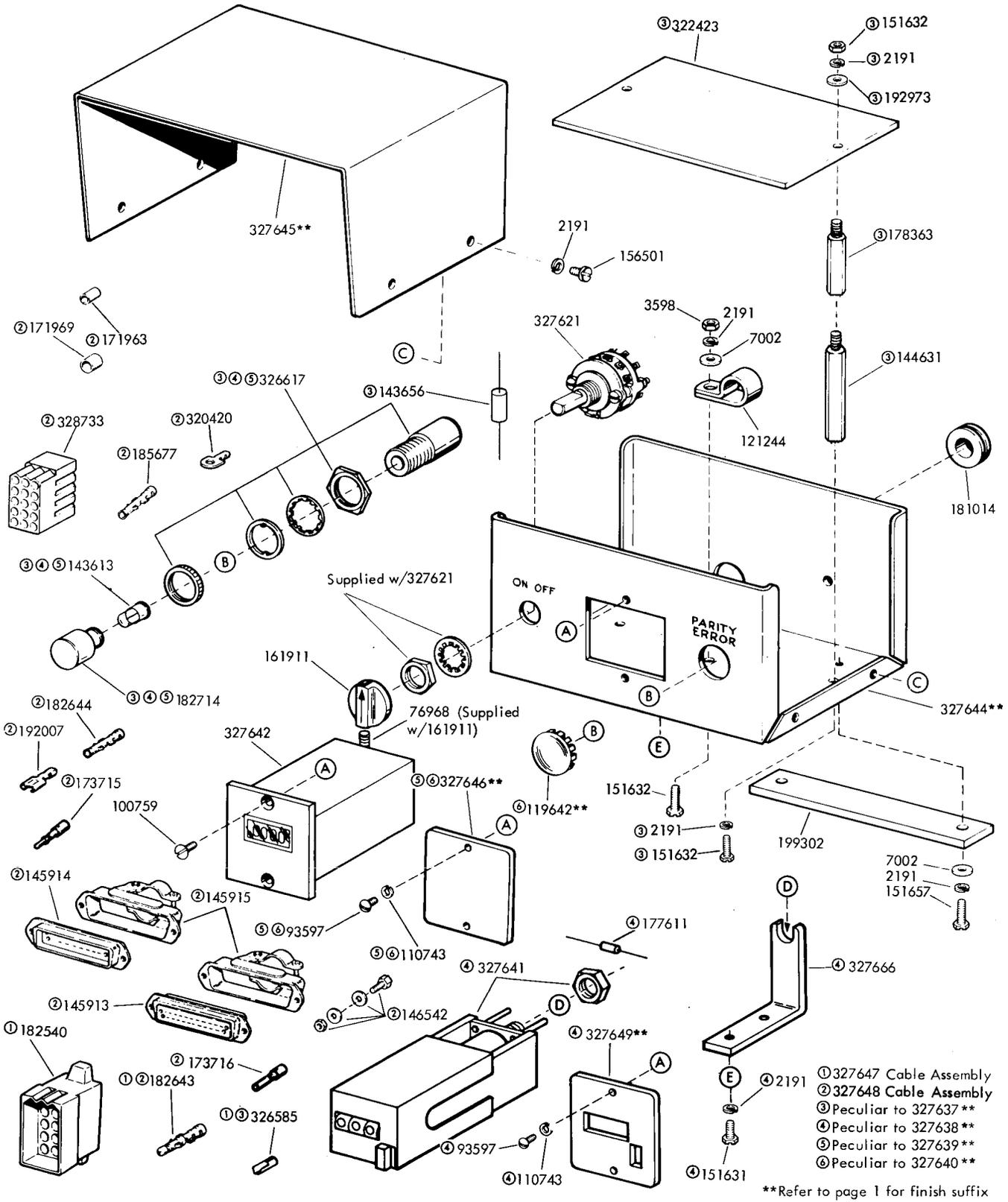
FIGURE 3. 327637\*\*, 327638\*\*, 327639\*\* INDICATOR ASSEMBLIES AND 327640\*\* BYPASS SWITCH ASSEMBLY
