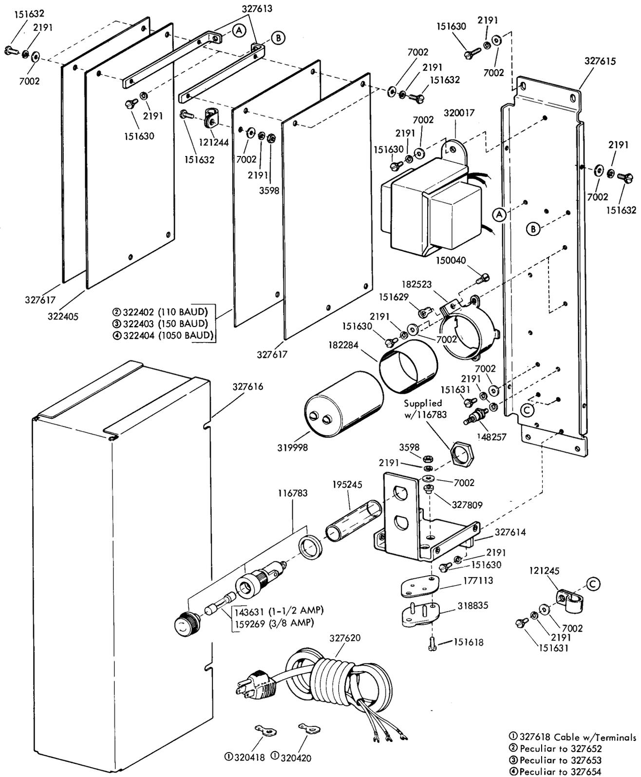
FIGURE 1. 327652, 327653 AND 327654 BASE PLATE ASSEMBLIES
