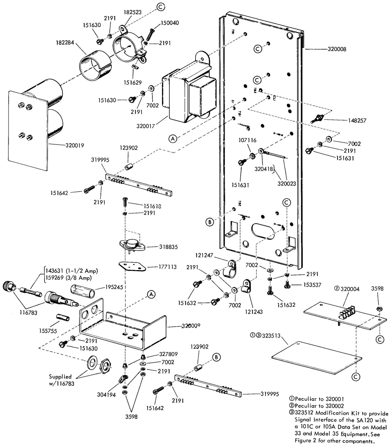
FIGURE 1. 320001 AND 320002 BASE PLATE ASSEMBLIES
