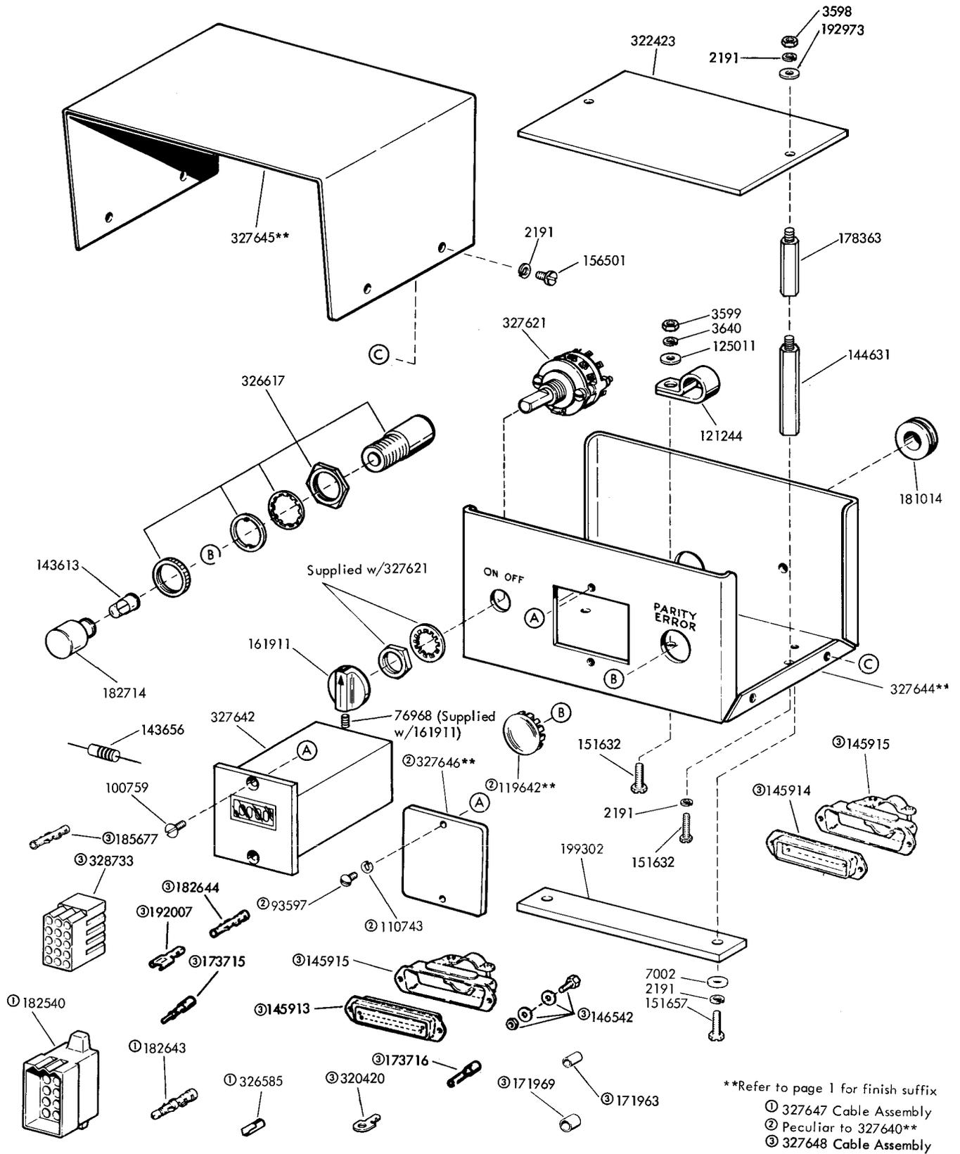
FIGURE 4. 327637\*\* INDICATOR ASSEMBLY AND 327640\*\* BYPASS SWITCH ASSEMBLY
