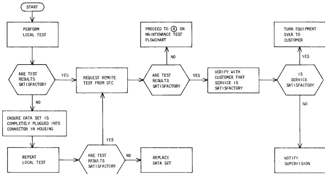
Fig. 4—Installation Test Sequence
