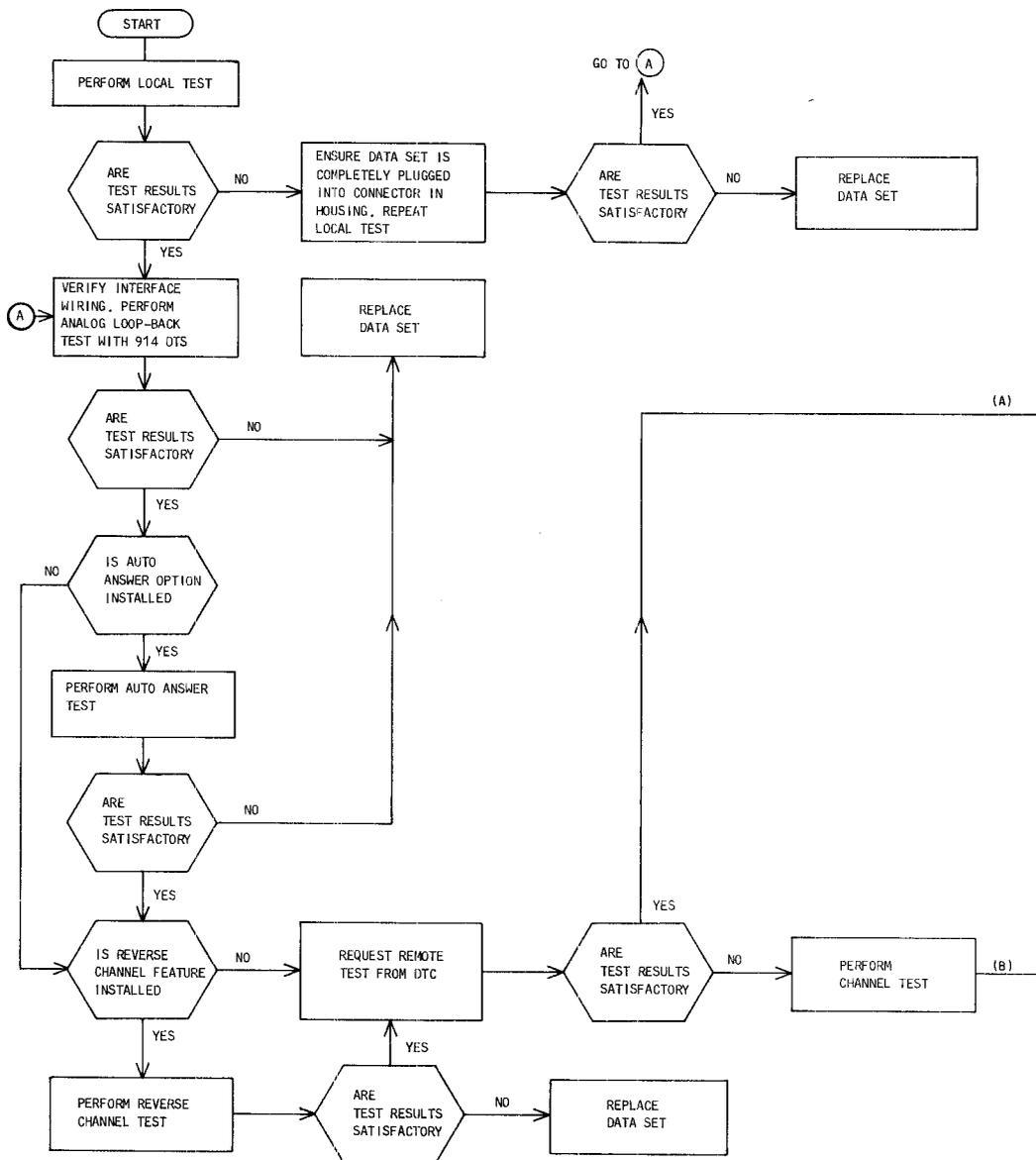
Fig. 6—Maintenance Test Flowchart (Sheet 1 of 2)
