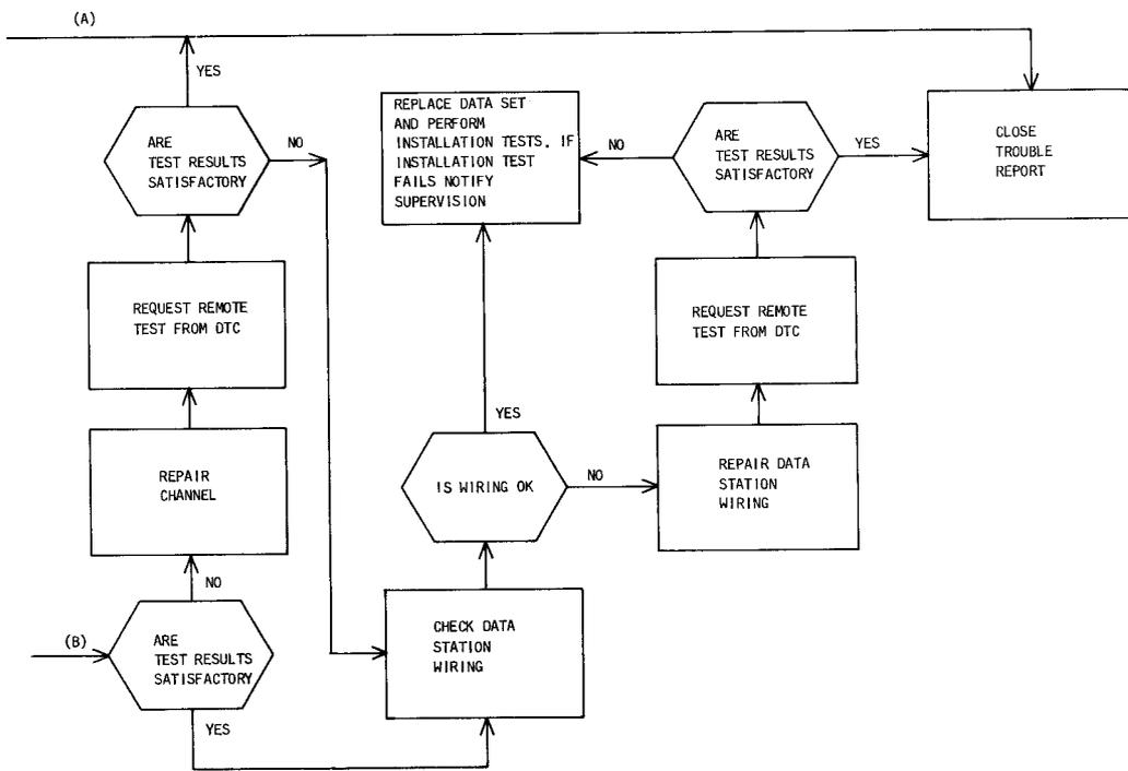
Fig. 6—Maintenance Test Flowchart (Sheet 2 of 2)
