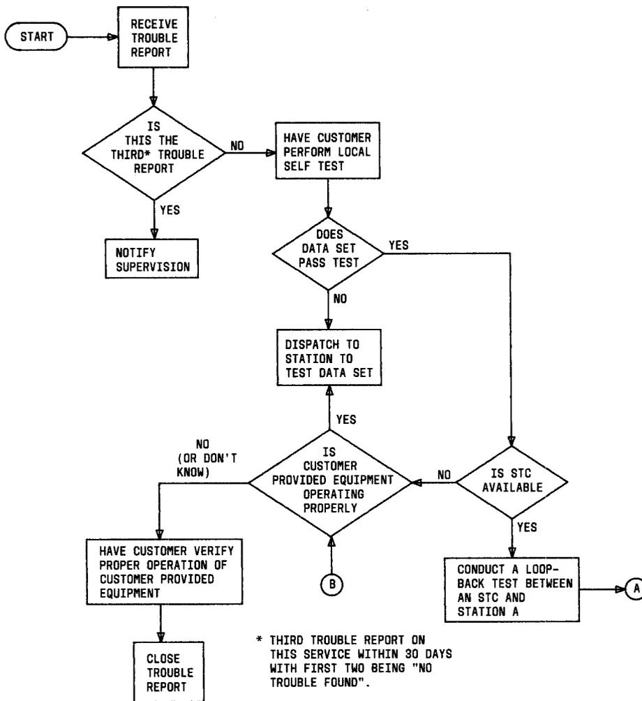
Fig. 4—4-Wire Maintenance Flowchart (Sheet 1 of 2)
