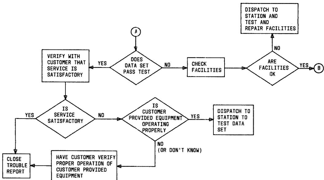
Fig. 3—2-Wire Maintenance Flowchart (Sheet 2 of 2)
