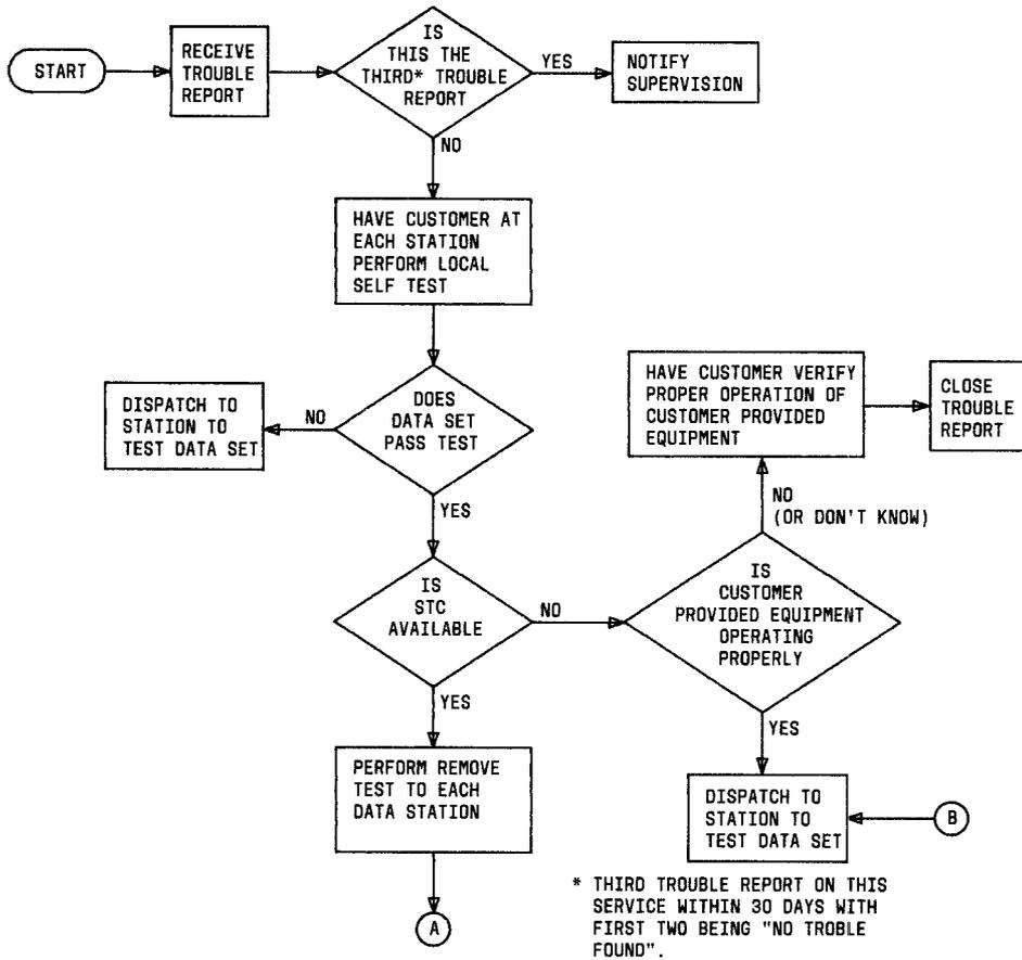
Fig. 3—2-Wire Maintenance Flowchart (Sheet 1 of 2)
