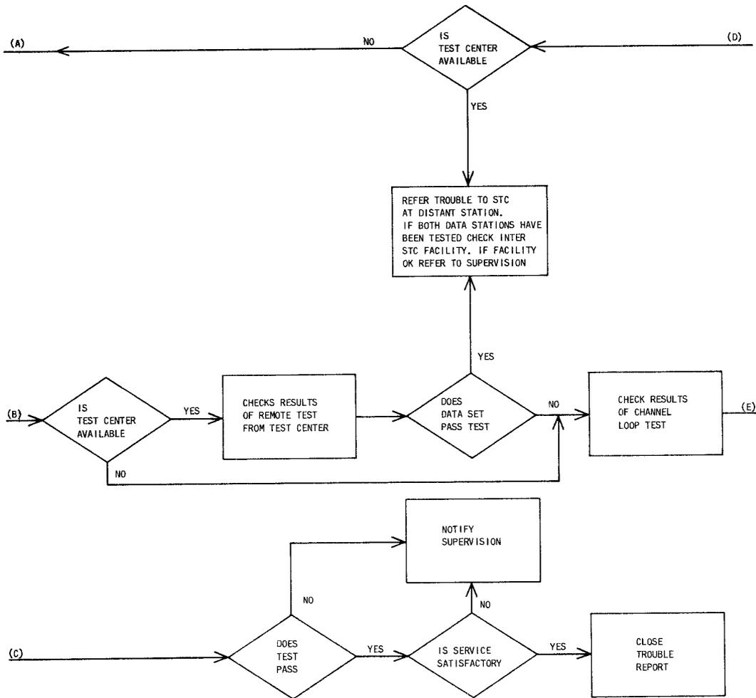
Fig. 6—4-Wire Maintenance Test Sequence (Sheet 2 of 3)
