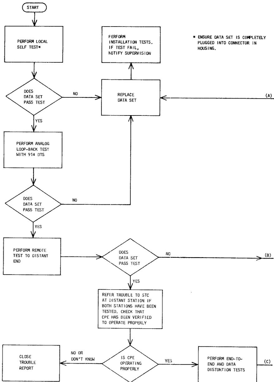
Fig. 6—4-Wire Maintenance Test Sequence (Sheet 1 of 3)
