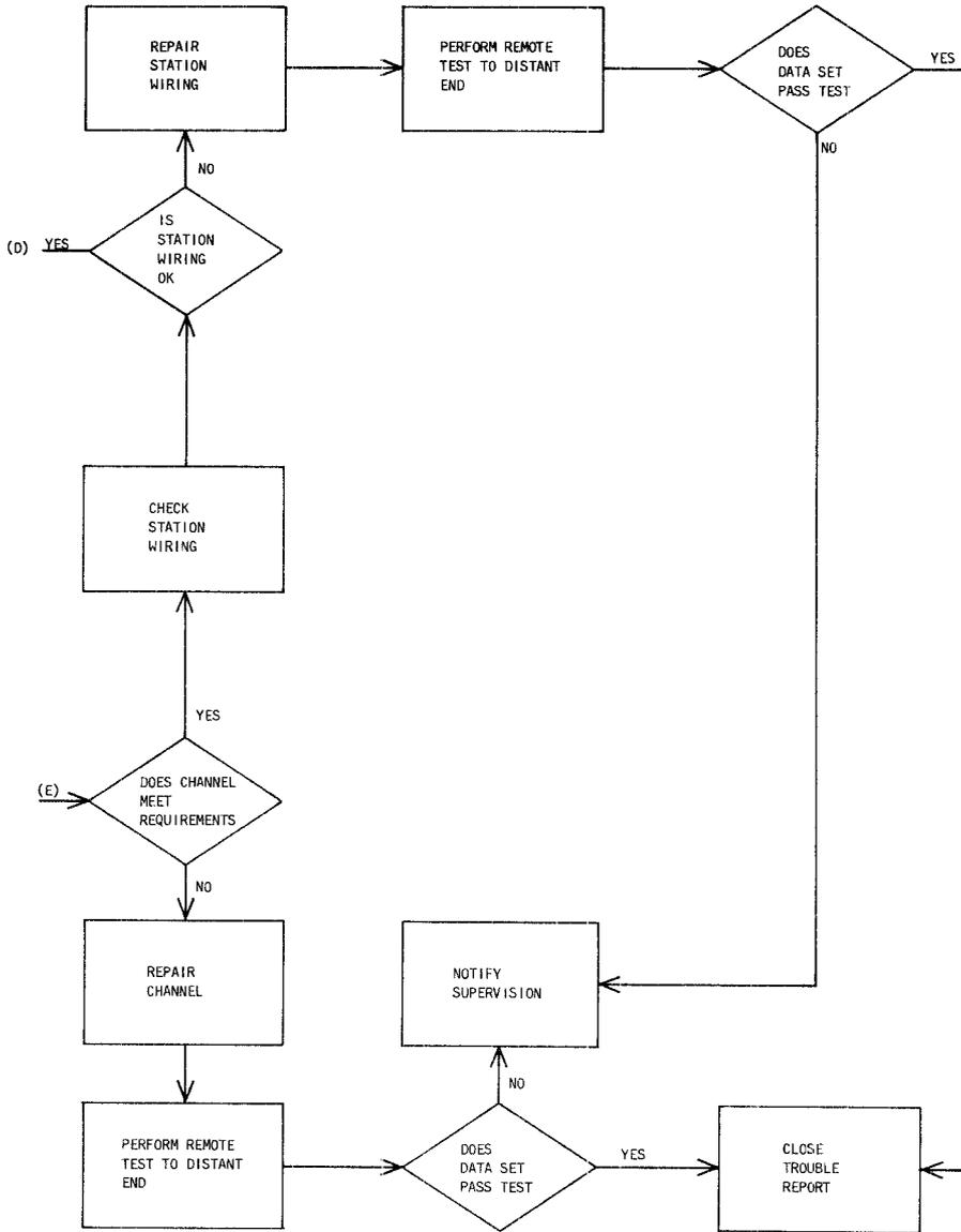
Fig. 6—4-Wire Maintenance Test Sequence (Sheet 3 of 3)
