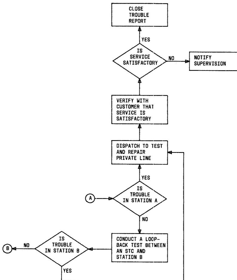
Fig. 4—4-Wire Maintenance Flowchart (Sheet 2 of 2)
