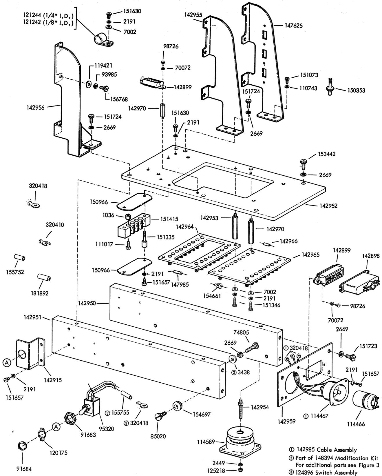
FIGURE 1. HIGH SPEED TAPE PUNCH BASE
