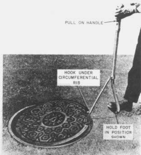
Fig. 30—Unseating Cover With PTS-49 Manhole Cover Lifter
