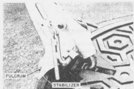
Fig. 18—Manhole Cover Lifter in Position to Lift Cover
