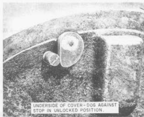
Fig. 4—Locking Assembly in Unlocked Position
