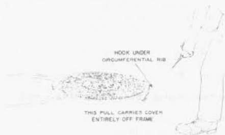
Fig. 11—Sliding Cover Clear of Frame
