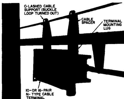
Fig. 14—10- or 16-Pair N-Type Cable Terminal Installed
