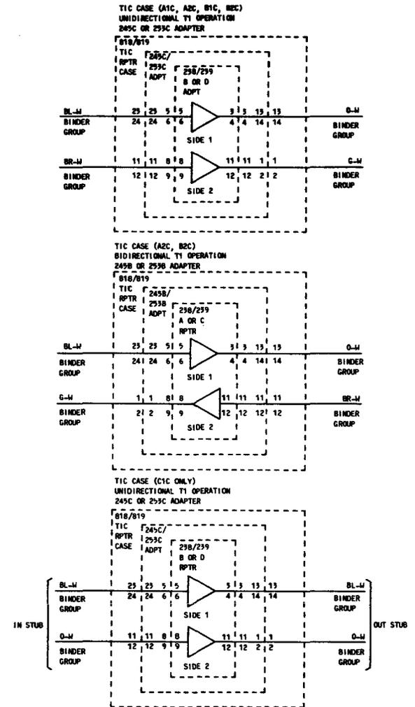
**Fig. 14—Equipping Housing With Adapters**
