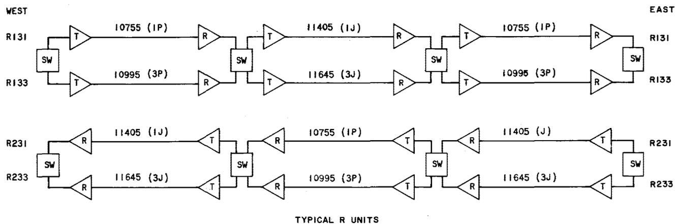
Fig. 2—Typical R Units for 11-GHz Radio Systems
