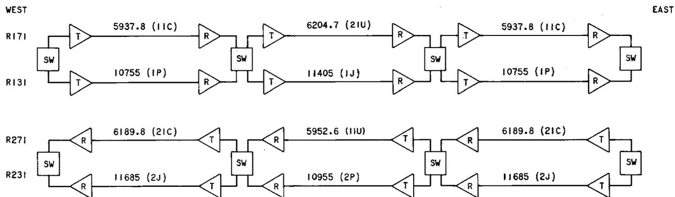
Fig. 4—Typical R Units for 6-GHz Radio Systems (Normal Plan for TM)
