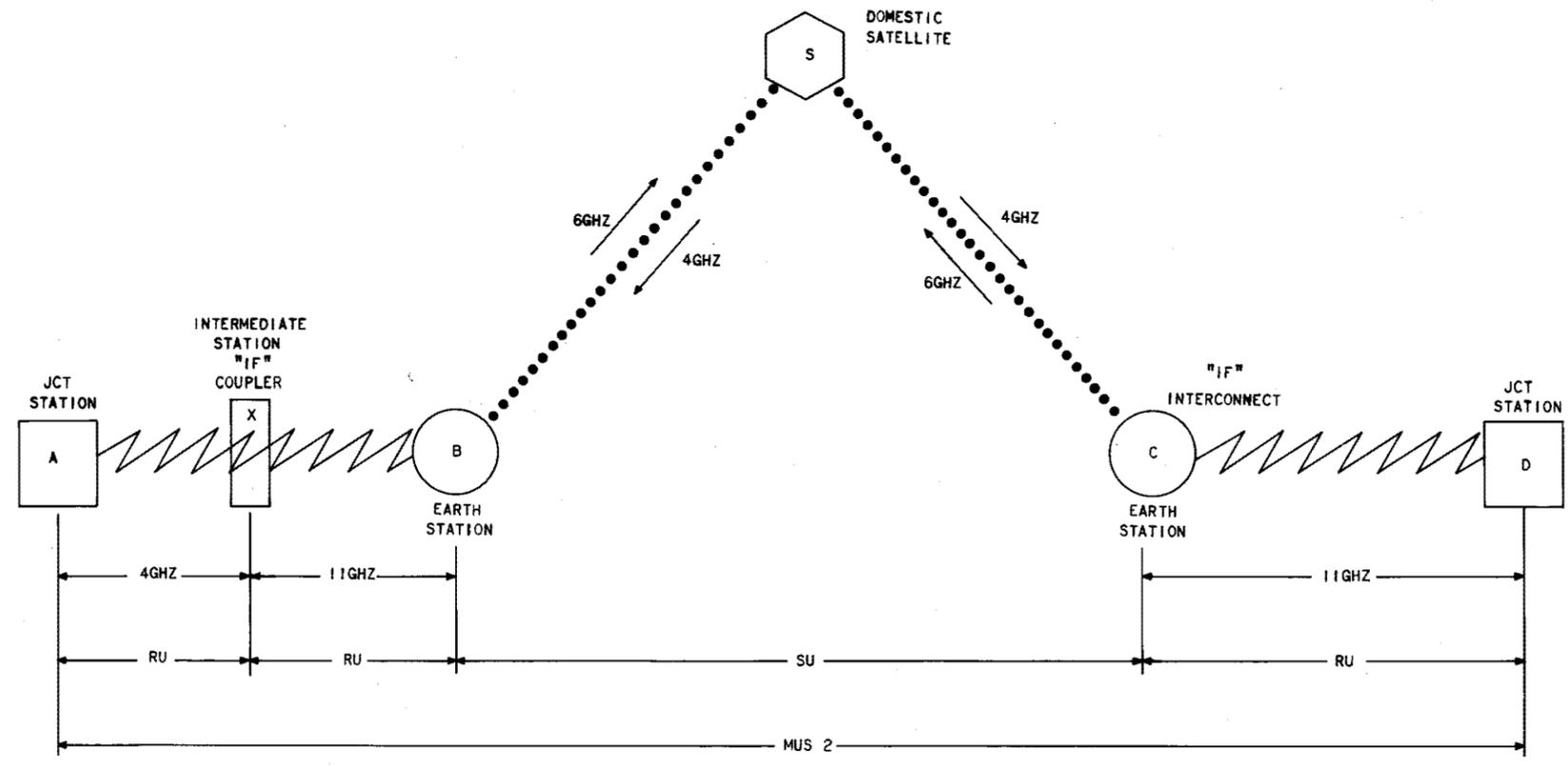
Fig. 6—Typical Domestic Satellite System
