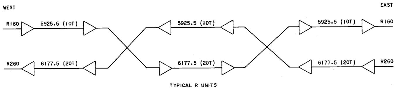
Fig. 3—Typical R Units for 6-GHz Radio Systems (Regular Plan for TH and TM)
