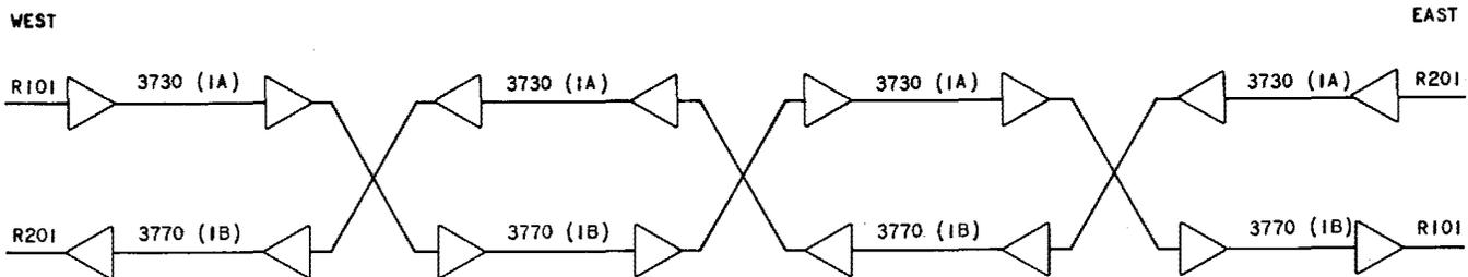
**Fig. 1—Typical R Units for 4-GHz Radio Systems**
