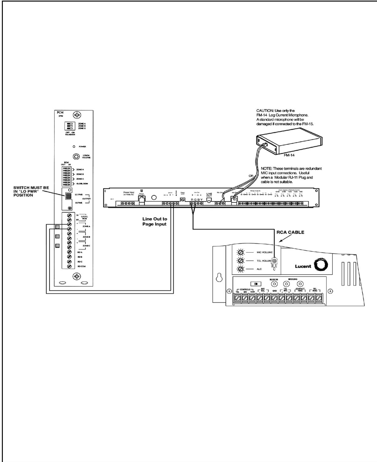
Figure 3-4. FM-15 ALC Used With A Lucent Paging Control System (LUPCMALL)
