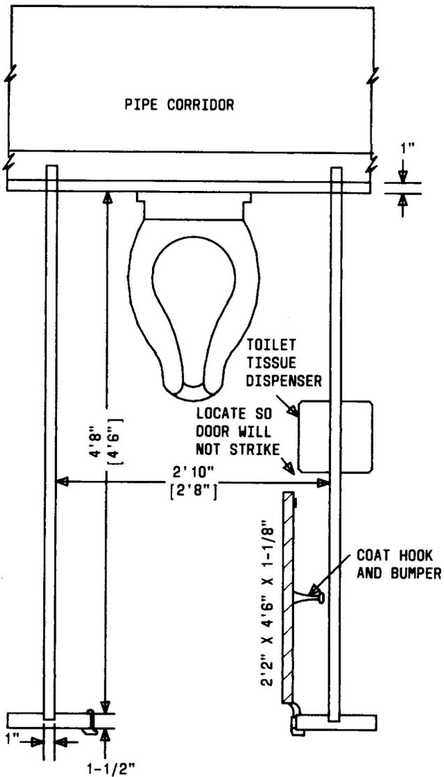
Fig. 3—Conventional Wall-Type Water Closet
