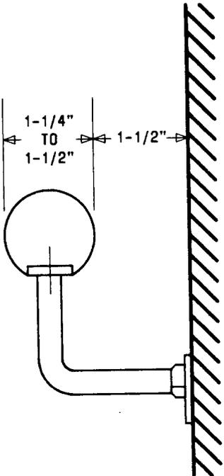
Fig. 9—Size and Spacing of Handrails and Grab Bars for Physically Handicapped Persons
