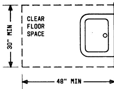
Fig. 11—Clear Floor Space at Lavatories for Physically Handicapped Persons
