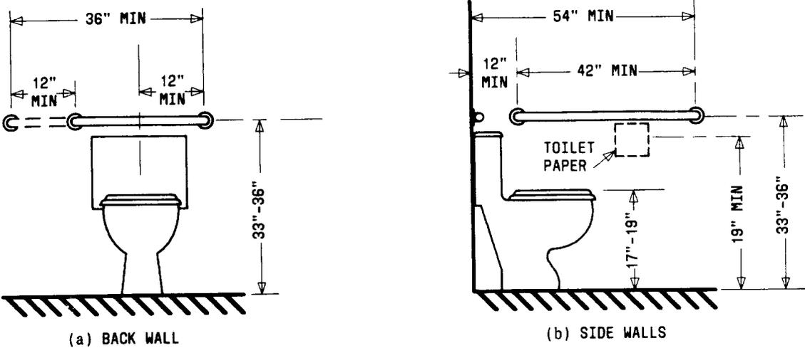
Fig. 8—Grab Bars in Water Closets for Physically Handicapped Persons
