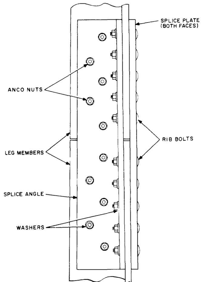
Fig. 8—Butt Leg Splice
