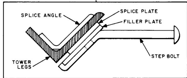
Fig. 12—Typical Step Bolt at Leg Splice
