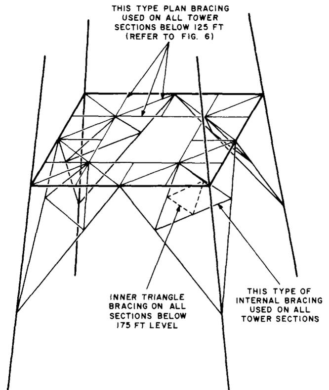
Fig. 7—Tower Bracing
