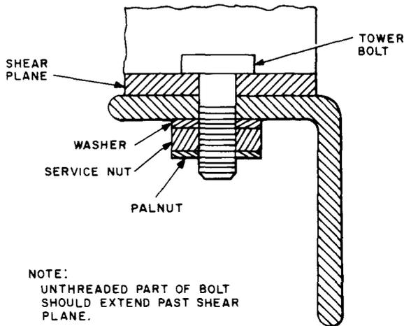
Fig. 5—Tower Bolt in Place
