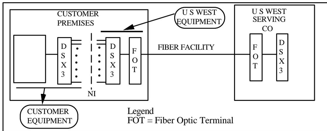
**Figure 2-2:** Electrical Interface CT Capacity
