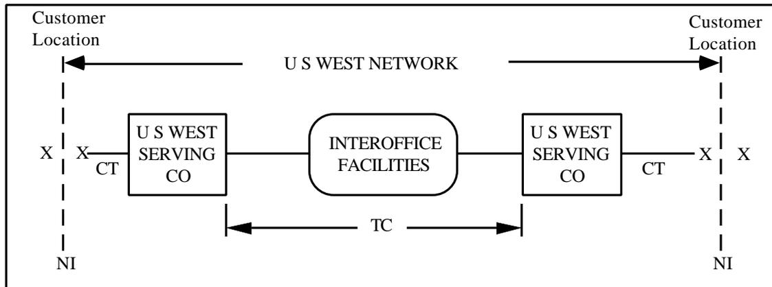
**Figure 2-6:** Customer Premises-to-Customer Premises Channel
