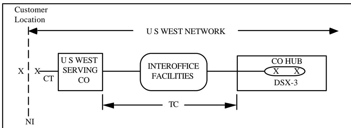
**Figure 2-7:** Customer Premises-to-CO Hub Channel
