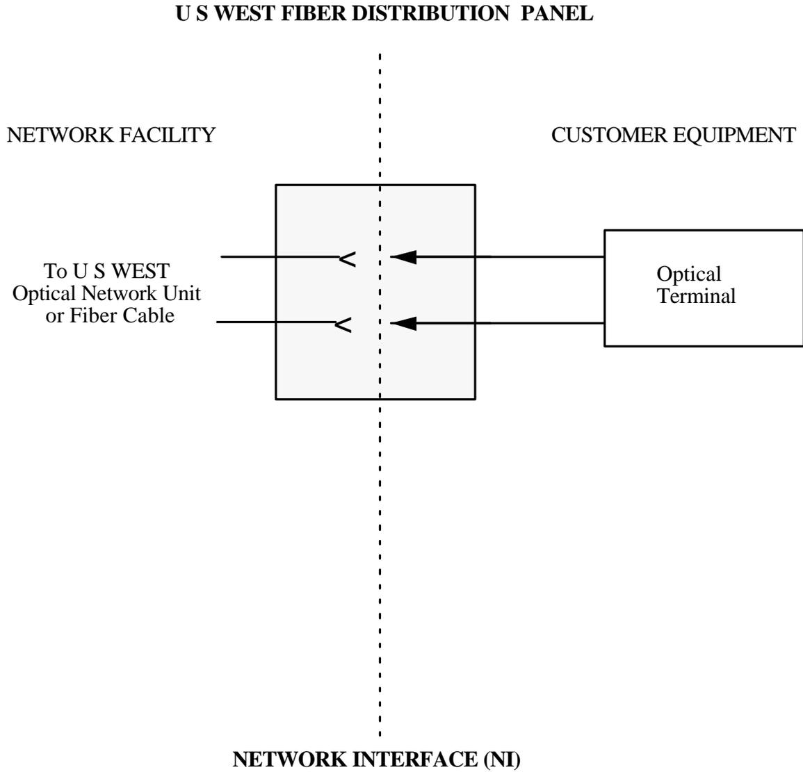
**Figure 3-3:** Optical Interface for Carriers and EUS
