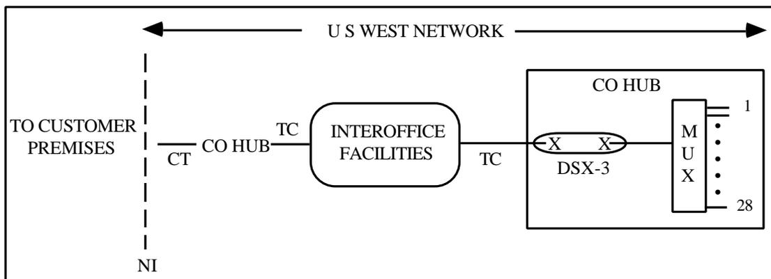
Figure 2-9: Hub Multiplexing Feature
