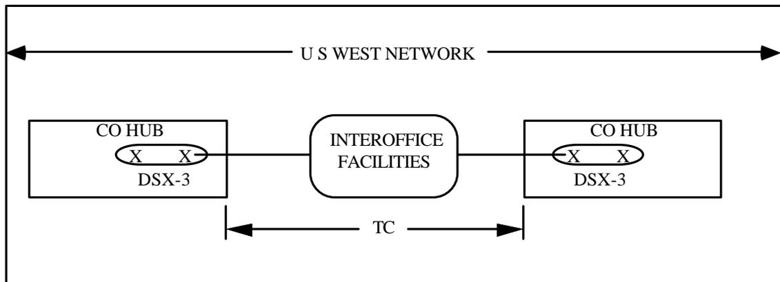
Figure 2-8: CO Hub-to-CO Hub Channel
