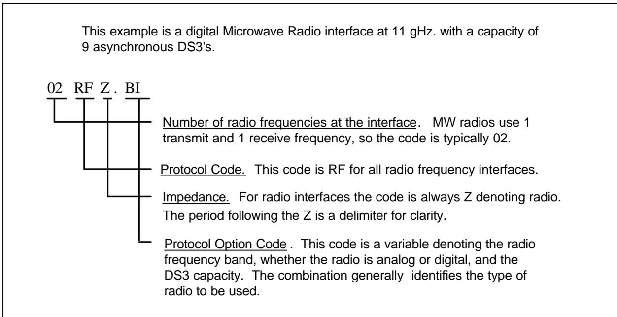
**Figure 4-3:** Radio NCI Code Example
