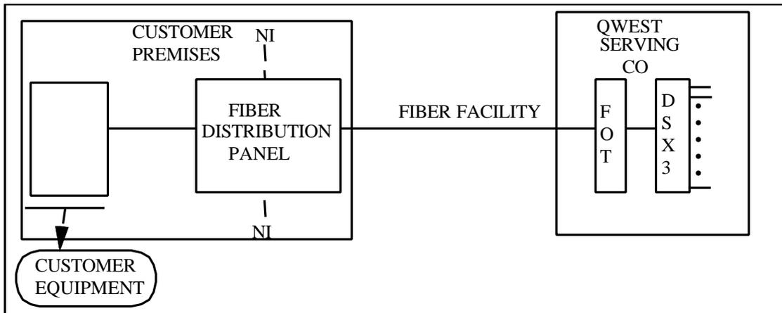
**Figure 2-3:** Optical Interface Capacity CT
