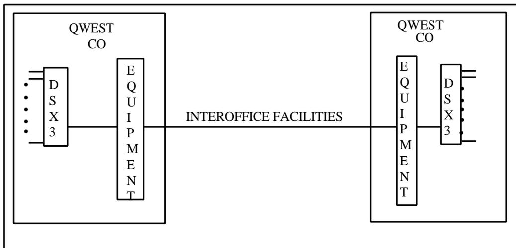
**Figure 2-5:** Transport Channel Element
