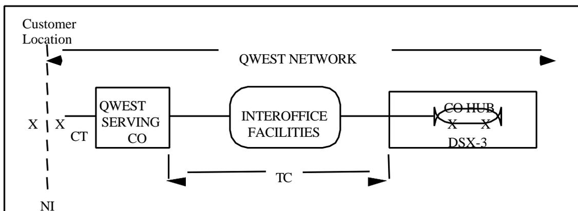
**Figure 2-7:** Customer Premises-to-CO Hub Channel
