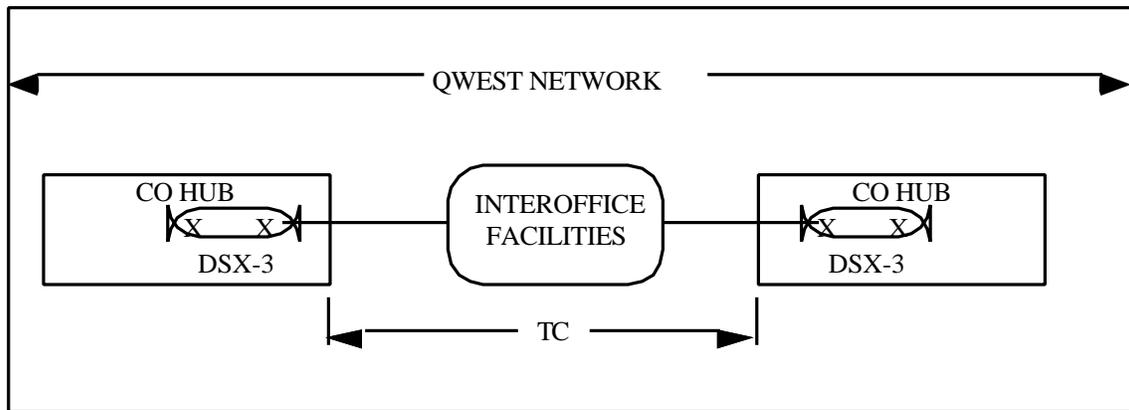
Figure 2-8: CO Hub-to-CO Hub Channel
