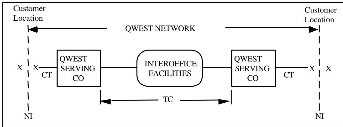
**Figure 2-6:** Customer Premises-to-Customer Premises Channel
