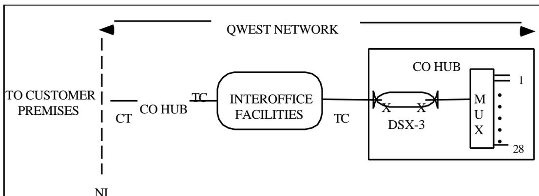
Figure 2-9: Hub Multiplexing Feature
