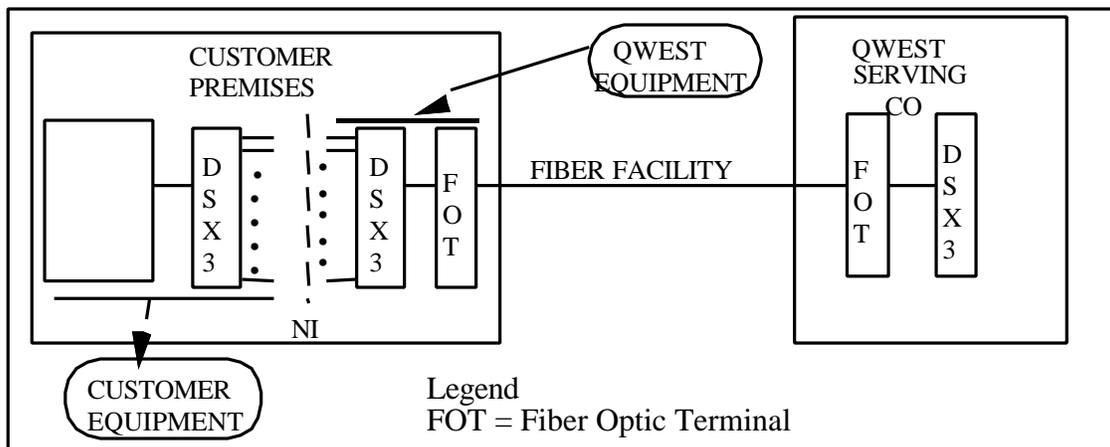
**Figure 2-2:** Electrical Interface CT Capacity
