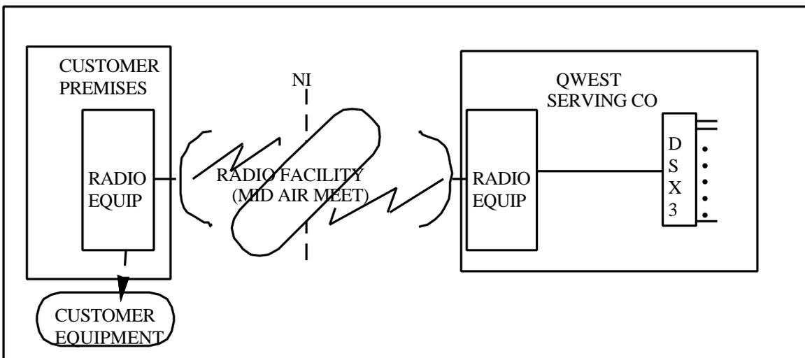
**Figure 2-4:** Radio Interface Capacity CT
