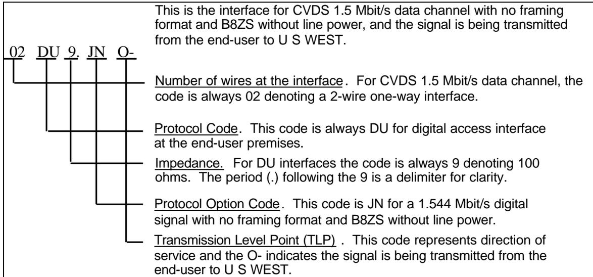
**Figure 3-1** CVDS 1.5 Mbit/s No Framing B8ZS Without Line Power NCI Code
