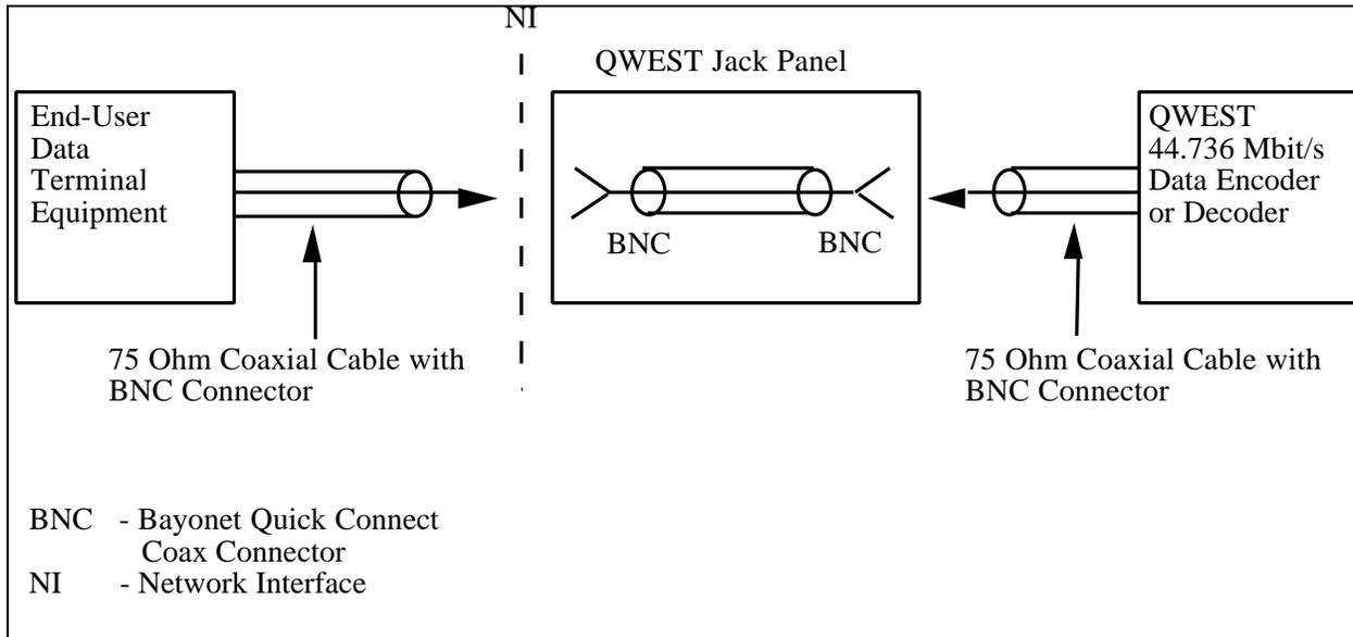
**Figure 4-2** CVDS 45 Mbit/s Network Interface Connection
