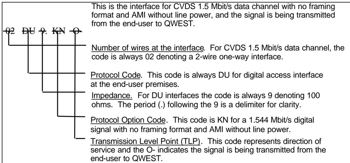
**Figure 3-2** CVDS 1.5 Mbit/s No Framing AMI Without Line Power NCI Code
