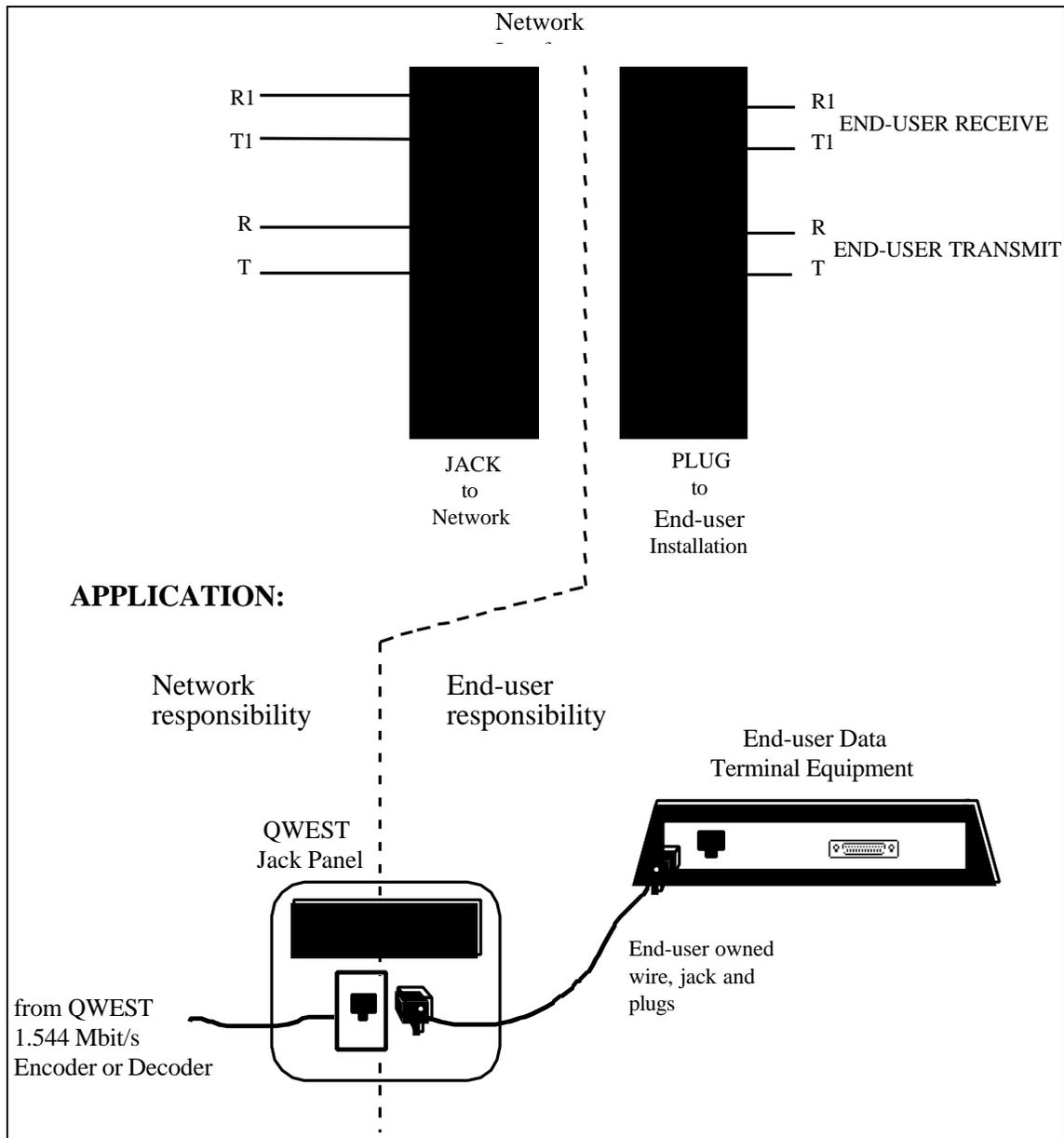
Figure 4-1 CVDS 1.5 Mbit/s Network Interface Connection
