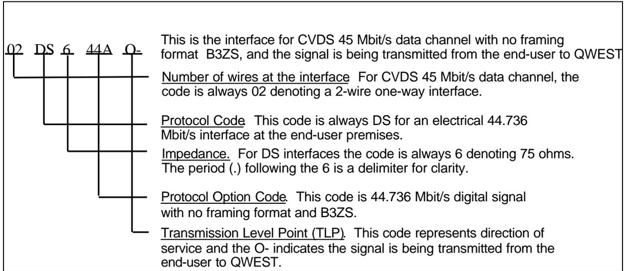
**Figure 3-3** CVDS 45 Mbit/s No Framing B3ZS NCI Code
