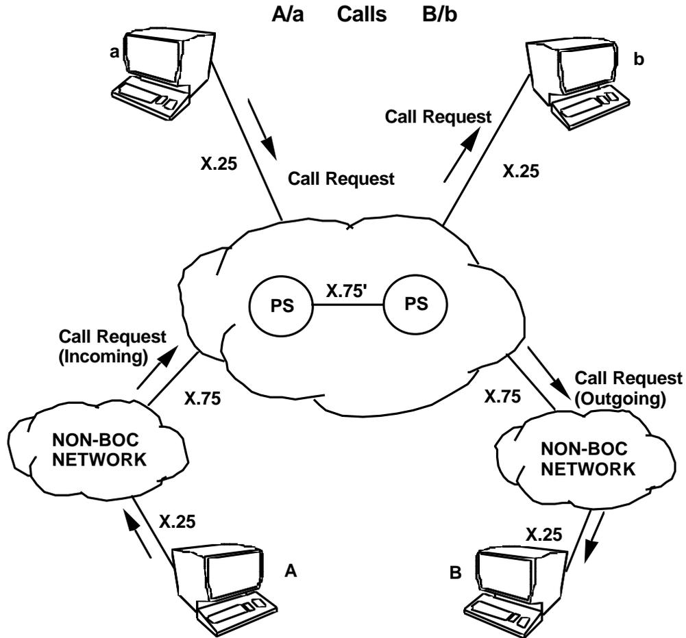
Figure 2-17 'Incoming' and 'outgoing' X.75 Interfaces Relative to a BOC Network
