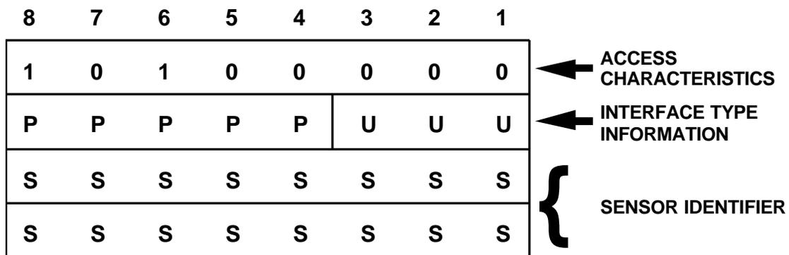
**Figure 2-16** Access Characteristics
