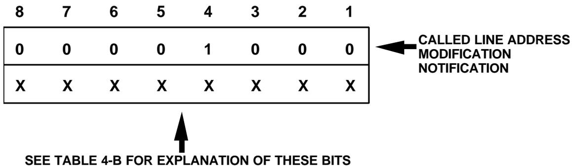
**Figure 2-9** Called Line Address Modification Notification
