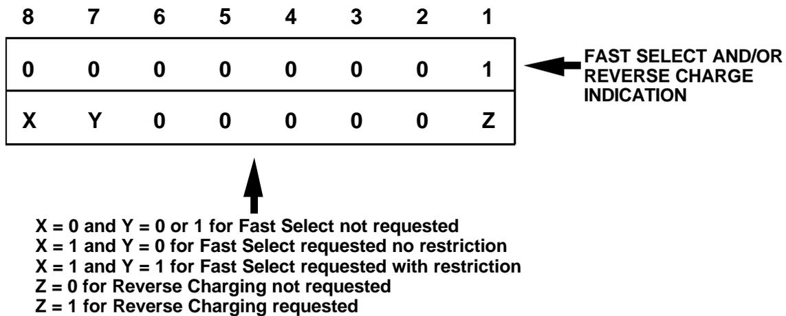
**Figure 2-6** Fast Select And/Or Reverse Charge Identification
