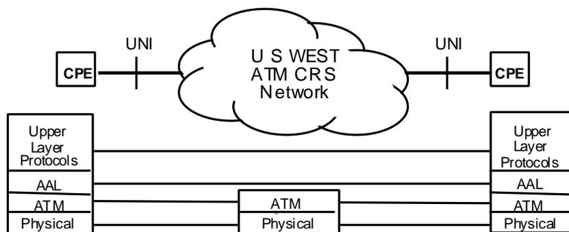
**Figure 2-1** U S WEST ATM Cell Relay Service Protocol Relationships
