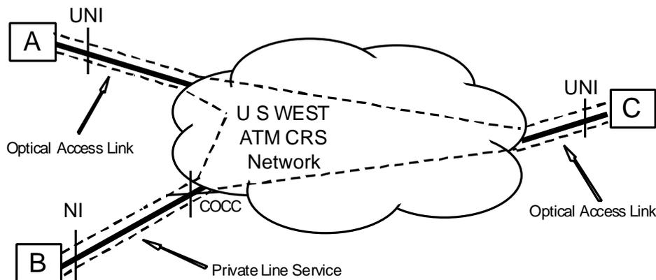
**Figure 2-2** Example of EU Networking Using U S WEST ATM Cell Relay Service
