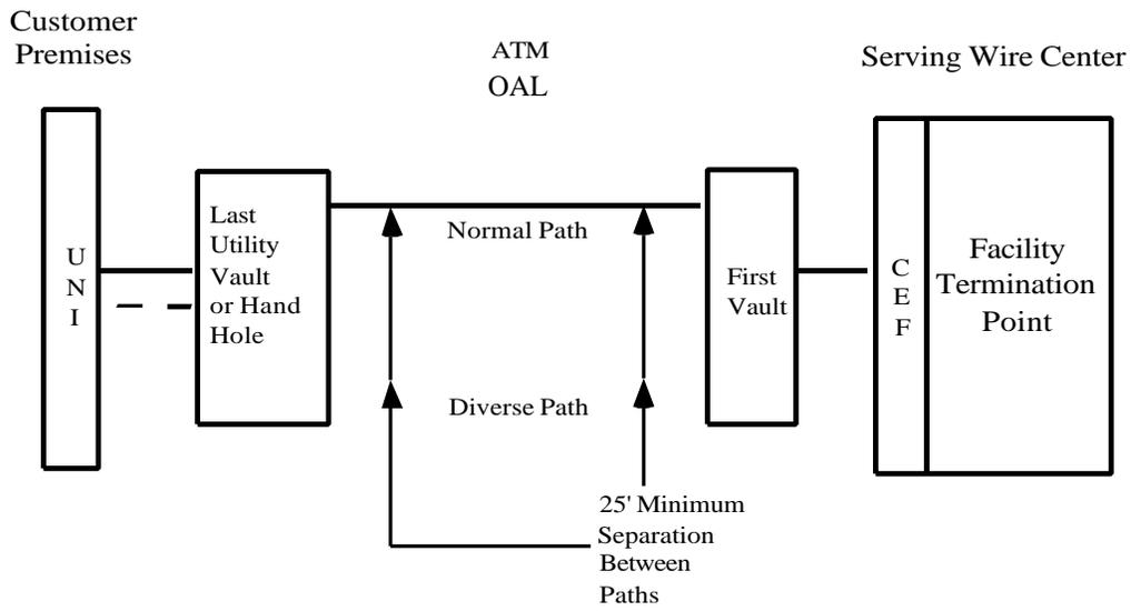
NOTE: There is no minimum separation from the vault/ terminal into the wire center/ customer premises
