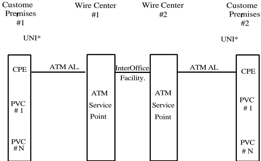
N = 1 thru 50 VPCs, 1 thru 220 VCCs for a 1.544 Mbps access line speed
